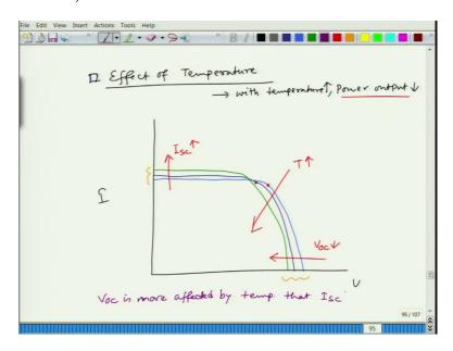
And another not-so-intuitive effect of temperature ok. Usually, at a lower temperature, the photovoltaic efficiency or photovoltaic generation is much more than for the higher temperature ok. So, with temperature, power output decreases ok with temperature increase, power output decreases.
