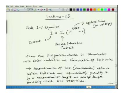
So today we are going to talk about the real interesting thing which is when light falls on the photovoltaic material or the P-N junction diode, what happens, ok. What magic happens that it gives you electric current, ok. So, up to the last class, we have looked at the dark I-V equation, which is given by,
