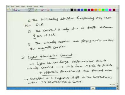
So, let me just summarize these observations. So, the interesting stuff is happening only near the space charge region and the current is only due to drift because  $\xi \neq 0$  here or at SCR. But the effect is failed nearby region as well because the added electrons or holes they can come drift near the space charge region edge. Just by thermal agitation or thermal movement and they can be sucked into the other side.
