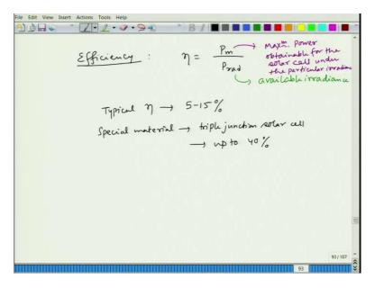
So, that is one quantity that talks about the performance metric you can say of the photovoltaic material or panel, and often you will hear this term efficiency; efficiency is very simple; it is what power you are getting. And by tracking the maximum power point and power that is put in the material, that means solar power that is coming on the panel ok.
