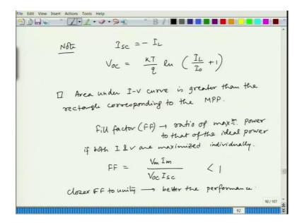
So, some quick notes; note that this  $I_{SC}$  is nothing but  $-I_L$ . If you look back a couple of yeah here, yeah,  $I_L$  is the current value when V equal to 0. Now we have inverted it in the positive direction. So,  $I_{SC}$ , the short circuit current is nothing but the minus of light generated current ok and  $V_{OC}$  is
