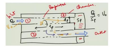
So, we can sort of draw the configurations. Suppose we have this kind of a thing, if the flow comes in here and it can be a circular section and you have a perforated section. So, you have this. So, you have this kind of a thing. So, and it goes like this. The flow has to necessarily come out here and again grace and become like a grazing flow in the duct 2.
