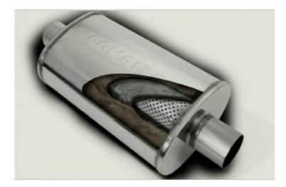
You know you see, this is the part and this connects of course, this is a you know let us say this inlet this is the outlet where my mouse is pointing, the flow comes in here and its smoothly guided by the perforated pipe and leaves outside, it does not allowed to expand. I mean not allow to freely expand the acoustic wave, nevertheless allowed to interact with the cavity and the cavity is not empty now.
