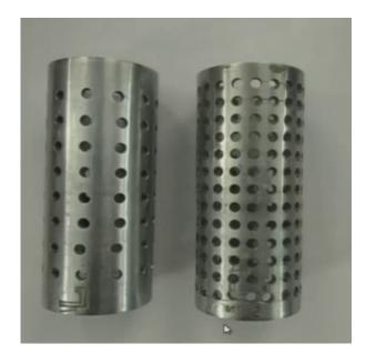
So, we see these perforated tube, so these are something that we fabricated sometime back, this is nothing but something like 2 and a half a 3 mm MS Steel pipes and a number of holes are drilled at regular intervals as you can see here about 2 mm, 3 mm holes and the regular regulated. This is definitely highly porous because you know porosity is about 28 to 30 percent somewhere between that and this is about only 12 percent.
