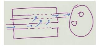
But there are other elements which something like let me just sort of draw it quickly for you guys. So, here we can have a solid pipe and we have a overlapping element and ok, so the flow has to go through this, flow has to go through this ok. So, basically such an element is called a cross flow expansion chamber.
