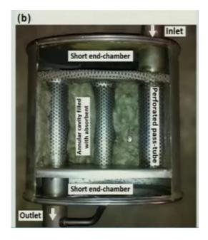
And then, this is yet another more complicate mufflers hopefully we will be doing some plane wave analysis of this thing next week. So basically, you know the flow comes in here as it is shown somewhere here inlet and this is an outlet, but in the process it has to negotiate number of turns like the flow is reversed here is end chamber.
