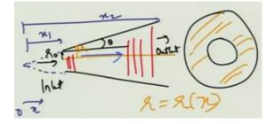
So, you see here this is a schematic of a conical duct and the wave propagation. Let us say this is the inlet and this is the outlet. So, what we are going to do is basically use our Webster's horn equation to study acoustic wave propagation in such a system.
