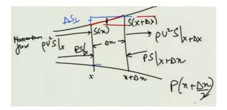
So, it will turn out that momentum equation for a duct of gradually varying area section is the same as the momentum equation for a duct with a uniform cross section.
