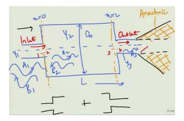
So, this was the simple expansion chamber muffler. And we saw that I mean after a little bit lengthy derivation, we saw that the transmission loss of such a system then is given by the following expression which is of course we studied that in detail.
