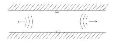
Your duct system is here, and the membrane is ruptured now, which completely you put a pin or something and it produces a noise tuck something like that. And so, it produces a wave, actually two waves are a pair of waves; one that propagates like I said in this direction, and the other one in the negative *x*-direction, ok. So, the membrane is gone, this disturbance which propagates.
