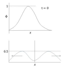
So, this is self-consistent, but as the time propagates. So, right now we have x, we have  $\phi$ , we have the general Gaussian pulse say at t = 0. And so, the wave splits apart. So, it comes down becomes smaller at certain time and then as the time evolves, it starts splitting into two parts; one this pulse propagates in the positive direction, this pulse propagates in negative direction.
