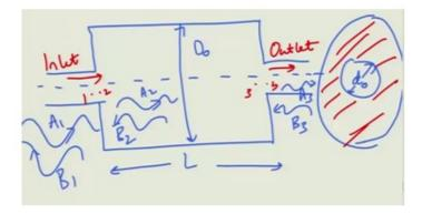
So, basically as you can now guess that a simple expansion chamber something like this you have your thing like this and you have and here you have a thing like this. So, the section can be elliptical this section it can be elliptical or a circular thing pressures are of circular cross section. They can also be elliptical, but circular other ones that are more preferred because they have less break out noise have more rigidity like I was mentioning.
