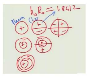
So, this transfer matrix is there. So, what is the limit if you recall the lectures from week 2 what for a duct of radius  $R_0$  or diameter  $D_0$  the cut on frequency for the 1 0 mode 1 0. You know if you recall our discussion this was the plane wave mode, this was the first
