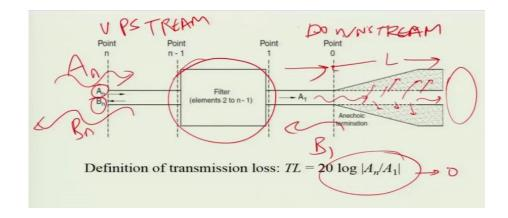
So, but the trick here is that to make it of sufficiently large length. So, that by the time the acoustic power reaches here most of it is dissipated and there is nothing left to be reflected. It is sufficiently dampened or the amplitude has died down a lot.
