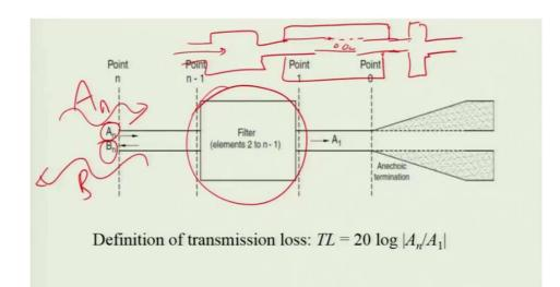
So, what do we see here? Well, we see a wave, that is coming well towards the muffler directed towards the muffler or coat and coat incident on the muffler, which is  $A_n$  and the wave front that propagates in the opposite direction.
