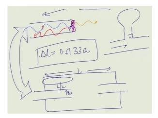
So, when a wave is coming here, some part is being reflected back, but other part is also going. This is much more complicated, because the point I am going to make is that this thing does not exist infinite flange businessis no longer there. This has this really simplified the matter, but the fact that it is notthere poses considerable difficulty in the mathematical analysis.
