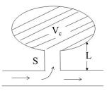
So, net impedance like what we discussed in the last class.Let me go to the slide the last class, we saw this was the system j  $\omega L/S$  and  $+\gamma p_0/j\omega VC$ . So, when we simplify the matter simplify this thing and find out the frequency at which the impedance goes to 0; this is also imaginarythis part is imaginary this part is imaginary.
