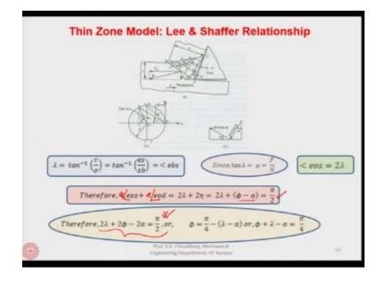
Assuming uniform stress  $\tau$  and normal stress  $\sigma$  on the rake face the friction angle we can find out here. And this will be the  $\tan^{-1}\frac{\tau}{\sigma}$ . From this you can find out that this will be equal to  $\tan^{-1}\frac{es}{sb}$ . Since  $\tan \lambda = \mu$ , you can find out the  $\mu$  which is  $\frac{F}{N}$ .
