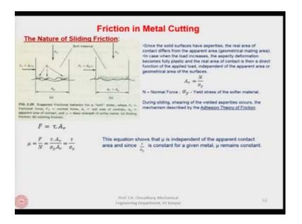
After that we will be discussing the topic which is friction in metal cutting. Why we are discussing this, because in the normal case when we have the sliding friction there we have the F and the N, because of the normal force the friction force F is created. So, the  $\frac{F}{N}$  we always assumed to be constant; that means, the F is proportional to N, this is what happens in the case of the sliding friction.
