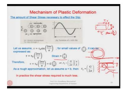
Then we started discussing the amount of shear stress necessary to affect the slip. Here we said that if we had the equilibrium position or equilibrium lattice structure and when a stress is applied with sufficient shear force, in that case the atoms will be moving from the stable position to the next position because of the high strain rate of deformation and the distance moved by the atom is x and the distance of between two layers of atoms is b and the atomic distance is a.
