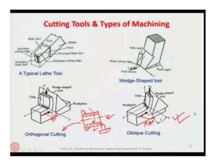
Now we will discuss about the cutting tools and the types of machining. This is a typical lathe tool, as shown in the slide. Here we have the shank, this is called the shank which is the portion by which the tool is clamped in the tool post and then we have the rake face, we have the principal flank face, this is the principal flank face.
