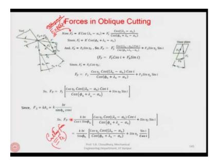
Let us look at this slide. Here we have determined analytically the cutting force,  $F_p$ . This is the cutting force along the cutting velocity vector and this  $F_p$  is equivalent to the cutting force in the orthogonal cutting. We found out the following expression and this expression can be further simplified by taking  $\cos \eta_s = \frac{1}{\sqrt{1 + \tan^2 \eta_s}}$ . This is the formula
