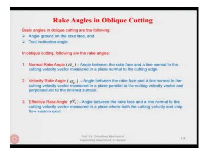
Now, let us see the rake angles. If the forces we have seen now how the rake angles can be determined in case of the oblique cutting. The basic angles in oblique cutting are the angle ground on the rake face and the tool inclination angle. Now, since the tool is inclined with respect to the cutting velocity vector, the chip does not flow exactly perpendicular or normal to the cutting edge. It will flow to that side of the normal to the cutting edge where it will get less resistance to the flow.
