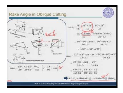
So, if you extend this line, it meets the D point. Now, this line is intersecting with this vertical line EF at a point which is EE prime. So, this is E this is E prime and this is D and this angle is i. So, from here we are finding out that this is DE sin i which is equal to EE prime; this is what we got in here.
