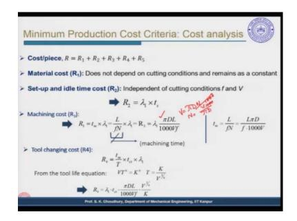
With these designations now, we have the cost per piece R, this will be equal to the raw material cost plus settling plus idle time cost per piece plus machining time cost per piece plus the we have  $R_4$ , we said that this is the tool changing cost per piece and the tool cost per piece. So, all these costs are to be considered for calculating the tool cost per piece overall.
