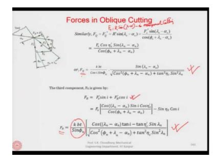
For example,  $\eta$  is introduced, because this is due to the tool inclination in the oblique cutting. Similarly, we can find out the  $F_Q$  which is the  $F_Q' = R' \sin(\lambda_n - \alpha_n)$ . So, if you remember that in the orthogonal case  $F_T$  was equal to  $R \sin(\lambda - \alpha)$ .
