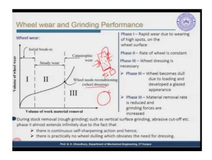
Now, let us see how the grinding wheel wears out. If you plot the volume of wheel wear along the y-axis and the volume of work material removal along the x-axis; you will find a curve of the wheel wear which will be more or less similar to the one that we have seen in case of the single point cutting tool.
