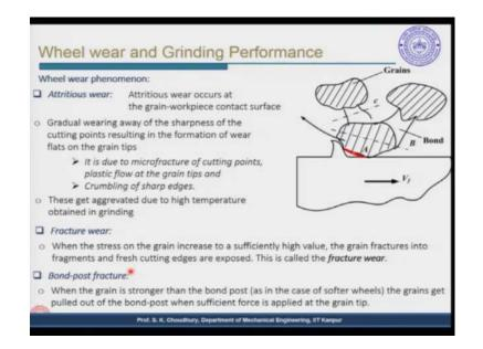
Now the wheel wear phenomena: when the wheel gets in contact with the work piece initially because of the wear due to the rubbing and ploughing, there is a flat created here, this is shown as A. This is the gradual wearing away of the sharpness of the cutting points, resulting in the formation of wear flats on the grain tips. So, this is due to the micro fracture of cutting points, it could be due to plastic flow at the grain tips and due to crumbling of the sharp edges.
