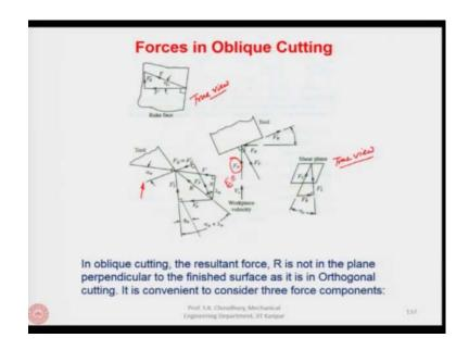
These are the forces in oblique cutting in the diagram shown. What is shown is that, this is the tool in the base plane and the tool is inclined. Inclined means this tool edge is making an angle of i with respect to the line perpendicular to the cutting velocity vector.
