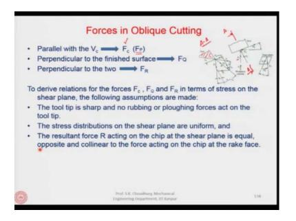
These forces are parallel with the cutting velocity which we will call as the  $F_c$ . Here by the way this is given as the  $F_p$  probably; if you can see that this is the  $F_p$ , this is equivalent to what we have said earlier as the  $F_c$  or the cutting force.
