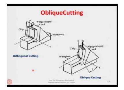
Next topic that we will be discussing after the grinding process is the oblique cutting. I would like to show you the diagrams which we have already seen earlier and compare the orthogonal cutting with the oblique cutting. We said that in case of orthogonal cutting, the tool edge is perfectly perpendicular to the direction of the cutting velocity vector.
