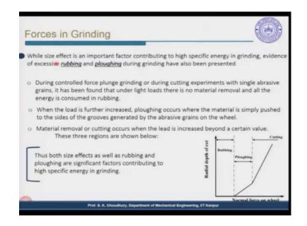
While size effect is an important factor contributing to high specific energy in grinding, there is excessive rubbing and ploughing during the grinding, they are also responsible along with the size effect for very high specific energy.
