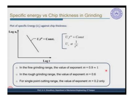
Now, let us see how in the grinding process this can be plotted; for example, if we plot the same curve in the log-log scale. Let us say here it is the log of the uncut thickness and here it is the log of the specific energy, then the curve will be a straight line like this. And, this straight line can be represented by the equation as the  $U_c t^m = Const$  or
