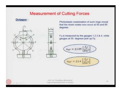
As you can see from the above slide that the left figure is an octagon which has the principle of the ring type dynamometer, but it is more rigid. And, another view of the ring type dynamometer is also shown from the side. Photoelastic examination of such rings reveals that the strain nodes occur at  $50^{\circ}$  and  $90^{\circ}$ . If you remember, in the ring type
