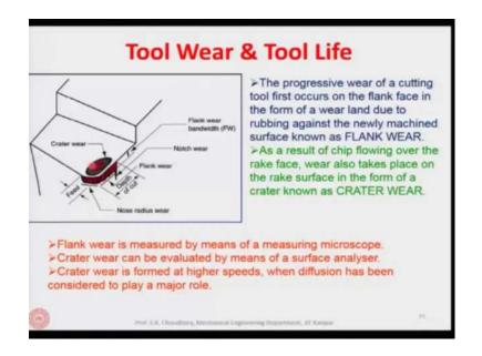
Now, how the tool wears out? As I said that chips are moving continuously over the rake face of the tool so that there is a wear at the rake face. The flank face is in continuous touch with the already machined surface, so there is also a wear.
