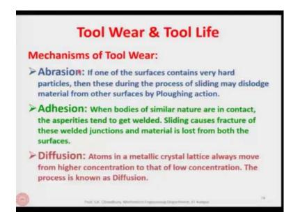
Now, the mechanism of tool wear can be either abrasion or adhesion or diffusion. It can be either one of them or a couple of them together. By mechanism we mean to say the factors which are responsible for the tool wear. What is abrasion? If one of the surfaces contains very hard particles, then during the process of sliding these may dislodge material from other surfaces by ploughing action.
