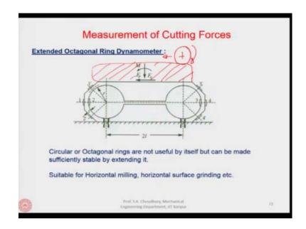
Next is the extended octagonal ring dynamometer; the octagonal structure that I have shown is an improvement of the ring type structure, which is still not enough to withstand the rigidity that is required for milling or grinding for example. So, these extended octagonal ring dynamometers are used for grinding or milling.
