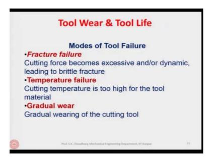
Next topic will be tool wear and tool life. Let me give you a preamble that this is a very important topic because the tool material is very expensive. The tool material is harder than the work piece material. Tool materials should have less wear.
