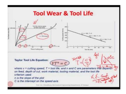
The curves for the tool flank wear are drawn against the time of cutting. The curves are drawn for different cutting speeds. Usually at higher cutting speed, the flank wear will be more. At lower speed the flank wear is less or the less steep curve, but at a higher speed the flank wear is more, this is very obvious.
