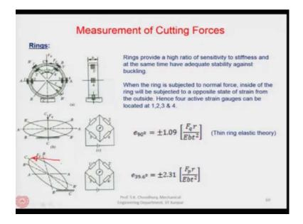
Now, let us see how it is done in case of a ring type dynamometer or ring type element. Rings provide a high ratio of sensitivity to stiffness and at the same time have adequate stability against buckling. These are the elements which are also used to measure forces. Now for example, if we have a ring like structure and the side view is here. So, it has been seen that these are the nodes when they are subjected to the forces like  $F_q$  and  $F_p$ as shown here.
