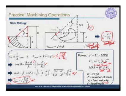
Now, in case of practical machining operations of slab milling, it is little different than the other processes because here in case of drill we had two teeth. In case of single point cutting tool we had one tooth and in case of milling it is more than 2, it is multiple. So, the basic difference is that here the feed which is given is feed per tooth.
