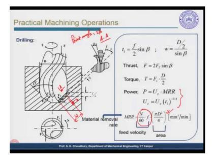
If you see this diagram here - the torque is given here and this is the force which is the thrust, both are given to the tool which is the drill here. Now, if you take a cross section A-A, we said that it will be visible like this. So, here we have the tool with the rake face and this defines the inclination of the rake face of the tool.
