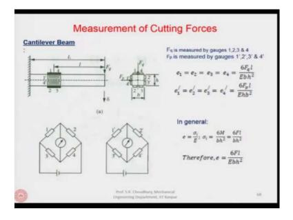
For example, for a cantilever beam, normally the load that has to be measured is sensed through the moment; because if the point of application of the load is known then the load into this distance will be moment. So, if you can measure the moment, from there knowing the distance from the application of the load we can find out what is the force. This is the principle by which the forces are measured in the cantilever beam.
