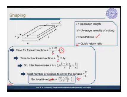
Now, let us see how much time it takes for shaping a particular length and the width of a part. Let us say we have a block alright and this block has to be either shaped or it can be produced by planing.
