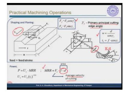
Now, let us see what happens in case of shaping and planing. Now, in shaping and planing the tool used is almost the similar to the tool that is used in the case of the turning. So, here is the diagram showing shaping or planing, only difference is that in shaping the tool moves, tool reciprocates and in case of planning, the workpiece reciprocates, otherwise there is no difference as it is.
