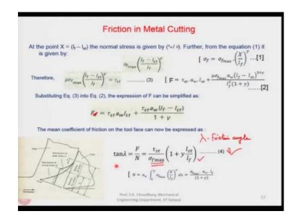
And what we said is that here is the distribution of the normal shear stress along the chip tool contact length which is  $l_f$  and this is how the distribution of the shear stress looks like.
