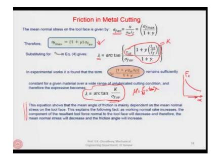
Next, we said that the mean normal stress on the tool face is given this way. We found out the mean normal stress and from there we can find out the  $\sigma_{f_{\text{max}}}$  which is  $(1+y)\sigma_{f_{av}}$ . So, finally we get that the friction angle is this and it was said that this factor remains sufficiently constant in practice (see the slide above) and therefore, this can be assumed to be equal to  $\arctan \frac{K}{\sigma_{f_{av}}}$ .
