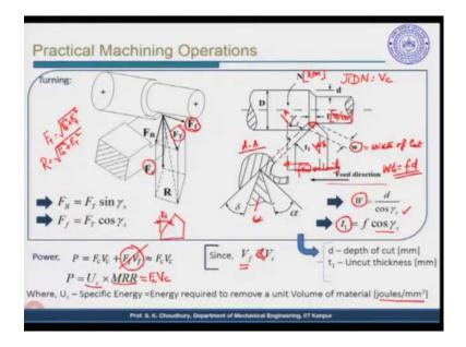
Well, let us see the turning operation. The workpiece is shown here in the schematic diagram; it is a pictorial view and earlier also we have discussed that this is the  $F_f$  which is the Friction force. Friction force is parallel to the workpiece axis and it is normally given in the direction of the feed.
