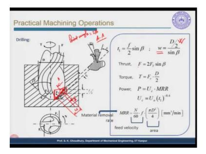
Now, in case of drilling, it is different because first of all in case of drilling the forces are different, that is, both the rotation and the feed is given to the tool, that is to the drill and here is a diagram of the drill shown. As you can see that suppose drill initially was at this point and with one movement of the drill, it has penetrated from this point to this point. So, the distance between these two point will be feed by 2; half of the feed because there
