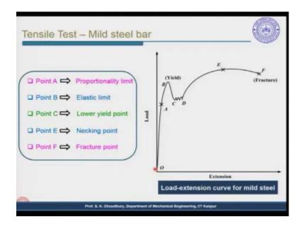
We have, let us say, a mild steel workpiece and it is being elongated and the force and the elongation or the extension and the load are being measured. So, if it is a mild steel workpiece, it is a ductile material. So, when we are applying the force, it is elongated up to a certain level, up to a certain point and as we know that up to this point the material remains in the elastic stage, meaning, that if we remove the load from this point, the material will come back to the initial position.
