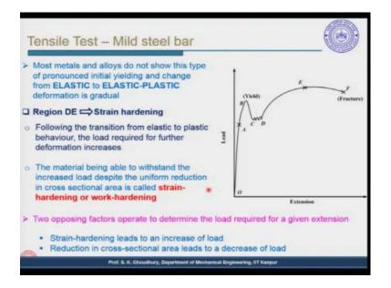
Most metals and alloys do not show this type of pronounced initial yielding and change from elastic to plastic, elastic plastic or plastic deformation is gradual. But, in case of mild steel this is the picture. Now, region D-E is the region of strain hardening; following the transition from elastic to plastic behavior, the load required for further deformation increases.
