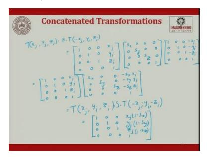
So, if we wanted to represent this in the matrices form, we can try to write it as  $T(x_i, y_i, z_i)$ . S.  $T(-x_i, y_i, z_i)$
