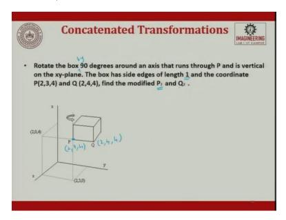
So now, let us take an example and try to solve the example. Rotate the box by 90 degrees above, around an axis that runs through P, point P and is vertical on the xy-plane. The box has side edges of length 1 and the coordinates P is nothing but (2, 3, 4) and Q is nothing but (2, 4, 4), find the modified P2 and Q2.
