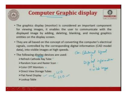
So now, let us get into Computer Graphic Display. Computer Graphic Display, the graphic display monitor is considered an important component of viewing image. Without the monitor whatever you develop, how are you going to it? So, the visualization of the complete CAD happens only because of the graphic display there. It enables the user to communicate with the display image by adding, deleting, blanking, moving graphics entity on the display screen.
