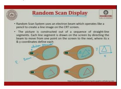
Now, let us look into random scan display. How does this random scan display work? Random scan display uses an electron beam, you see a beam which is coming out from a electron generator. So this is electron generator, this is the beam which is an electron beam. Random scan system uses an electron beam which operates like a pencil to create a line image on the CRT screen. The picture you see here it hits, then it draws and then it goes.
