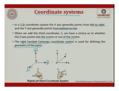
When we talk about coordinate system, there are 2 types of coordinate system. One, is called as the right hand coordinate system, the other one is called as a left hand coordinate system. So 2D, 3D is an extrapolation of 2D. So, what we do is, we will first try to understand 2D and then we can try to move towards 3D. In a 2D coordinate system, the X axis generally points from left to right and the Y axis generates point from bottom to top.
