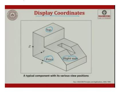
So, this is display coordinates which talks about top, front and side. So, this side, so right side view, front side view, top side. These are nothing but display coordinates.
