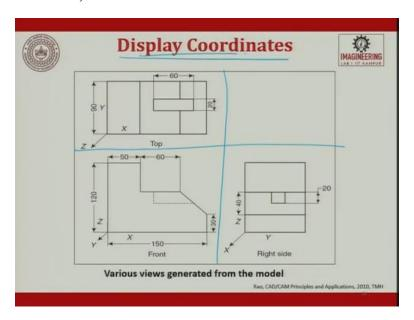
And this is, for that 3D object you can see here. Top, front and right side, all the three are generated. This is nothing but, a display coordinate system or display coordinates.
