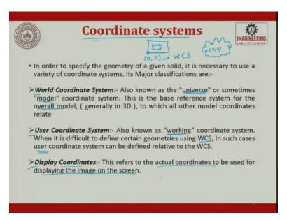
When we talk about coordinate system, there are 3 types of coordinate system generally followed in CAD. One, is called as the world coordinate system, the other one is called as user coordinate system and the third one is called as display coordinates. The world coordinate system is also known as universal or universe, or sometimes model coordinate system. It is the base reference system, for the overall model to which all other model coordinates are related.
