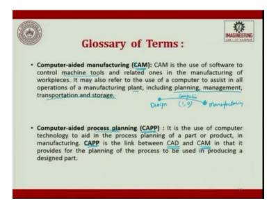
So, CAM is use of a software to control machine tool and relate once in the manufacturing of work pieces. For example, in CAM you can write you can draw a component and then generate a G code wherein which that can be used by the CNC. It may also refer to the use of a computer to assist in all operations of manufacturing plant including planning, management, transportation and storage. So, computer plays a very important role in CAM.
