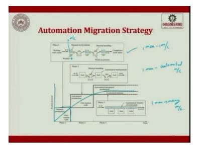
So, this is what is phase one wherein which you can see manual workstation; the jobs are here. So, there is a worker, so the worker does the job can push us the job to the next worker. He does some job push to the next worker, next worker, next worker, so here it is completely machine there and then worker. So, worker is trying to do the job, and the job is moved from station to station.
