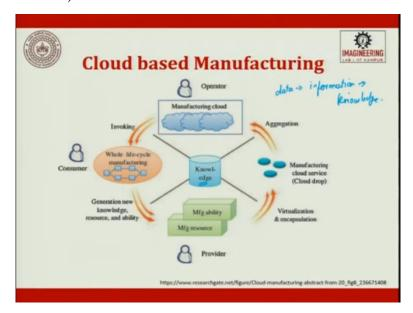
So, the cloud-based manufacturing that was for cloud computing, now let us move to our scenario of manufacturing so, you will have operator, you will have Manufacturing cloud server, then you will have provider, you will also have customer. So, operator he gets data from the customer, so customer is the consumer here, so the whole life cycle manufacturing is taken care, so then from here, how does he get the data he gets generation of knowledge, resource, and ability from this.
