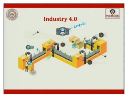
So, this is a video which shows industry 4.0. You can see here a bot linked plant, so here it says yes there is a cap which is laid and then the bottle goes inside the filling station happens here, it checks for the level if the level is of the specified limits then the bottle keeps going and then you start printing the label on top of it and then it checks for the level and finally it gets packed.
