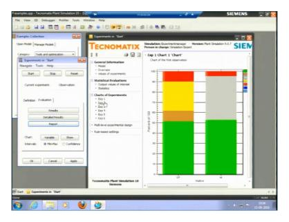
It was given here; the inputs that we gave output values sorry, output values are here, in these results. Experiment number one is a 100 parts with mean time to failure as mean time to repair as 5 minutes experiment number 2 is 100 parts with mean time to repair as 10 minutes.
