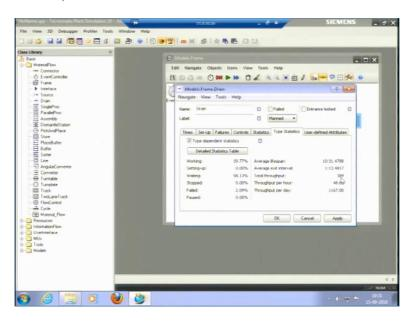
So, let me pick this constant time here and it was just to make you understand properly one minute I will apply. So, let me see if I run it for an 8-hour day and there to see the throughput open we try to see throughput it is throughput per day is 1167, per hour is 48 and the total throughput is 389 for an 8-hour day, for 8 hours.
