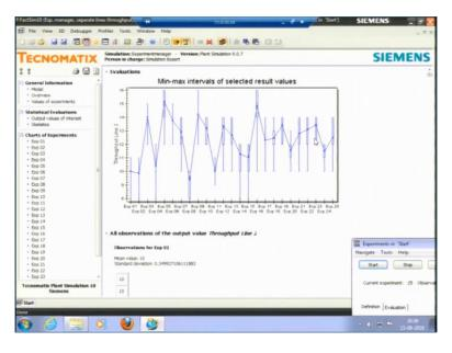
So, these are the output values of interest. So, if you see this, this is each experiment and 50 observations are given, this is for the throughput 2 you can see now, we have a box plot here so, what does this show? This, for instance, this is my experiment number 5, this line, in experiment number 5 there 50 observation and this is box plot this is my median and you can say there is a whisker and the third quartile is quite lower and we do not have the first quartile,
