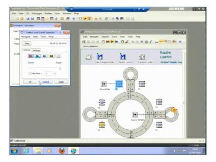
So, this is continuous material flow, I will select 2 lane track here so, traffic circle or segment table, traffic circle pick and open the model so, this is the model is already running so, I will just run the model you can see this is the trolley that can pick our material from so, this is source parts some processing is being done here, I can see what is the time of the processing here, the times is constant 1 minute.
