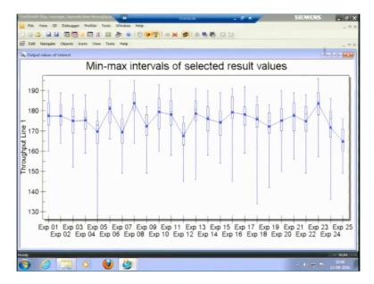
So, this I have obtained, the chart put for over the throughput of line 1. You can see throughput of a line, the variability is less, the two reasons for this: number 1 the processing times were in
