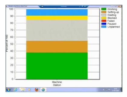
So, in this model we can see the chart, what is setting there is no end time I will put the end time here, 08:00:00, apply, okay. Let me try to run this model so, it has run for 1 day so, entity buffer is there, entity machine is there, this is similar to that. So, we can see the charts here, show chart. So, for only one machine it is showing the chart that, this is something unplanned blue colour is unplanned, then we have blocked we have, we do not have any failure here, we
