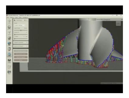
555 nodes are being created. Now, it has produced the supports here you can see the supports are ready, you can see here advantage of choosing mesh mixer is that we can provide ergonomic support structure to our 3D printed file. One of the issues that is to be considered here the supports are very easily removable here. So, this is 1 of the issues that should be taken care of so, because the tip dia is 0.5 mm that can be easily removed here.
