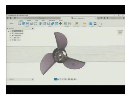
Now, this is the component that is imported here. But this is a propeller this was broken somehow and it is scanned to be 3D print again. So, this is a 3D image scan. With traditional manufacturing processes, it is very difficult to create objects or scan.
