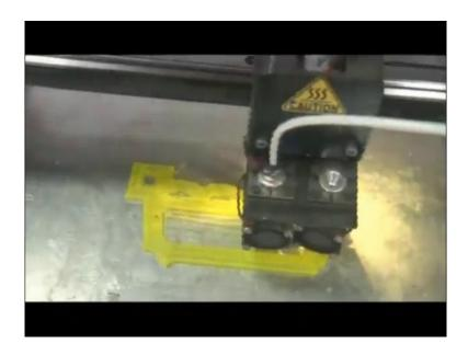
It is now printing, it is printing, this is the brim command that we mentioned before and brim is, brim fabricated before, actual model. So, this is the very first line that is being drawn by the machine.
