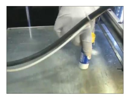
So, this is distilled water with some cleansing agent here, few drops, some of the liquid cleaner is spread and it is cleaned with the help of spatula so, the whole machine had there is actually glass, so we have to be careful, what is this white milky gear, white milky material? It is nothing but, we have used Fevistik that is the adhesive material, this Fevistik.
