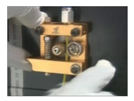
So this is, these are our rollers, we are taking it off. We are unloading the filament now, okay unloading the filament you can see, again this is the filament of size 1.75 mm. Now, we can see that the filament is little distorted from the tape that is it would not enter the rollers properly.
