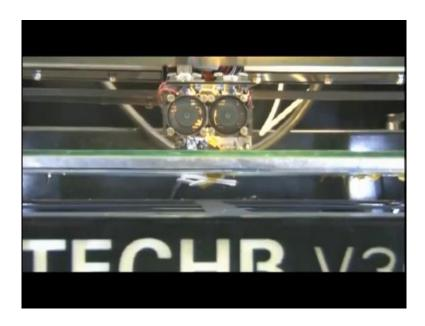
Before print preview, we will just come to manual control here. In manual control, so we are going to check manually that whether the things are moving up. Yes, we are checking the materials is coming in, materials is coming out you can see the materials is coming out, so we are manually checking whether the feeder is working or not, okay.
