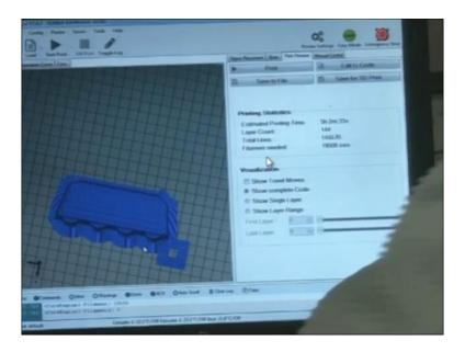
So, there are two nozzles here, extruder nozzle extruder 1 and extruder 2. Extruder 1 and extruder 2, two nozzles are there so accordingly we have two nozzles here, extruder 1 and extruder 2 we can put the material, what is the kind of material? We have put it ABS for extruder 1 and ABS for extruder 2.
