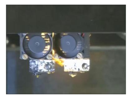
This is one more thing that we mentioned earlier, there are two fans. Fan 1 and fan 2 here, the two fans here, fan 1 and 2. After fuses it becomes viscous, and for the long time, it will deshape the CAD model, if it is not properly controlled with a structure temperature. So, after depositing, these fans are responsible for the cooling and solidification of the layers.
