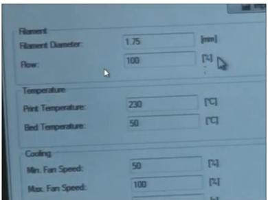
So, this is the filament, so it is in the form of a wire, again the diameter is 1.75 mm, then we see this flow, flow is 100 percent that means, whatever input we give, whatever speed with feed input we give, it will run a 100 percent in that speed only. So whatever we are going to input so it will work in that, according to that only. The next we can talk about temperature.
