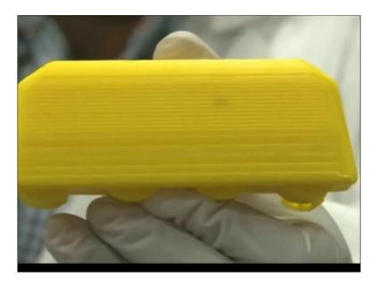
So, this is brim that is taken off from the job that is pre-fabricated. So, this is the model that would be developed. So, this is the pocket, this extra material is brim, this extra material is brim, and this whole material is brim.
