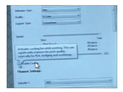
So, this is we are talking about the slicer and we were talking about the support and then speed, speed as we discussed speed in speed as it is fixed to 40 millimetre per second outer perimeter speed is 6 to 20 millimetres per second, and inch feel speed is again 40 millimetres per second. We can make it fast and slow using this tab as well.
