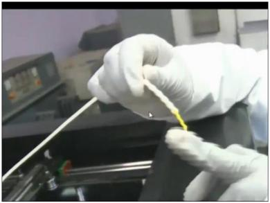
Now, this is our head this our and there are heaters here that are heating. The filament, the spool is coming through this tube, the white tube, the filament is coming through this white tube. So, this is the head that can be moved, or this is our X and Y movement, Z movement that actually bed is moving up, and down that movement is controlled with bed and they are two nozzles here, the only one nozzle is active at this point of time.
