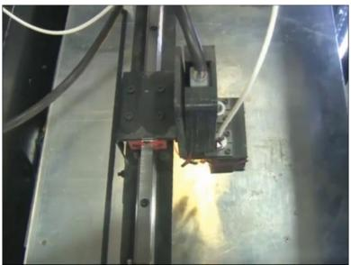
We can see that the loading of filament is properly done. Now, we can see that whether the filament is coming through the nozzle or not? Yes, it is coming. Now, this means the temperature is now maintained, now we will use this two clips to hold the glass with the bed, with a table bed.
