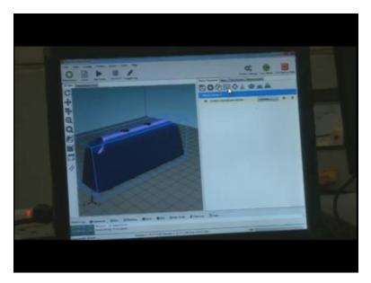
So when we need to print at the centre, auto positioning will bring the object at exact center in the envelope. So we need not to drag it like we were dragging before we need not to drag it. Next one is center object, auto positioning, auto positioning it will position the object so as the least material is used.
