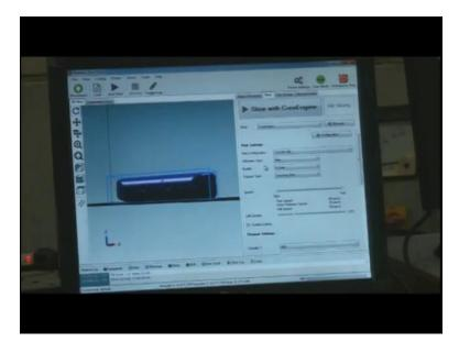
So, this is I can see the most important tab because we are going on discuss this slicing here. So, slicing with Cura engine. So, Cura engine is the software that is used for slicing here. So slicing the time used in V30, this machine, V30 is Cura engine. So, it cares the quality of the product that we need to manufacture, it will discuss everything like thickness, wall thickness, quality, support, then volume, time.
