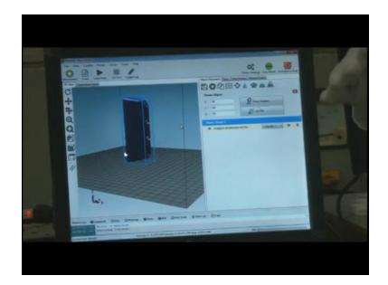
So, we rotate and try to keep the CAD, CAD is meant about this model computer aided design model we have I will use keep on using the word CAD for this model, this CAD is kept in proper alignment so as to minimize material use the y is kept 0, x 90, z 90. So, if y is kept again 90, so the height increases, what is the drawback when we increase height?
