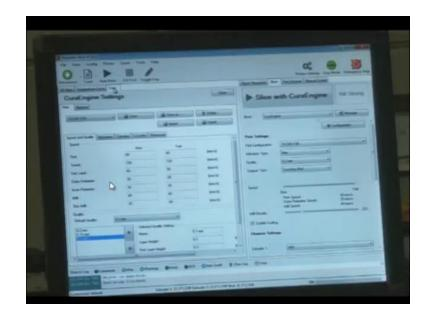
So this is 3D Cura, 3D view includes understanding via 3D view, temperature curve in Cura. Temperature curve we can just see when we actually do machining. So nozzle, at the nozzle heaters are there, heaters supposed to heat so to fuse the raw materials, heaters are heated. So, the orifice, at from the orifice, the material would come and this temperature would be shown in the window.
