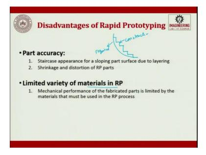
So, there are some disadvantages of rapid prototyping or rapid manufacturing. The part accuracy is very important. So part accuracy means when you have a curved surface, when we try to move along the x and y direction, you have this type of error. So, this is what is the required and this is what is the constructed, I am just zooming, okay.
