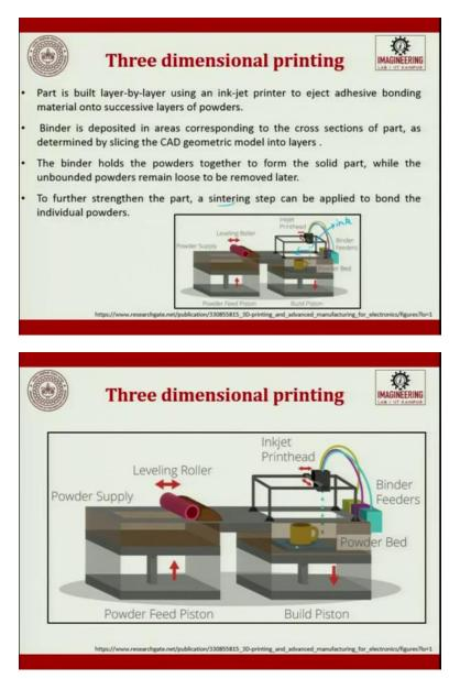
The three-dimensional printing is the next area. So, we saw selective laser there, ceramic can be used, metal can be used, plastic can be used, elastomer also can be used. So the three-dimensional printing. So, this is another niche area which is coming out. So, here the part is built layer by layer using an inkjet printer.
