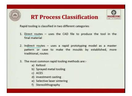
So rapid tooling process classification, there are two types which are done, one is called as direct routes and, the other one is called as indirect routes. The direct route uses the CAD file to produce the tool in the final material. Indirect routes are use a rapid prototyping model as a master pattern or case to make the mould by established more traditional routes.
