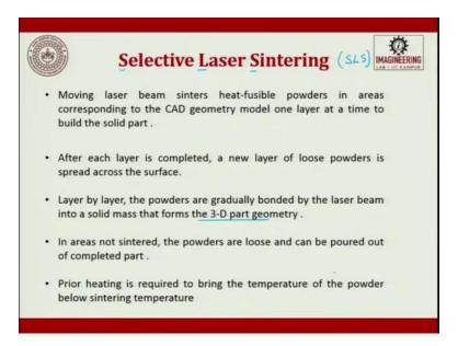
The most popular one amongst this is used exhaustively today is selective laser sintering, which is otherwise called as SLS. Moving laser beam sinters heat fused powders in areas corresponding to the CAD geometry model, one layer at a time to build the solid part after each layer is completed, a new layer of loose powder is spread across the surface.
