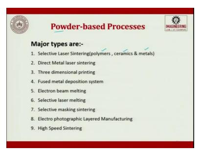
So, there are different types, which falls in the powder-based processing. The major types are going to be selective laser sintering which can be polymer, which can be ceramic, which can be metal-based.
