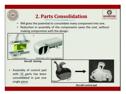
Second thing is the rapid manufacturing is used for part consolidation. Earlier rapid manufacturing you earlier we used to produce 6 parts and 8 parts that will be a lot of amount of material also can be reduced which is very much required for aerospace industry and automobile.
