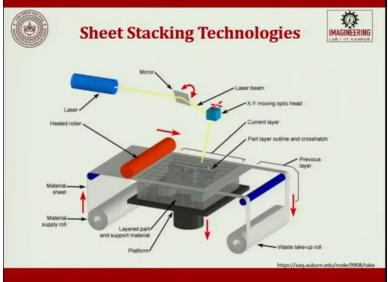
The next one in the solid is going to be sheet stacking technologies. So in sheet stacking technologies, the solid physical model made by stacking of sheet stock, each outline of the cross-section shape of the CAD model that is a slice into a layer. Okay, so I would repeat solid physical model made by stacking layers of sheet stock each an outline of the cross-sectional shape of a CAD model that is sliced into layer.
