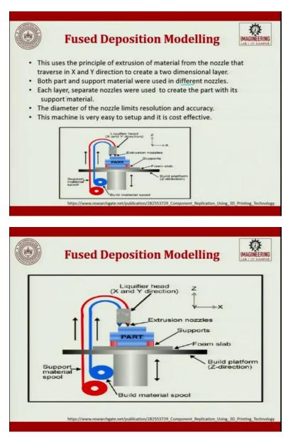
So, this is the process for fused deposition modeling. The use, this uses the principle of extruding. So, here the wire is fed into through an extruder. So, then what happens there is a tension which is maintained by two rollers through which the wire gets fed inside.
