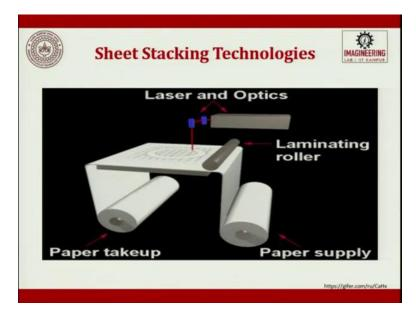
So, you can see here the zip file is given which will help to understand more the layer is there then the heated roller then it is in roll, out roll. So this is a paper supply there is a paper take-up. (Refer Slide Time: 15:47)
