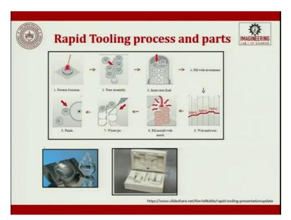
So, you see here rapid tooling process and how is it used to develop parts. So, the pattern creation will happen through a laser then the tree assembly is done. So, after the tree assembly, we try to insert it into here flash or into a container where there is a ceramic slurry, then, we try to fill with investment, then we try to melt the wax.
