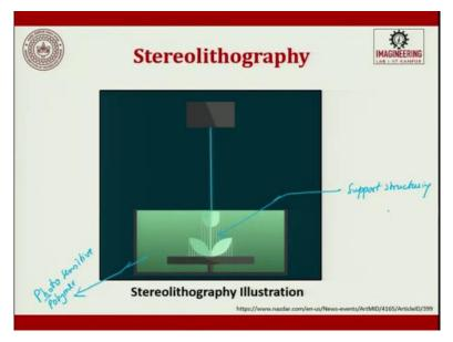
So this is how if you see the animation, it looks like. So here you see that there are straight lines which are there. So these straight lines are nothing but support structure. They will be removed, I said post-processing steps. So in the post-processing steps, all these supporting structures will be removed. So here is a laser and this is a photosensitive polymer. So when I say photo you can use light for curing it.
