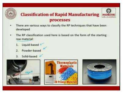
When we start going into rapid manufacturing process, there are several techniques used, basically, the rapid manufacturing or the rapid prototyping processes are classified based upon the starting material. There are several ways of classification. One way of classification is to start with the form of the material whatever is available, so there can be liquid-based, there can be powder-based and there can be solid-based.
