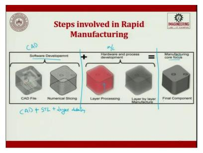
So this is what we have discussed until now. So we will try to divide it into two steps so this first step is all done in a CAD software, so software development a CAD file is drawn, so here then you make facets then after facets, you will try to make layers. So CAD, then CAD then the next step is going to be STL, then it is going to be layer by layer, layer detailing, that is what it is nothing but the slicing.
