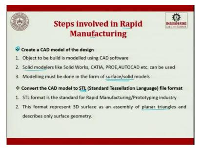
So what are all the steps involved in rapid manufacturing or additive manufacturing? First step is going to be create the CAD, the first few lectures what we saw in the CAD, first two weeks we discussed about CAD, so creating a CAD model of the design is the first step in the rapid manufacturing.
