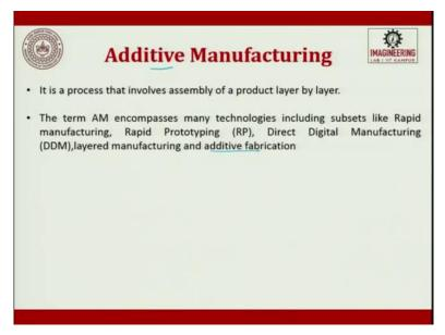
The next one is additive manufacturing. It is a process that involves assembly of your product layer by layer, okay. So for example, if you want to construct a 3D object, even today what we do is we divide into several small pieces, so these pieces can be something like a cuboid or it can be a work-cell.
