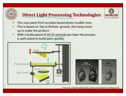
The next most popular process which is commonly used today is direct light processing technology. This uses parts of acrylate-based photocurable resin. So here what happens, till now it was all laser was on the top and the object it was projecting projected on to the vat or the photopolymer tank, it was just projected there. But here in DLP, it is going to be vice versa.
