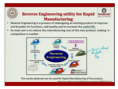
The next important thing, so we are going in the front route where we have points, point to lines, lines to surface, surface to solid we went. The other way is also possible, we try to do reverse engineering of the existing object and try to develop either the same or the negative of it. So reverse engineering utility for rapid manufacturing. Rapid manufacturing also use reverse engineering.
