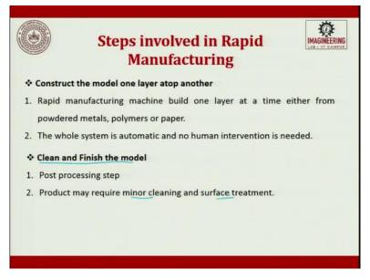
The third one is going to be construct the model one layer on top of another. So the third step is going to be layer by layer, that is going to be the third step. So now you have made facets after that what you do is, along the Z direction you cut the object into several thin layers, right? After you cut this thin layers, the next step is going to be construct the model one layer atop another.
