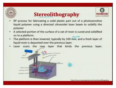
This is what a stereolithography process all about. RP process for fabricating a solid plastic part out of a photosensitive liquid polymer using a direct ultraviolet light, laser beam which tries to fall on the polymer and try to solidify. So it is one spot now overlapping of spots will be there, so now what will happen? It will try to produce a single layer.
