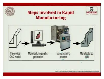
So this is what is given in the picture form, that was given in a schematic form this is given. So what are you trying to generate in this software numerical here when you start doing it, so you are also trying to develop not only layer by layer when you do layer by layer you are also trying to develop the path, tool path motion. You are trying to develop a tool path motion, okay.
