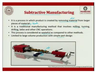
So, in manufacturing, you have several verticals. One major vertical today wherein which we do lot of mass customization is by doing subtractive manufacturing process. In this process in which the product is created by removing material from large pieces of material or suppose removing chip from the blank or a raw material.
