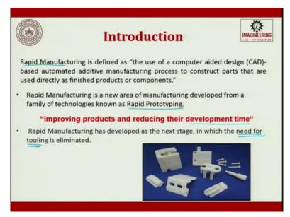
So to define rapid manufacturing, we are using this definition, the use of CAD-based automated additive manufacturing process to construct parts that are used directly as finished products or components is nothing but rapid manufacturing. There is a big difference between rapid prototyping and rapid manufacturing.
