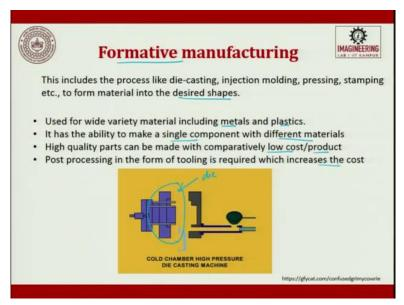
The next one is formative manufacturing wherein which it is a constant volume process there is no change in volume between the raw material taken and the output produced, so this includes the process like die-casting, injection molding, pressing, stamping, etc to form material in the desired shape, so here you will have a die, and this will be a die.
