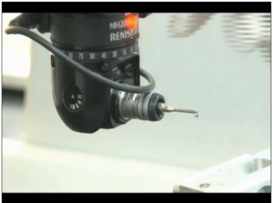
We have actually this is LVDT, this is LVDT. We have 3LVDTs, each axis has an LVDT. These LVDTs for Z-axis, so for inside the column above, we have for Y-axis, here we have for Y-axis and also we have for X-axis as well here. This is a probe, we can rotate it to (90) 180 degree. This is 180 degrees.
