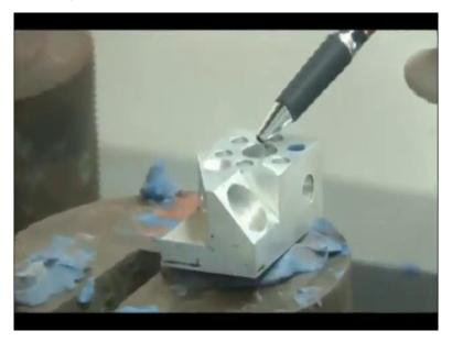
So we have got the origin point here that is a centre point, origin point here, the centre point of the cylinder is the origin. So next is how to measure all the parameters? We can select the circles here, these 6 circles, okay. This is cone here as well.
