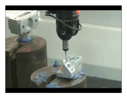
So this is our workpiece, the features of which we are going to measure. So we will take 3 points from this plane, 3 points from this plane. So this is our cylinder, this is cylinder. What is display? This is ZY plane, this is ZX plane. What is this stop plane? This is XY plane. So this we have selected plane, plane 1. It will try to record the points at least 3 points are required to define a plane.
