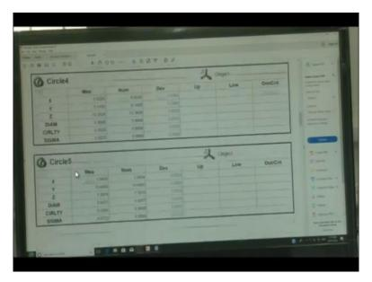
So this is an element list. We have generated this plane and the dimensions of the plane X, Y, and Z, measured nominal, what is deviation. Then up-low and did you know these deviation these distribution, not exactly distribution but tolerances can also be obtained from here.
