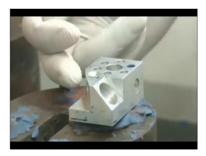
In the construction, we can click angle, now it will ask between which entities you need the angle? Plane 1 and plane 3. So the angle between plane 1 and plane 3 is 45 degrees. So this is the angle it is showing 45-degree angle. So similar to the angle we can also measure the distance between cylinder 1 and circle 1.
