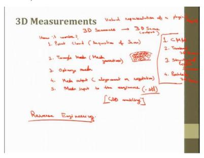
3D measurements, what are 3D measurements? 3D measurement is a process of creating measurement or virtual 3D representation of a physical object. This is virtual representation of a physical object. Now 3D scanners are optical devices used to create 3D measurements or 3D scanners. We have 3D scanners. 3D scanners if I say 3D scanners the outputs are known as 3D scans, 3D scans is the output.
