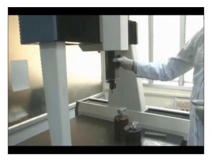
This is 3D object that we will measure using this co-ordinate measuring machine, okay. We will try to measure the features of the job, of this component. So you can see there are number of circles here. Okay, there center circle, center cylinder here, okay, we have circles here. Then we have 6 cylinders around the center cylinder. Okay, I will just measure this full cylinder. Then I will this 6, 1, 2, 3, 4, 5, and 6. I will measure try to locate these 6 circles, not the cylinders.
