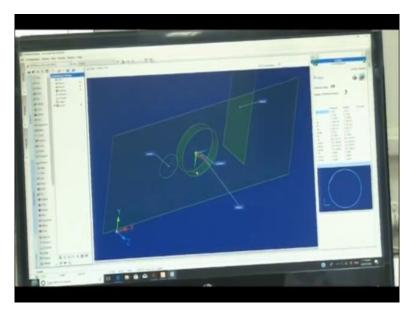
So to measure the circle, we will select circle from here, then measurement parameters, so it is trying to retract from the 2 mm, we have entered 1, so at least 3 points are required to locate a circle.
