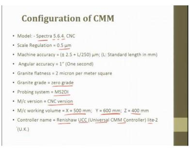
So the CMM machine that we have here, the configuration of that is it is Spectra 5.6.4. What is 5, 6, 4? 5 is 500 and 600 and 400 is the work area or workspace that is available in the 3 axes. 500 mm, 600 mm, and 400mm, okay. Then scale regulation is 0.5 micrometer machine, accuracy is  $(\pm 2.5 + L/250)$  micrometers, so this L is the standard length in mm, so angular accuracy is by one second of the angle.
