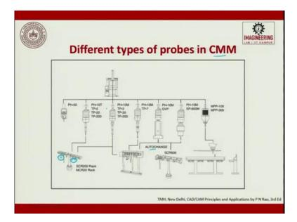
So, different types of probes in CMM a use star it is not only one, these are the different types of probes you will have. So, you can have link there, you can have star type so, you can see a ring-type so, these are multiple probes which are used. Okay, and like in CNC machines here also you can have auto changes where this tells the probes are changed and the head will be the same.
