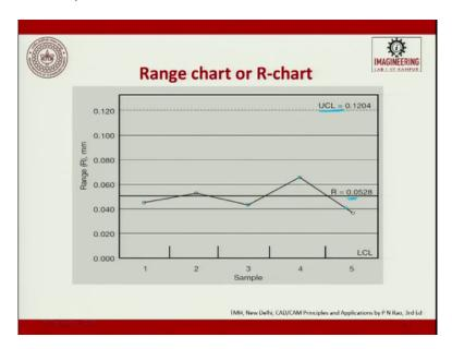
So, if you see an R-chart this is the range and you can see the samples how have the samples, are performed. So, the UCL upper critical level is 0.104 the range is 0.0528, so now we say whether the process is under control or not. So, this is typically a chart which shows how the
