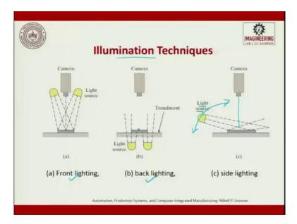
So, the illumination techniques it can be front side, front light it can be light from the back it can be light from the side. So, front side is when there is an opaque table and then object is moving on opaque table then we do this, and backlight is whenever we try to do biological samples we put it on a glass plate put, the sample here and light is thrown from the bottom.
