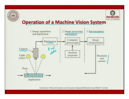
So, the operation of a machine vision system this is what happens in the acquisition I gave you an example of a camera with a flash so, you see here a light source is thrown on a part so this tries to lights are thrown and from the thrown lights you try to capture an image through a camera. So, now whatever image you are captured through the camera, will be then digitized. During the digitization, the analogues data is converted into pixel data.
