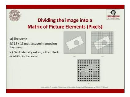
Then now, the dividing the image into a matrix of pixels so, it is a scene, this is the photo you have taken and now, you divided into a matrix, so  $12 \times 12$  matrix is superimposed on the object and wherever there is a completely dark that means to say, there is no image present it is declared as black and wherever there is an image it is declared as white, there are certain portions where there is a mixture of black and white.
