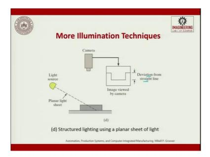
So, the more illumination techniques is also there. So, we have a structure light, this is a structure like the light source falls on a planer light sheet, so you will try to get a structure light which falls on it now, from the structured light we try to acquire the data and try to take the image. So, this is the deviation of the straightness. So, we can also have light source which is structured.
