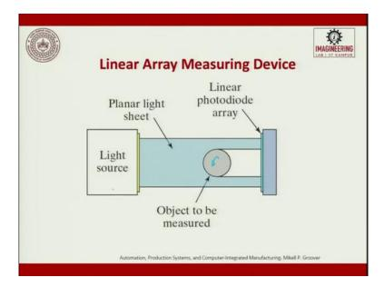
The next one is a linear array measuring device so, you have a light source wherein which you have linear and this passes through a plane, light passes parallel to it so, you have a linear photodiode so, light source falls so, again on off, ones and zeros with a, in the photodiode is there, the object is kept in between.
