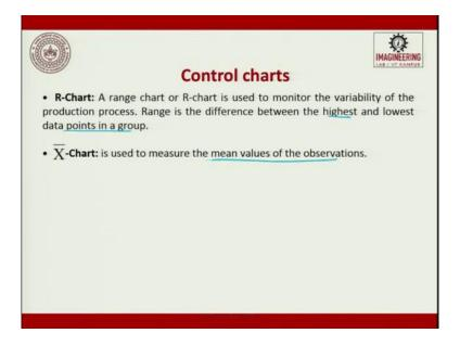
There are two major control charts, R-chart, a range chart, or an R-chart is used to monitor the variability of the production process. Range is the difference between the highest and the lowest data point in a group. So, this is R-chart, we also have an x-bar chart, which is used to measure the min value of the observations.
