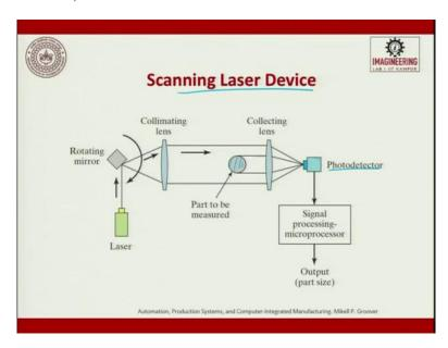
This is a scanning laser device technique so, wherein which what we use is we, use a laser the laser hits at a rotating mirror this rotating mirror the light is passed through a collimating lens then it goes to another collimating lens and then if you keep the path which is there in between.
