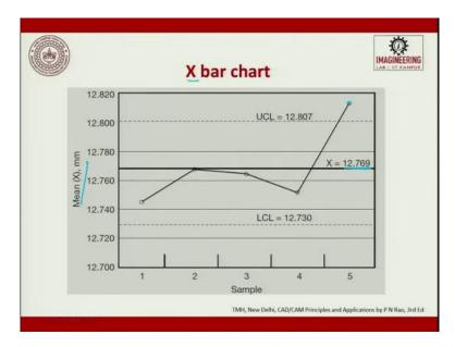
So, if you look at the x-bar chart we will see the min chart, so UCL is 12.807 lower, upper control, lower control between these two. There is an X which is the mean 12.768 and you will see the process is going out of control when it crosses the limit. So, this chart is called a x-bar chart.
