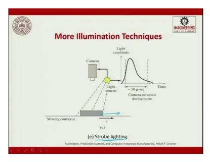
This is a strobe lighting so, in strobe lighting, this is a moving conveyor is there. So here is a light source and then we try to see this is the light amplitude and this is the camera, this is the time in seconds. The camera actuation during the pulse you see it goes during this side, and this is trying to take care with a moving velocity and object moves, and the camera captures. We use strobes lighting technique.
