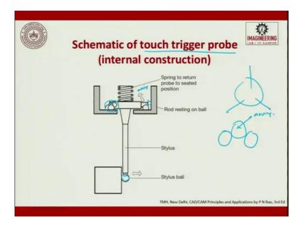
This is what is the internal construction, so you see here, this is the stylus ball, this is the stylus so, this is sitting, resting, it is a three dimensional one. So, it is resting, this is one, here you will have two and the backside you will have three. At 60 degrees each, it is almost this is what is the resting position where this probe is sitting and the spring to return probe to the seated position.
