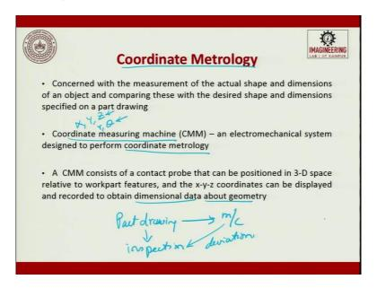
When we talk about coordinate measurement so, these two if we go to P to Q chart it is more of manual assisted measuring. When we talk about coordinate measurement concern with a measurement of the actual shape and dimensions of an object and comparing these with the desired shape and dimensions specified on a part drawing. So, what is that you have developed a part drawing you have used it for machining and now, same part drawing is used for inspection.
