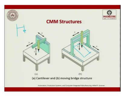
So, this is a typical cantilever type this is a cantilever type okay so, there is an overhand and there is one more overhand then you have a stylus which touches and then you try to get the output. So, if there is an error in this stylus, it is transfer to this and so, naturally, the error data whatever you measure is going to be tricky to handle.
