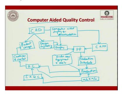
So, how does it happen is, first we will have a CAD, from a CAD it is attached to computer-aided drafting and documentation. From there the data goes to computer-aided process planning. From the process planning, it goes to a process planning. Then, from here, you have a drafting, this goes to process planning.
