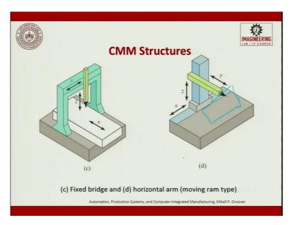
So, it will not be carried so, the third one you can have is fixed gantry but a moving table. The next one is horizontal arm so, the difference between the horizontal arm and the cantilever type is, there is a horizontal and then there is a vertical, here there is only horizontal so, if you have a large component and if it is along a plain and you want to measure it along the vertical axis then we use this horizontal arm.
