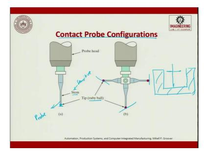
So, the most critical part is the structure wherein which the resolutions, all these resolutions repeatability, reliability, precision, all these things are taken care of. But, the heart of the CMM comes from the probe. So a probe has a spindle to hold the probe, this is the probe. This is the probe head and this is the probe.
