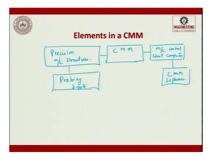
What are all the elements of a CMM? You will have a precision machine structure, this leads to a coordinate measuring machine, you will have machine control unit computer, then you have a CMM software, then you will have a probing system.
