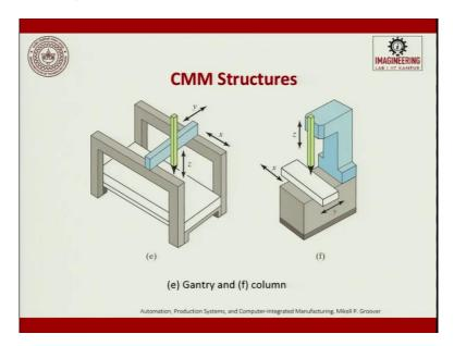
Then you have a gantry type which is used and then finally it is also a column type. These are the 6 common CMM structures which are exhaustively used in the factory environment. So, Thank You.
