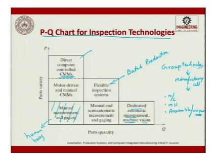
When we try to put PQ chart for inspection technique this is P and this is Q, this P is path variety and Q is path quantity. So, here if you see manually measuring and gages where and which we use human-oriented work is done here. So, here a human being is exhaustively used in measuring. Next, if you slowly move out the same thing if we could automate it is manual and semi-automatic can be done if it is more quantity lesser variety then we go for dedicated measuring machines.
