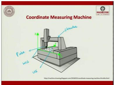
So this is how a CMM works so here is a part so, the this is a probe so, this is the structure what moves, this is the structure and you have this is the probe and then this is the well coordinate system and here, you will have a user coordinate system and here the probe touches the work peace and wherever you see a dot points these are all the points.
