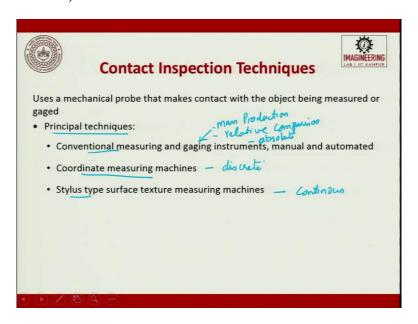
So, contact inspection techniques uses a mechanical probe that makes contact with the object being measured or gaged. The principal techniques are conventional measuring and gaging instruments, gages, gages are only used to for mass production and they are generally used to have a relative comparison. They will not give you the absolute value, absolute value cannot be there. If you just measure and say okay, that deviation, it falls within the deviation you are getting it.
