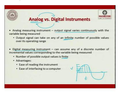
So, there are two types of instrument which are generally used for measurement one is called as analog the other one is called as digital. There is a mixed opinion people say all analog instruments should be converted in to digital and we start using the data but, now people say that digital puts a restriction on increasing the resolution more.
