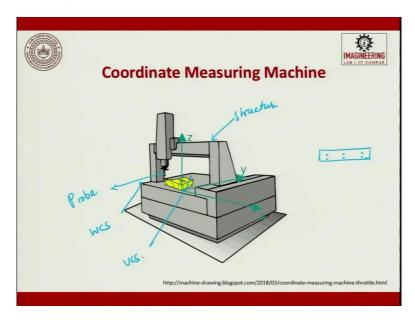
Suppose, you want take a plain so it touches 6 points and it tries to generate a plain surface. So these are the points the data points are taken and then, the data is now using a help of a computer and then we try to get the data.
