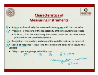
The characteristics of measuring instruments, first is accuracy. We have seen accuracy and resolution in robotics we have seen in CNC, a quick recap of the same accuracy. How closely the, they measured value agrees with the true value is called as accuracy. Then resolution, the smallest variation of the variable that can be detected is called resolution. Between these two you have one more terminology which is called as precision.
