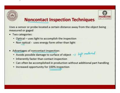
So, when we talk about non-contact inspection techniques use a sensor or a probe located a certain distance away from the object being measured or gaged. So, two categories, one is optical uses lights to accomplish the inspection, non-contact uses energy form other than light. So, the advantages of the non-contact inspection, is avoid possible damage of surface objects that is what I said, soft materials, it can be skin, it can be rubber, it can be PDMS whatever it is.
