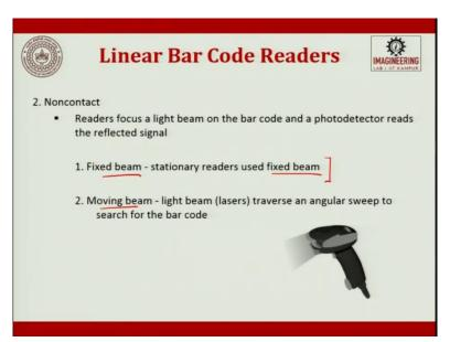
So, next is a non-contact bar code reader. So, in these readers, focused light of beam on the bar and the photodetectors reads the reflected signal, it is kind of a fixed beam and moving beam. So, this is non-contact or stationary readers used fixed beam. As I just mentioned, like in the big shopping centers, moving beam, the light beam (lasers) transverse an angular sweep to search for the bar code.
