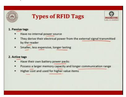
The two major types of tags are there. Passive tags and active tags. The passive tags are the ones that have no internal power source. They derive their electrical power from the external signal transmitted by the reader. So, these are passive. These are smaller and less expensive and longer-lasting. Active tags are the one, which has a transponder in them, they have their own battery power packs.
