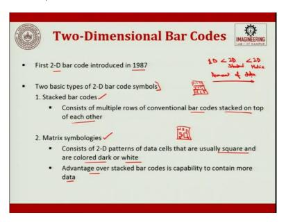
So, next is a two-dimensional bar code. The two-dimensional bar code was first introduced in 1987. The two basic types of them, number one is stacked bar codes. Number two is matrix bar code. Matrix bar code, as I took the example of the QR code in general that is matrix—QR code for WhatsApp when I picked that is a matrix kind of a bar code. So, this stacked bar code, what are they? These consist of multiple rows of conventional bar codes stacked on top of each other.
