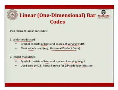
Now, what are the major kinds of linear bar codes? One is width-modulated and the other is height-modulated. Now, width-modulated bar codes are a symbol that consists of bars and spaces of varying width. These are the most widely used that is UPC. I will discuss what is UPC and core-39. Height-modulated. This symbol consists of bars and spaces of varying heights. These are majorly used in U.S Postal service or zipcode identification.
