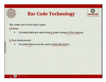
So, I am not going into the detail of this. This is just an overview of how the AIDC system works. Next is bar code technology. So, no the error rate in bar code technology is approximately ten thousand times lower than in manual keyboard data entry. The error rates of the most of other technologies are not as low as bar codes but are still better than manual methods. So, the bar code is also too economical to use.
