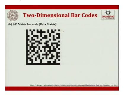
Next is matrix bar code, this is how matrix bar code looks like. So, it consists of 2D patterns of data cells that are usually square and colored dark and white. These are up to thirty times denser than code 39. Code 39 is before; this is around thirty times more than a code 39 can create. However, there are more complex type bar codes and they require more sophisticated printing and reading equipment.
