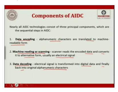
Now, components of AIDC. An AIDC system typically consists of three major components. Data encoding, machine-reading and scanning, and data decoding. What is data encoding? So, data encoding here implies that data has to be used by the computer, it has to be readable by
