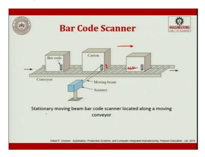
Like this is the conveyer that is going. This is the kind of a moving beam because beam is moving up and down. Suppose if the beam is also fixed if the bars are like this. The fixed beam can also sometimes read that. Whenever the beam—supposed this is the beam, if it covers—I will put beam with some other colour. So, this is the beam, if it covers this whole code, it might be able to read that.
