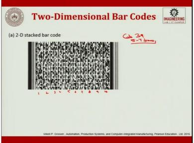
The 2D barcodes stacked and matrix. This is how a stacked bar code looks like. It is 1, 2, 3, 4, 5, 6, 7, 8, 9, 10. Ten barcodes stacked horizontally here. So, it typically consists of the multiple rows of conventional bar codes stacked on top of each other or just stacked side by side. The data's density of stacked bar codes typically five to seven times, here it is ten times. For linear barcode 39, it is five to seven times. Generally, five to seven times, the bar code is repeated.
