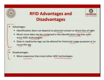
So, advantages and disadvantages. The advantages are the identification does not depend upon physical contact or direct line of sight. Much more data can be contained in the identification tag than with most AIDC technologies. The data in read/write tags can be altered for historical usage purposes or to reuse the tag. So, the data can be reused. The larger number of data can be put in here and identification does not depend upon the physical contact.
