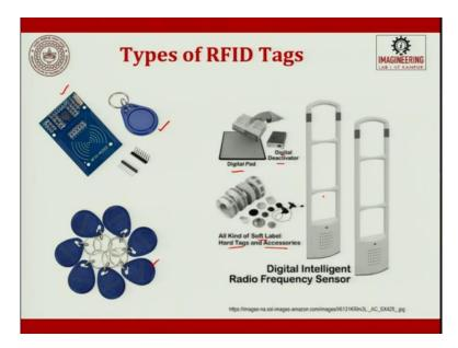
So, these are a few kinds of typical RFID tags. So, the tags are in the keyring. Here we have this reader circuit and this is one set of it. So, this is the digital pad, digital deactivator. These are the kind of soft label hard tag than accessories. So, this is a radio frequency sensors like the antenna is there that helps to emit and then get the information.
