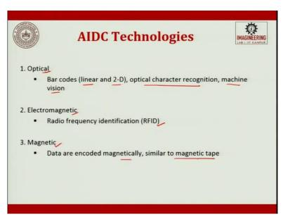
These are the major components of an automatic identification system. So, these systems can be optical, electromagnetic, magnetic, and so on. In the optical system, we have generally the barcodes. Bar codes can be linear of two dimensional, optical character recognition (OCR) and machine vision. These are optical characters. I will discuss about these.
