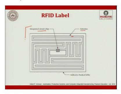
However, RFID are generally two types that is active and passive. This is an integrated circuit chip and antenna. This is an RFID label. This also has to be printed. Now, before talking about these things, an important factor is printing. Printing of bar codes, the printing of RFID. In many applications, the labels are printed from medium to large quantities for product packages and for carton used to ship or packaged box in case of bar codes.
