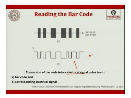
Now, conversion of bar code into an electrical signal, how do we read bar code? Reading means, the bar code is decoded here. So, this is a sweep of light beam. The light beam travels here. It is converted into an electrical signal here, this is an electrical signal. So, this signal gives the information or transfer information to the next step.
