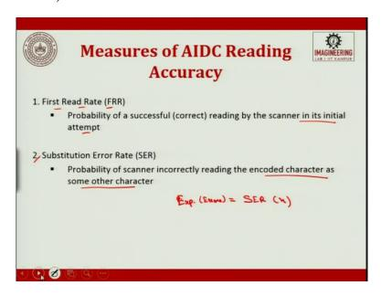
Now, measures of AIDC reading accuracy. The accuracy of the data that is represented there has to be high. There are two major measures for that. First is the 'first character reading'. Next is that if the first character is not read properly then what is the subsequent error in the further characters.
