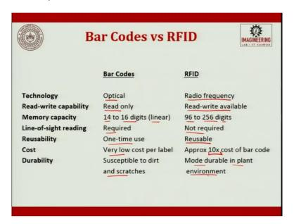
Now, a few major differences between bar codes and RFID. The technology for bar code is optical. The technology here is RF, radiofrequency. Read and write capability, the QR codes can read-only. RFID can write as well. Memory capacity is 14 to 16 digits. For linear it is 96 to 256 digits.
