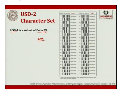
Now, this is a subset of code 39. How does it look like? This is just an example here. So, this is USD-2. Now, the reason this code 39 name given to it is that it has nine elements that is bars and spaces, which are used in each character and three of the elements are wide. The placement of wide spaces and bars in the code uniquely designates the character. Each code begins and ends with either a wide or a narrow bar.
