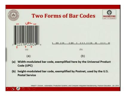
Now, what are these? These are the kinds of width-modulated and height-modulated linear bar codes. So, this is a width-modulated bar code that is a UPC. This is a height-modulated bar code that is a, used by Postnet in U.S Postal service. So, what are these? In a width-modulated
