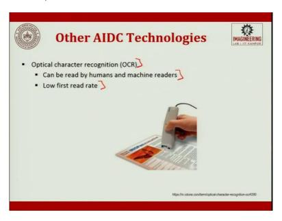
Similar to magnetic tapes, we have optical character recognition. It can be read by humans and machine readers, so it is a low first read rate. So, it is just used to read the data by humans and the data is then converted, the characters are recognized and data is converted into the soft form.
