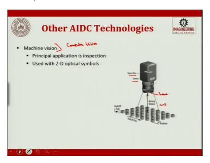
Similar to that is machine vision. Machine vision is a very wide or big topic. Similar to machine vision, we have computer vision. When we talk about robotic or artificial intelligence, computer visions come into play. Machine vision principle applications is in inspection that is what is the distance between them? What are the number of components those are there?
