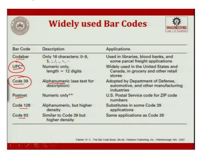
Now, widely used bar codes, these are general barcodes, which are being used in the industries these days as it was just mentioned UPC before. UPC is a universal product code. So, that is numeric only and length is 12 digits. It is widely used in U.S, Canada in grocery and other
