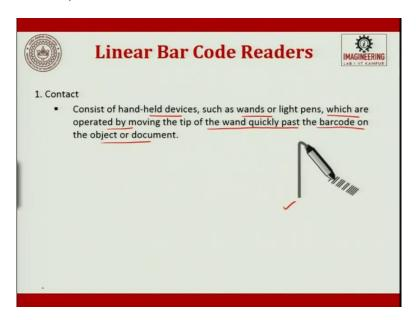
So, what are the contact bar codes again? It consists of handheld devices such as wands and light pens, which are operated by moving the tip of the wand quickly past the barcode on the object or document. This is the kind of contact bar code reader.
