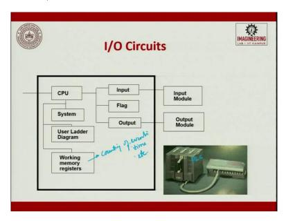
So, the input/output circuit, if you see, a CPU will be there, a system will be there. You will have a user ladder diagram will be there. Then there will be a working memory space. Working memory is used for counting of events, time and etc. So that is the working memory registers. So, whatever gets from the ladder diagram, so if there is a flow of one data signal so that will go get recorded and here and it keeps on adding.
