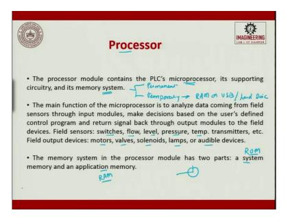
Next, we will see about the processor. The processor module contains the PLC microprocessor, its supporting circuitry, and its memory system. So, your processor will also have a memory system. Memory you can have permanent and temporary. So temporary you can have through your RAM space or you can use it through USB or a hard disk. Possible, right?
