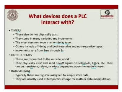
Then we have a timer. These timers also do not exist in physical form like a clock. It is inbuilt inside the PLC. So here, what happens, it counts internally. They are maybe in many varieties and increments. The most common type is an on-delay type. The other includes off-delay and both retentive and non-retentive types. The increment varies from 1 millisecond to 1 second.
