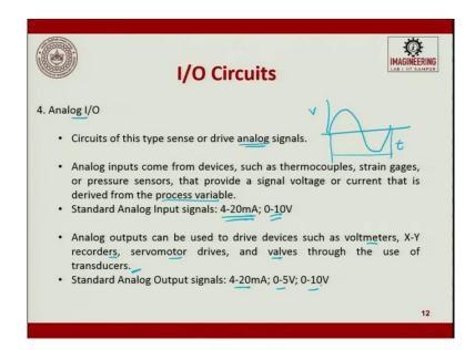
There is a need today to work on analogous input/output also. The first three what we saw was discrete. Now, we are trying to see the analog input/output. The circuit of this type sense or drive analog signals. Analog signal or continuous signal because for a period of time, I would like to discretize to my requirement. So in that way, I would like to play with the analogous signal.
