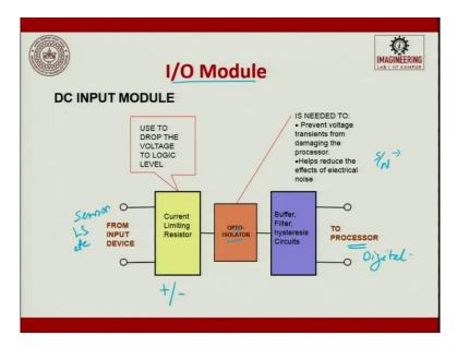
So, the DC input module, we are discussing about DC. Today, you also have AC. So, these are input. So, the current limiting resistor used to drop the voltage to logic level. So, we use here current limiting resistor. Then we have an optoisolator, is needed to prevent voltage transients from damaging the processor we have here optoisolator that helps to reduce the effect of electric noise.
