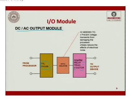
So, AC/DC output devices, we saw two input devices, now we will see AC/DC output devices. So here, from the processor, we will try to take a TTL signal and then send it to an optoisolator. TTL signal is a transient logic. So here, we will try to see whether it is plus five, minus five.
