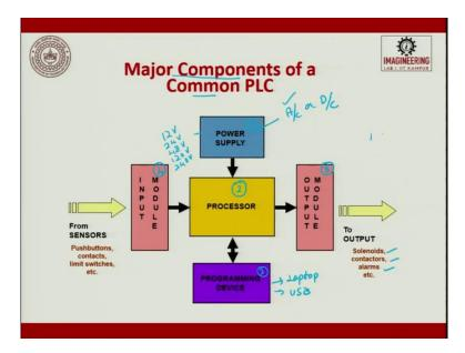
When we talk about the major components of a PLC, you will have a power supply. This power supply can be AC or DC. Generally, today what we do is we try to use only AC power supply because DC conversion—that is a huge amount of losses. So, we will use an AC power supply for it and here you will operate it from 12 volts, 24 volts, 48 volts, 120 volts, and 240 volts.
