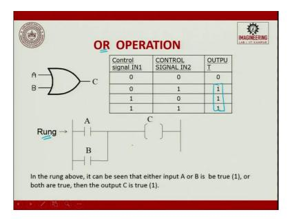
NOR operation. If A is 0, B is 0. C will be 0. If A is 1, B is 0. C will be 1. If B is 1, A is 0, C will be 1 and if A and B are 1 then C will be 1. So, you can see is nothing but an OR signal. So, this can be represented in a rung form like this. A, B OR form. If it is AND, it will be together. If it is rung OR type then the rung will have like this. In the above rung, it can be seen either A or B, if it is true then C will be true.
