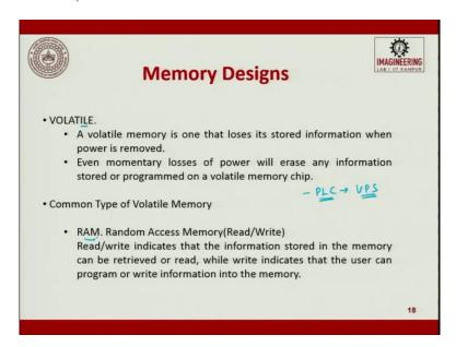
The memory devices are volatile. Volatile memory is one that loses its stored information when power is removed or when you press a reset button. Every momentary loss of power will erase any information stored and programmed on the volatile memory chip. So that is why, in PLC, you will also try to have a UPS attached to the machines so that it tries to give supply for some more time before it is getting shut off.
