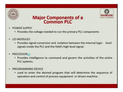
The power supply provides the voltage needed to run the primary PLC components. Input/output modules provide the signals, conversations, and isolation between the internal logic level signal inside the PLC and the field's high-level signals. So, input/output devices are basically for in and out. The processor; provides intelligence to command and govern the activity of the entire PLC system is done by a processor.
