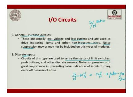
So, general-purpose output. These are usually low voltage, low current which is used inside a CNC machine automation system low voltage, low current, and are used to drive indicating lights and other non-inductive loads. For example, today you have a smartphone. Through a smartphone, you are able to control the intensity of the lights, switching on of the AC, all these things.
