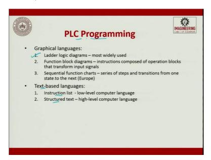
What are the different types of PLC program? We have graphical language, three. One is called a ladder logic diagram, most widely used. Function block diagram, instruction composed of
