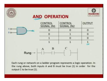
AND operation. This is how you try to draw your device. So, which is it has two in and one out. So the control signal in 1 is 0. The control signal in 2 is 0. The output will be 0. So, the control signal will be 0, B will be 1 and the output will be 0. If the control signal is 1 and B is also 1 and then now you will try to get an output as 1. So, now what you will do is, you will write this program in this form, whatever we did here, we will write it in one rung information.
