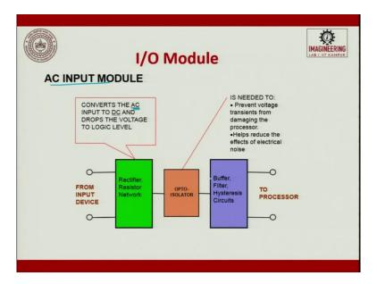
AC input module, an AC input module, you have a rectifier resistor network. So, the rectifiers function is to convert the AC input to the DC signal and drop the voltage to the logic level. So here, we did not have that, we had only resistor network but here you will have a convertor with us. Then you will have an optoisolator, the same function what it does and then you will have a buffer, filter, hysteresis circuit, etc.
