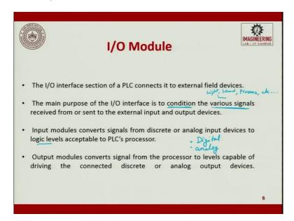
The input/output interface section of a PLC connects it to the external field devices. The external field devices are sensors, limit switches etc. The main purpose of the input/output interface is to condition the various signals received from or sent to the external input and output devices. Conditioning, conditioning of various signals. Various signals can be light-based, can be sound-based, can be presence-absence, etc.
