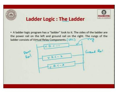
What is a ladder logic diagram? It is otherwise called as a ladder. A ladder logic program has a ladder look of it. The sides of the ladder are the power rails on the left and ground rails on the right. The rungs of the ladder consist of virtual relay components. So, for example, I will try to draw a ladder logic diagram. So, this is the power rail on one side. This is the ground rail on the other side and then you have rung.
