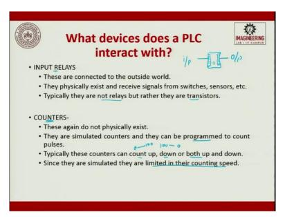
What devices does a PLC interact with? It interacts with input relays. These are connected to the output outside the world. So, PLC input is also outside world input, this is output. This is also output world but we can see but this is also an output world where we can see. So these are connected to the outside world. They physically exist and receive signals from switches and sensors.
