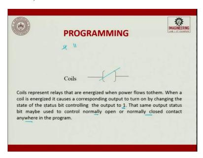
A coil represents relay that is energized when power flow to them. When a coil is energized, it causes a corresponding output to turn on by changing the state of the status bit controlling the output to 0. That same output status bit may be used to control normally open or normally closed contact anywhere in the program. So, are you able to understand? Coils represent relay. These are coils, so you can have normally closed and normally open and then this in turn, attached to your coil.
