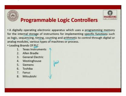
What is a programmable logic controller, PLC? A digitally operating electronic apparatus which uses a programming memory for the internal storage of instructions for implementing specific functions such as logic, sequence, timing, counting and arithmetic to control through digital or analog modules, various types of machine or processes.
