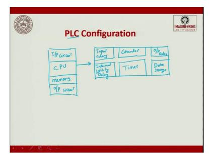
Let us now see the PLC configuration. For PLC configuration, which we have already seen but now I will put all the bits and piece information into one block diagram. So you have a CPU, you have a memory, you have an output circuit, you have an input circuit. This, in turn, is attached to data storage, so all the program, which is executed 1-0's, will be there.
