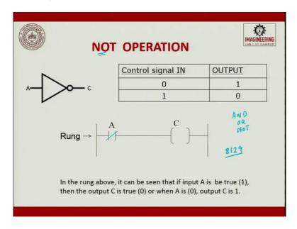
You can also have your NOT operation. If A is 0, B will be 1 or C will be 1. If A is 1, C will be 0. So here, you can see that A is normally closed and you put this. If the rung above, it can be seen that if the input is true then the output is true-0 or when input is 0, the output will be 1,
