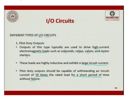
The different types of I/O circuits. Pilot duty output, the outputs of this type typically are used to drive high-current electromagnetic loads such as solenoids, relays, valves, and motor starters. So, what is a solenoid? The on-off switch is a solenoid. Valves open-close, motor startstop we have a motor starter circuit today, so, where need a very high current. So, pilot duty output is where the output of this type typically uses to drive a high current electromagnetic load.
