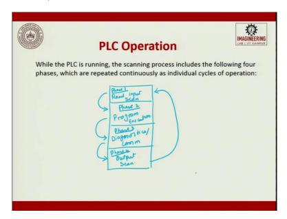
So, while PLC is running, the scanning process includes the following four phases. I will draw the phases, which are repeated continuously. As individual cycles of operations. So let us put four phases. S, phase one, it is 'read input scan'. Phase two is 'program execution'. Phase three
