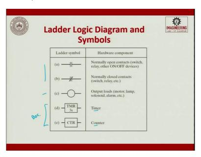
So, in a ladder logic diagram, these are the symbols used. Normally the open contact, switch, relay, other on/off devices, we give this. When normally closed, we say this. When output loads such as motor, lamps these are for inputs. These are output loads of motor, lamps, solenoid,
