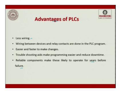
So what are the advantages of PLC? PLCs since earlier we used to have a lot of wire connections, now the PLC uses less wire. The wires between devices and relay contacts are done in the PLC program. Easier and faster to make changes. So since it is programmed based, it is very easy. Troubleshooting aids making the program easier and reducing downtime. Reliable components make also make this like to operate for years before failure.
