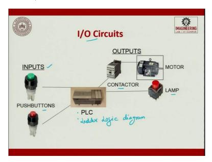
So, when you talk about input/output, so input device is a button. This is a push-button. This is a toggle switch, something like that. So input signals, you will have a PLC then PLC in turn connected to the contractor which in turn, starts a motor or it drives to switch on your bulb. So these are the inputs, all the processing information is done in the PLC, which follows a ladder logic diagram.
