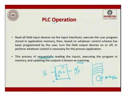
When we talk about the PLC operations, read all field input device via the input interface, executes the user program stored in the application memory, then based on whatever control scheme has been programmed by the user, turn the field output devices on or off, or perform whatever control is necessary for the process application.
