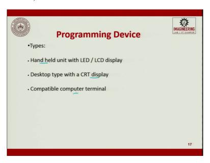
The programming devices, there are three types which is handheld like your manual entry in the CNC machine. You have a hand held units with LED/LCD display. You have a desktop type with a CRT display. Then you have a compatible computer terminal.
