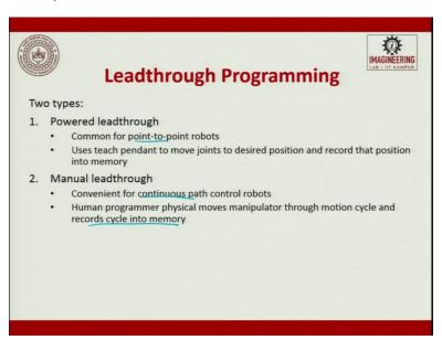
Leadthrough programming again there are powered leadthrough and manual leadthrough. Commonly it is point-to-point and manual leadthrough is continuous, this is very important. Uses a teach pendant to move joints to the desired position and record that position. So, it might move in a bang-bang position, start/stop.
