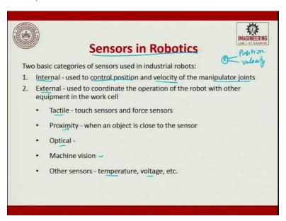
What are the different types of sensors which are used in robots? There are two basic classifications in sensors; one is called as internal sensors, the other one is called as external sensors.
