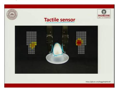
So, this is a tactile sensing device. A tactile sensing because lifting an egg is a huge challenge because an egg is not circular; it is not a sphere. So, it has a shape which keeps changing and there is a radius and here the gripper if it is flat. You will never get a proper contact.
