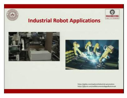
So, this is a typical pick and place robot you can see, and then these are robots, where there is welding which is happening. And these welding you can see there, the object is twisted moved up and down and then you can see the gun which is attached to a gripper.
