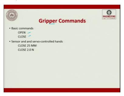
The gripper commands can be basic OPEN/ CLOSE or it can be CLOSE and WAIT OR CLOSE with the load. So, it will be 25 millimeters, CLOSE at 2 Newton's.
