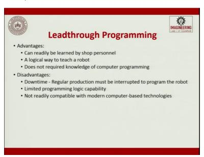
So, the advantages can easily be learned by the shop floor man. A logical way of teaching a robot; does not requir a knowledge of computer programming. It is something like a semi-scale labor can teach. So, here, the disadvantages are the downtime – regular production must be stopped to the program the robot. Limited programming logical capabilities; not readily compatible with the modern computer-based technologies is leadthrough programming.
