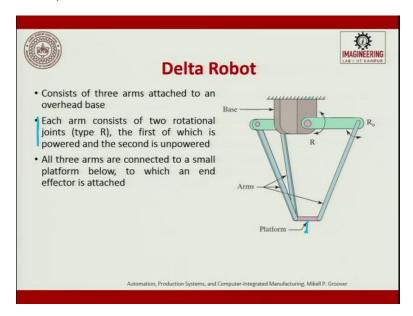
The last one is called as delta robot. Delta robot consists of three arms attached to the overhead base. This is an overhead base and each arm consists of two rotational axes. The first of which is powered and the second is unpowered, very-very important. So, one is powered and the other one is unpowered. All the three are connected to a small platform, this is a platform. So, you can have a drilling machine, milling machine or you can have a positioning device whatever it is.
