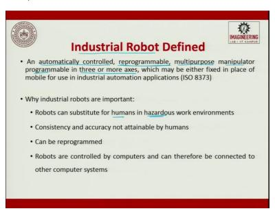
When we talk about industrial robots and automatically controlled, reprogrammable this is a very-very important word. Multipurpose manipulator programmed in three or more axes, which may be either fixed in place of mobile for use in industrial automation application, is the definition for industrial robots. So, the important things are automatically controlled, reprogrammable, multipurpose manipulator programmable in three or more axes; this is very important.
