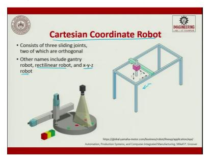
Next, is Cartesian Coordinate Robot; this is a Cartesian coordinate robot where we will have three linear joints x-axis, y-axis, and z-axis. So, all three are linear, so the work volume that it generates will also be linear. Rectilinear robot and x-y-z all are linear joints. So, this is basically used again for pick and place depending upon the sorting.
