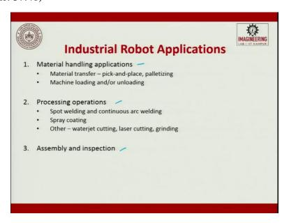
So, applications, material handling applications we have discussed, pick and place, and unloading. Then processing: spot welding, spray coating, water jet cutting, heat treatment etc. Assembly and inspection, these are the three areas where industrial robots play a very-very important role.
