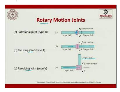
Then rotational, you have an input there is a joint which is fixed and this is able to rotate. So, this is a joint and then this swing in this direction; so this is rotational. Twisting is about this axis if it
