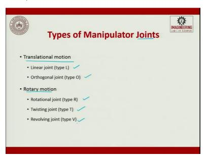
So, when we talk about types of joints we have two major classifications; one is linear I said translational, the other one is Rotational. In translational you will have two things: one is linear joint and the orthogonal joints. Under rotational motion, you will try to have rotational joints, twist joints, and revolving joints.
