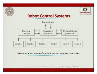
When we talk about robot control systems input, output. So, there is a program store and then there is an executive processor and then there is a computational processor. So, these are the joints which are linked to it. This is a typical hierarchical structure of a robot microcontroller used. So, we will have a program which is stored and then we will have a computational processor. This is the executive processor so input, output is given, joints are given there.
