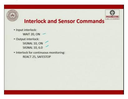
So then interlock and sensor commands are given, so wait 20 seconds or 20 milliseconds. SIGNAL 10 is ON, SIGNAL OFF, then REACT SAFETYSTOP YES/NO.
