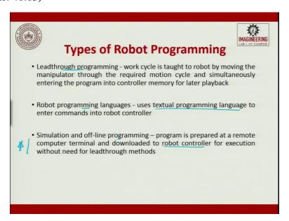
So, types of programming which I just discussed; leadthrough programming, robot programming through language, simultaneous and off-line programming. Leadthrough programming – a work cycle is taught to a robot by moving the manipulator through the required motion cycle, and simultaneously entering the program into a controller memory for later playback. So, it is just like holding a blind man walking through.
