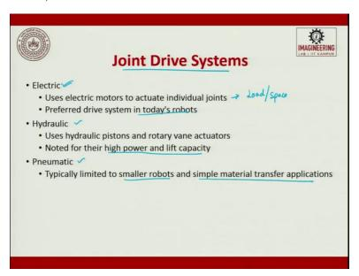
Joint Drive Systems: see you have now only put the joints. Now, each joint has to be activated, so how do you activate? This can be activated by three types. One, it can be done through electrical way; it can be done through a hydraulic way; it can be done through a pneumatic way. The most commonly used one is electric drive because its load per space whatever it is using is very high.
