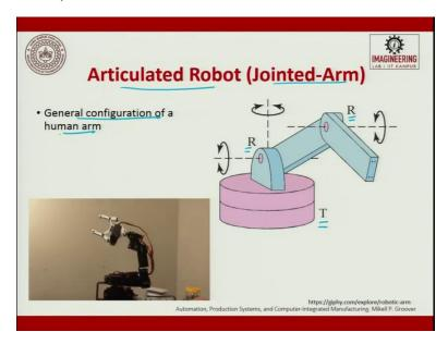
So, this is a typical articulate robot or the joint robot. So, you will have a base and when you see that please look at the acronym, this is twisting joint, rotational joint, rotational joint. So, if you go back twisting joint then rotational, rotational.
