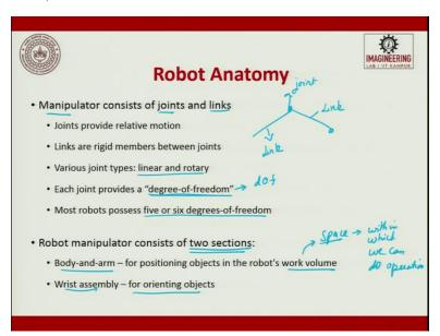
When we talk about manipulator; manipulator consists of joints and links. So, joints provide relative motion, what is relative? I had a link, I have a joint, I have a link. So, this joint is going to bring relative motion between these two fellows. So, links are rigid, this is a link; these links are rigid members between joints so this is a link, this is a joint.
