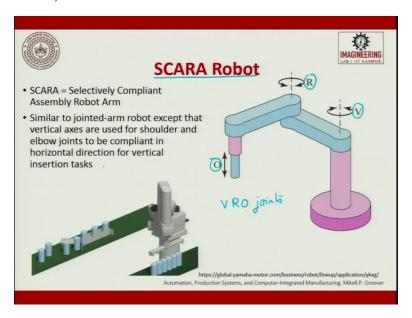
The next one that I was explaining to you is SCARA robot which is very commonly used. SCARA robot stands for, Selective Compliance Assembly Robot Arm. Similar to joint robot arm except
