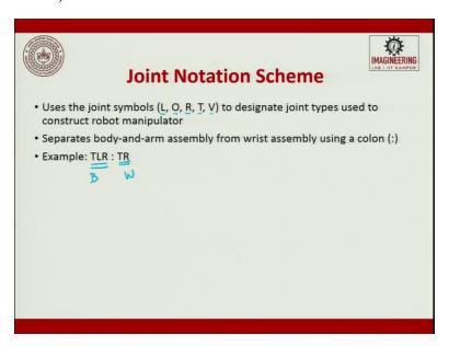
So, the uses of the joints symbol L, O, R, T, and V to designate joint type used to construct a robot arm. Separates body and arm assembly from wrist assembly using a code dot dot. So, you can see this is for the body, this is for the wrist. So, now if somebody writes TRL; this is for body colon TR it is for the wrist.
