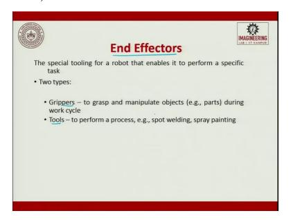
The end effectors for the robot that enables it to perform a specific task. There are two types of end effector: one is called gripper, the other one is a tool. Gripper to grasp and manipulate an object where the tool is to perform a task.
