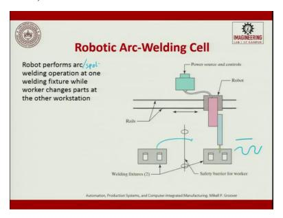
So, robotic arc-welding cell is now a common thing which is coming up, which is exhaustively used in car industry. The robot performs arc welding; arc welding/spot welding if you want. So, arc welding at one welding fixture while the work changes part at the other. So, it is typically like your CNC machines, so one place the new job is getting loaded; the other place the operation is going on.
