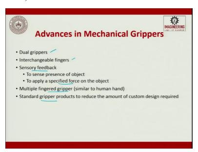
The advances in mechanical gripper are: there are dual grippers, interchangeable fingers, so that means to say you can make fingers like larger, smaller, round, box, prismatic like, helical like whatever it is. Then sensor feedback to sense the presence of an object; to apply a specific force on an object. So, these are some of the advancements.
