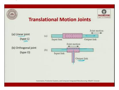
So, this is a typical linear joint, so link input, link output; so here is a joint. So, this is moving along this direction so this is linear joint. The next one is orthogonal joint, which is perpendicular, so you can see that orthogonal joint in link input and this is the output; so joint motion happens like this. So, these are part of translational; translational is to linear joints and rotational joints. By using several of these combinations of joints you make the body and arms structure.
