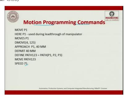
So, this is the motion programming commands, so we will say move P1. So, here P1 used through leadthrough manipulator. Moves P1, then DMOVE (4, 125) these are the coordinates. APPROACH P1 which is 40 millimeters; DEPART from 40 millimeters; DEFINE PATH123, PATH (P1, P2, P3). So, P1, P2, P3 will be defined earlier, MOVE PATH123 with the SPEED of 75. So, this is a motion programming which is used, leadthrough is 1, then it is motion-based.
