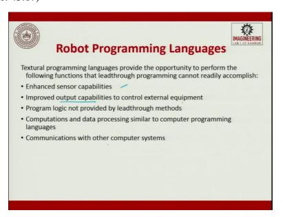
Textual programming takes the opportunity to perform the following functions that leadthrough programming cannot readily do. Enhanced sensors capability; improved output capability to improve external equipment. Program logic not provided by leadthrough methods will be done by robot programming. Computational and data processing similar to computer programming languages can be done by robot programming and communicates with other control systems.
