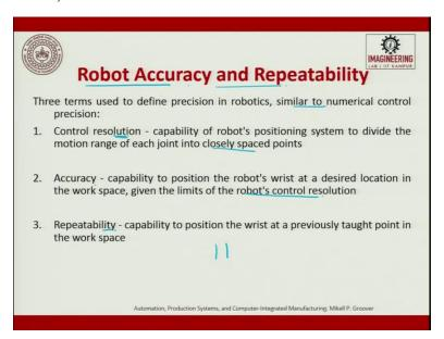
The last part of the robot discussion is, we have to understand robot terminology called robot accuracy and repeatability. There are three terms which are defined as far as robot is concerned.
