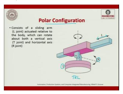
Next is Polar Configuration: Consists of a sliding arm actuated relative to the body, which can rotate about both a vertical axis and horizontal axis; so a vertical axis and a horizontal axis. So, this is LRR; so this is linear, rotational twist. So, here vertical axis will be T and the horizontal axis will be R. So, this is called a polar configuration body arm manipulator. So, this will be written as a TRL configuration.
