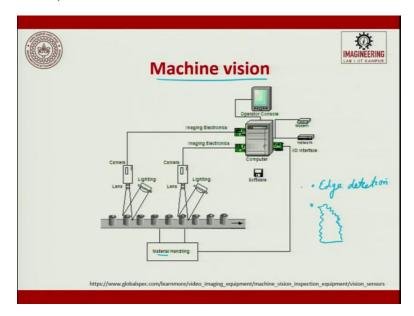
Then we have machine vision today. Machine vision works on edge detection and the other thing is if you have soft material. For example, rubber and if you want to measure the dimensions of the rubber; you want to do it without touching, then machine vision has a very important role. And suppose if you have a very complex texture which is on the surface. It is very difficult for measuring it through any other sensor apart from the machine vision sensor.
