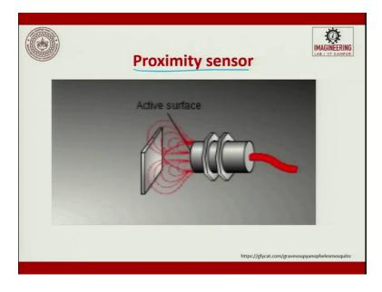
These are proximity as and when the current passes through or voltage passes through it creates an electromagnetic field. And when there is a metal object that comes in that range; it quickly activates senses or there is a metal object. So, then it tries to say yes or no; presence or absence of the sensor, so these are proximity sensors.
