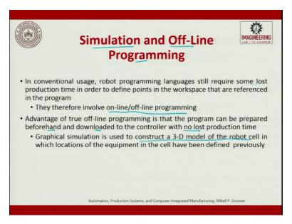
The simulation and off-line programming: In conventional usage robot programming language still require some lost production time in order to define points in the workspace that are referred in the programming.
