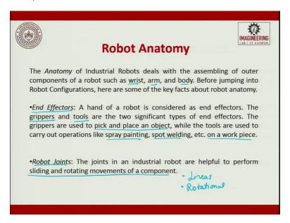
The anatomy of industrial robots deals with the assembling of outer components of your robot such as wrist, arm, or body. Before jumping into Robot Configuration, here are some of the key facts about robot anatomy we should know. End effector: A hand of a robot is considered as end effectors. For example, we talk this is an end effectors. So, this end effectors depending upon your requirements, it can do multiple operations like gripping, and then it can help in loading and unloading of parts.
