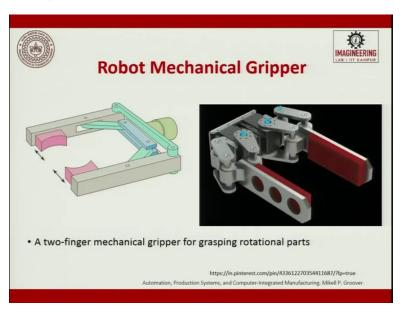
So this is a gripper. So, you can see a two-finger gripper, you can have both the fingers moving or you can have one finger fixed and the other finger moving.
