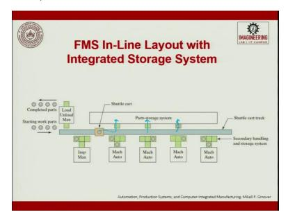
Next, the FMS in-line Layout with Integrated Storage System. So, the only difference between the previous one and this is a parts storage system will be here.
