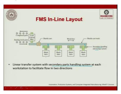
So, FMS in-line layout so here you see that you have a loading station and unloading station. The other thing is these two can be combined loading and, unloading can be combine at one place.
