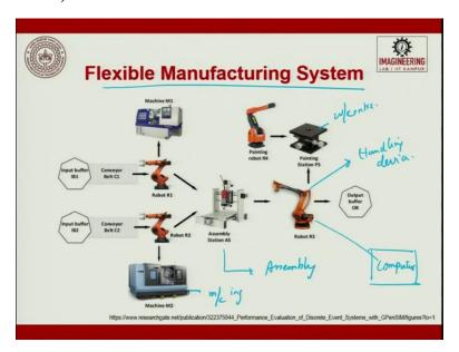
So, this is a flexible manufacturing system. So, here you see a machine 1, then you have input buffer, you have a conveyor. So, from input buffer conveyor comes, your robot takes it and loads it to the machine. After it is machined then what does is, it tries to take the part and keep it here to the assembly station and buffer 2 temporary buffer 2. It is stored for the parts, it is moved in the conveyor, robot is used; it pushes to machine 2 after machining it is kept on here. So, now there
