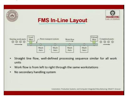
So, this is FMS in-line layout; so here we will see the starting work parts are lined up here. There is a loading station and then you have a conveyor which flows. The parts which are flowing here has to go all these operations machine 1, machine 2, machine 3, and machine 4. However, you are also left with an option of bypassing a station.
