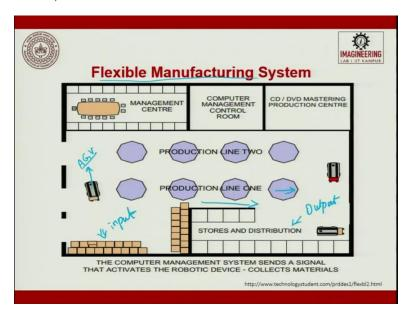
So, when we talk about flexible manufacturing system, flexible manufacturing system, this is a layout of a factory, this is management center and, here it is computer management control system. We will have CDs and DVDs master production center and these are the machine tools and these are the material handling devices.
