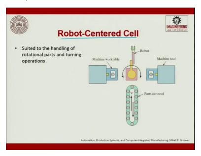
Next one is Robot-Centered Cell. A robot is placed which is used for handling the part between the workstations and the layout.
