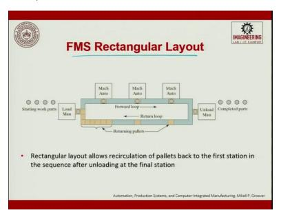
Next is FMS rectangular layout. Rectangular layout allows recirculation of a pallet back to the first station in the sequence after unloading at the final station.
