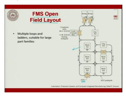
FMS open field layout is you keep adding, and deleting cell itself. So, multiple loops and ladders suitable for large part families can be done. Say for example, you can remove one, add one, you can go through the cell, you can nullify the cell; so each one of a cell of its own. So, you will have an automation so these are open loop system.
