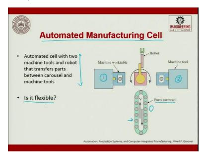
So, this is an automated manufacturing cell. What is automated manufacturing? Automated cell with two machine tools; here is one and here is two. Okay two machine tools and a robot arm that transfer's part between the machines and the carousel. Carousel is something like a conveyor belt in the airport whatever we have. A conveyor endless belt which keeps ongoing where luggage comes inside; and you stand here to pullout your luggage.
