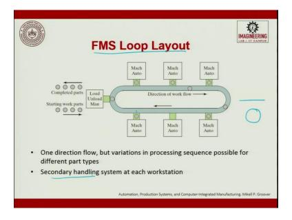
The next layout is FMS loop layout. Loop layout is you will form like a conveyor belts in the airports, so you start here, it keeps coming back to start once again. So, here will be a loading station and unloading station; so the advantages here it the straight line is now converted into a circle.
