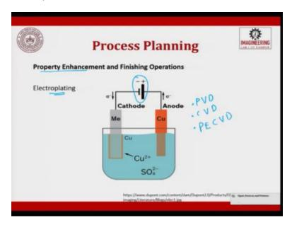
So, Property Enhancement, and Finishing Operation, one such property enhancement, is electroplating also, I was always talking about heat treatment electroplating, electroplating is you have a power supply to Anode and the Cathode, wherever there is a anode. So, you can see the material given and wherever it is a cathode, you can see a deposition happening. So, you can see Copper getting coated on top of this emit.
