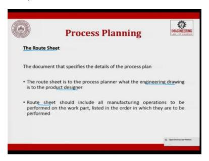
There is another important thing which comes in process planning is a routing sheet, the document that specifies the detail of the process plan. So, routing sheet is to the process planner, what the engineering drawing is to the product designer, routing sheet should include all manufacturing operations to be performed on the work part, list in the order in which they are to be performed.
