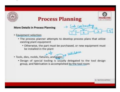
Moment you have understood the sequence, now next comes what are all the Equipments to be decided, for example you have a sheet, which is or a plate of 10 millimeter diameter, it has to be cut, it has to be cut, along a straight line. So, you can do it by water Jet cutting, you can do by plasma, you can do it even by shearing machine. So, any of the three you can choose.
