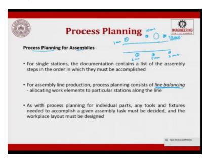
Then this is for a single part, as I told you for a complete assembly if you want to do process planning for assemblies is also done. For a single station the documentation contains a list of assembly steps in the order in which they must be accomplished. For assembly line production, for example a car getting assembled along a conveyor belt it moves, it gets assembled.
