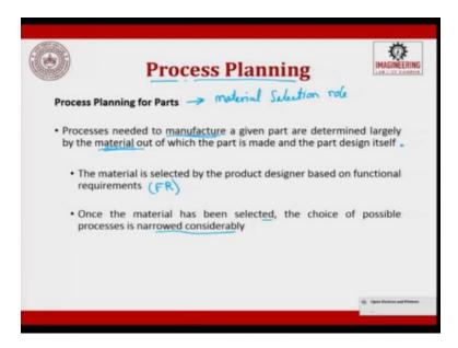
So, when we talk about process plan, the process planning, for a part, the processes need it to manufacture a given part are determined largely by the material out of which the part is made and the part design itself. So, here the manufacturing process is dictated by the material selection and whatever is in design drawing, which is given to you. The material is selected by the product designer based on functional requirements.
