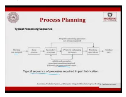
So, starting raw material, basic process, secondary process, then we try to do property enhancing process, I said it can be additional secondary processes sometimes required following property enhancement, or it can be even heat treatment whatever it is, after heat treatment it can do 2, 3, stages of heat treatment.
