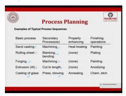
So, when we talk about the typical processes, just an over view, you have the basic process can be Casting, Rolling, Forging, Extrusion, and Casting of glass. The secondary processes can be machining, when we talk about rolling, it is blanking, it can be that is sharing or bending, forging it can be machining, cut off length and the press and blow is only exclusive for glass.
