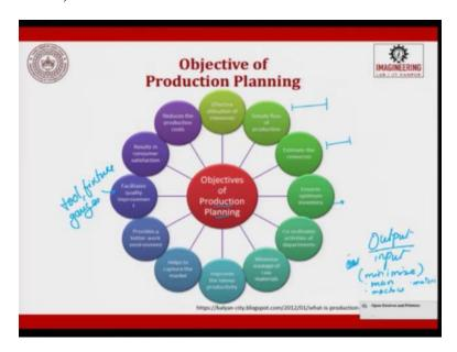
So, what are the objectives for a production planning, its objective should be effective utilization of resources, steady flow of production. So, that means to say throughout the month all 3 shifts they should give employment, eliminate the resources, unnecessary resources whatever it is there, then ensure optimum inventory, because inventory should not be there for a long time, because inventory is nothing but you have invested money of brought it and holding it without utilizing it.
