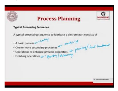
So, Typical Processing Sequence, first will be a basic process we will understand, then what we do is one or more secondary processes we will do, then operations to enhance physical properties and finishing operation, for example casting, let take a simple example it is casting, then we do secondary operations is machining, then we try to do finishing, or we try to do heat treatment enhancing, see it and then finally we try to do painting, or deburring whatever it is.
