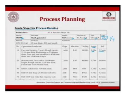
This is a typical route sheet for process planning, for example these are the operation number, this is the description of the operation, this is the department in which the operation has to be done, in the department which machine to be used, in this machine what tool to be used, what fixture to be used, what is the standard, that means to say what is a cycle time. So, setting time, so this is a tool, which is to be used on this machine to produce the part,
