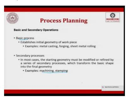
So, when we talk about the basic process is established by initial geometry of the work piece, it can be a casting process, forging process, sheet metal making process, whatever it is. The secondary processes can be machining, and stamping as I told you, which tries to convert a blank into a part as required.
