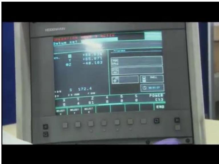
Now, this can be made as z 0 and also this is a new reference point if I say this is at the center, I can put it at x 0, y 0 and z also 0. Now, x, y, z all are 0 here. So, this is our center, so this is our actual reference point, also this is what would be taken by the software will be understood with software as well as the reference point.
