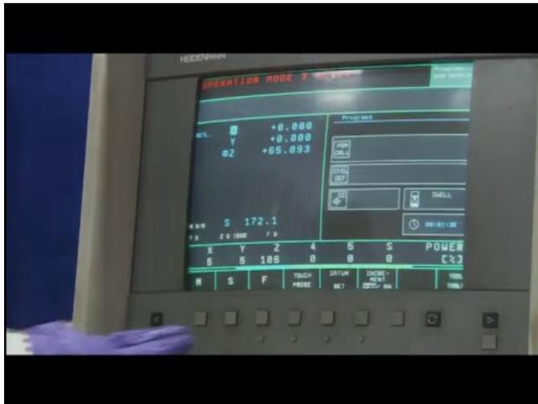
So, this is the manual operation, S is for spindle speed. So, if I say spindle speed, I can put some value, let say 1500 rpm. M 03.
