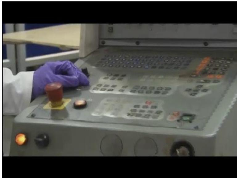
For that we have control panel, we have keys here or the whole keypad is here and some important keys like these knobs are there, feed override and feed under ride also can be charges generally known as feed override. So, there are certain controls MDI Manual Data Input button is there.
