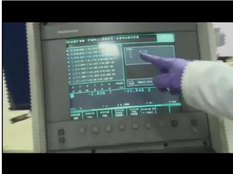
Now, step by step the codes are moving, see the codes are moving the move. See the movement is now going in x and y direction. So, the tool is not moving, the z axis is almost fixed, once the plunging has happened and cutting get started. Now, x and y direction are all taken care by the table, machine table, you can see here, see how rapidly tool moves from one point to the other in the rapid movement.
