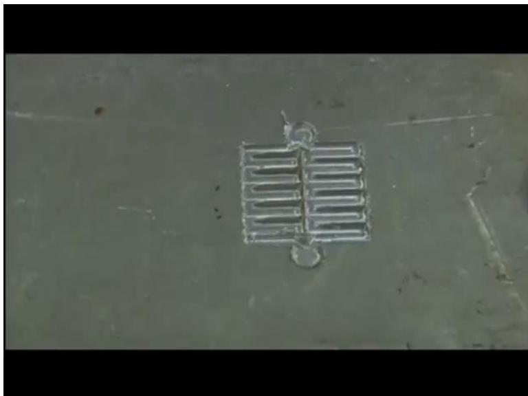
This is the work piece that is generated, it is exactly the profile that we did there. So, let us try to clean it a little bit. So, this is a profile that we have put it there and we have got it here. So, this is serpentine movement, these are straight movement, so we did not do finishing, this is just a rough machining cut that we have made using end milling cutter only, we did not use ball milling machine, ball milling tool to finish it. So, just to show you that how does that happen.
