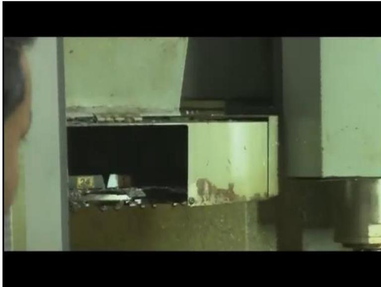
So, in this we have this turret as well, this is also known as tool magazine. It can hold number of tools, it can hold 24 tools, and these tools can be changed while working. As you know, M 6 is the miscellaneous command M 6 is tool changing command, will can put tool number like T 4, M 6.
