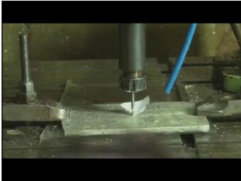
So, what we do? One of the ways is we put a piece of paper between the tool and the work piece. So, slowly we will start bringing our tool down, see, this paper is being rubbed below this it is stuck, let us repeat this. The paper is being moved, once it is stuck it is move, now the tool has just touched the work piece.
