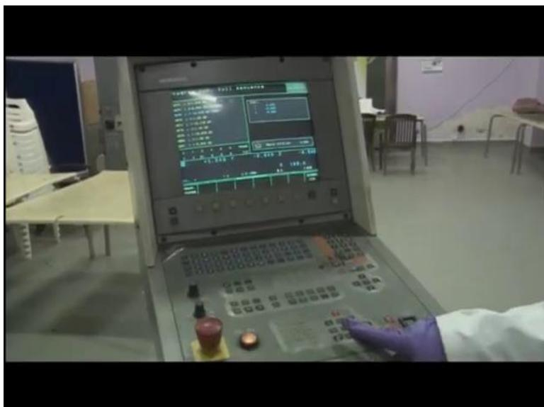
So, also while machining one can observe that whether the machining is going right or not, if any alteration or any changes required that can be put in here by the operator here, he can stop the machine in between and then see whether the machining is going right or not or what is the state of machining.
