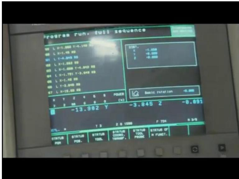
So, the code is running. So, how the job is moving the z direction is moving, we can see the movement on the right side window here, and on the left side the code is running. Also one thing is missing here, this is all the run, I won't say dry run I is a dry machining, dry run is something when we when we try to cut air, when we try to move the tool without a work piece, the work piece is there but there is no coolant that is why it can called the dry machine when no coolant is used.
