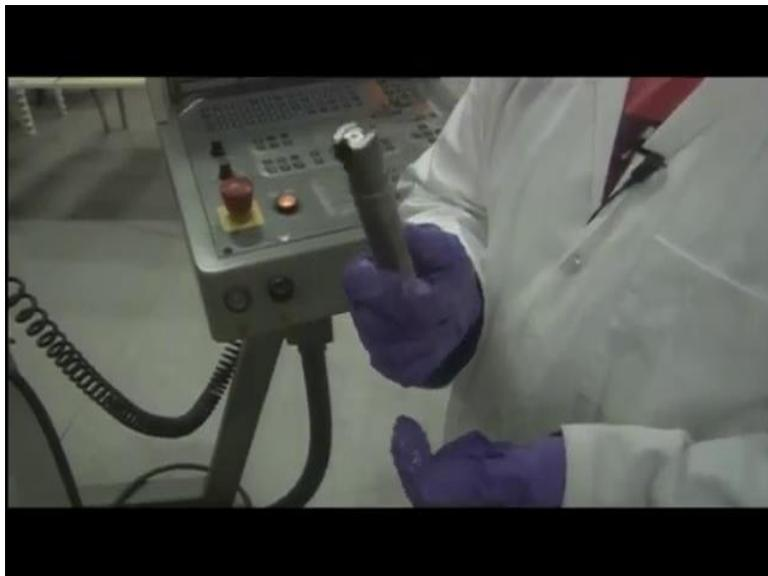
In the same way we have this tool, this is an inserted tool, this is that was a completely solid carbide tool, it means in this tool we have solid inserts. So, this is a tool in which the inserts can be put in and those can be shown, this they can be locked in using a screw, though their sharp tip there. Only the inserts get deteriorated and that can be definitely changed.
