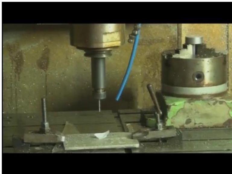
So, if I try to run that, so the tool has been given clockwise rotation, tool is been given RPM and given rotation. So, this these things we can check definitely manually when we feed it here on the control panel. This is clockwise and anticlockwise both the directions are being shown, then x movement, y movement then z movement all the movements can be done manually.
