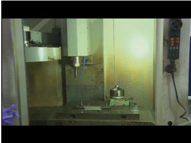
So, in the right hand side, this black control is our handheld control panel, we can hold it on the hand also we can mount it on the machine. So, how does this work, let us see.
