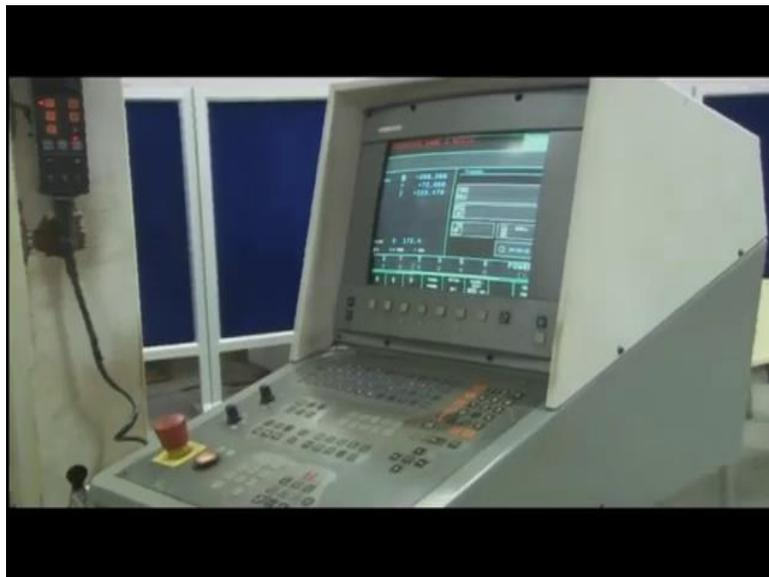
So, this is actually the hardware section as mentioned before this is integrated with the control panel, this control panel that is why it is known as CNC, Computer Numerical Control, this panel has knobs, buttons, keys on it, that can be used for MDI, MDI is Manual Data Input and also the initially we have to set the reference for that that is used.
