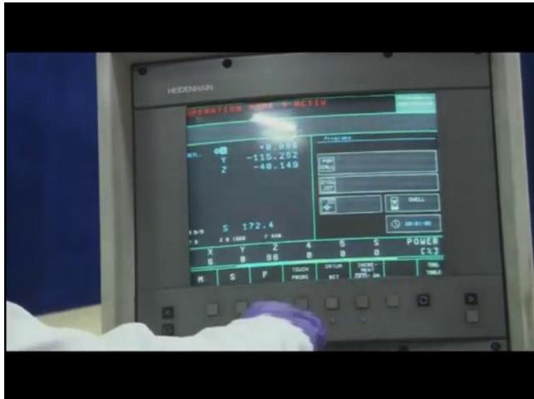
So, let us see how do we make 0, there is the control system this is the present location of the tool based upon the present data or the position that is recorded by computer itself. So, we will see here we put x 0, we will put y 0, enter and x, y are put 0, now as per this position, now the hardware understand or the software here for the machine understand and the software for the machine or the hardware understand that this is x 0 and y 0.
