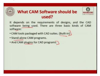
It depends upon the requirements of the designs, and the CAD software being used. There are three basic kinds of CAM software. So, this is again this repeating this is built-in, stand-alone, and plugin, three basic kinds of CAM softwares are there but which software to use. So, if it is a built-in software then it is certain that you would be definitely be more comfortable with the software that is integrated within your CAD suits.
