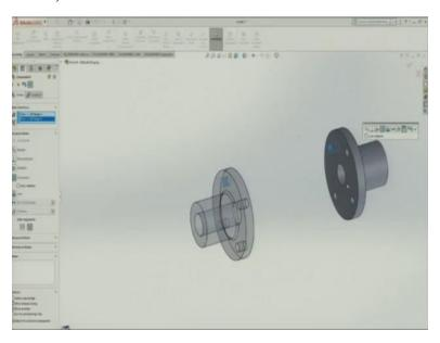
Again I am going to mate command, I am making this hole concentric with this hole. So, this has gone concentric now.
