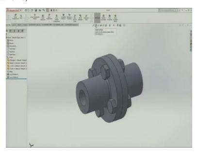
We will make the copies of copies that those are there in the parameters, we need to just rotate it we will make 4 copies of this pattern, spacing I will put 90 degree and did we along what I will put, equal spacing in 360 degree it is better, so yes 360 degree equal spacing. Now, bolts are copied or a pattern of bolt is created. I will accept it, I did not select nut along, similarly we can do the nut, we could have done it together.
