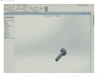
So, these components are here, this is the component bolt, I will change this dimension, so this dimension, I am just making it may be close to 30mm, this should be okay. So, again I am opening the assembly part, in the assembly okay now it looks too good. So, again mate, we have to mate this circle, this hole with this shaft, this is broad concentric, till now it is just mid concentric, axis,
