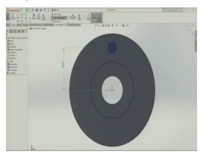
So, shaft dia let me put some circle here. So, shaft dia here is 20 millimeters, so 10 mm would be my radius. So, I will make extruded cut here. So, it has to be through so we can just extend the arrow or we can just put a through hole, both the ways could work. So, through hole that is all. Okay. Through all okay. This is shaft diameter that is made now here.
