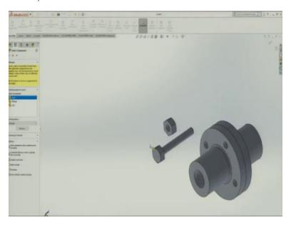
So, I will insert nut here and I will insert bolt here, insert component bolt, so this bolt looks a little larger, the length of the bolt is larger, so now while working as well in this assembly we can change the dimensions for the bolt as well.
