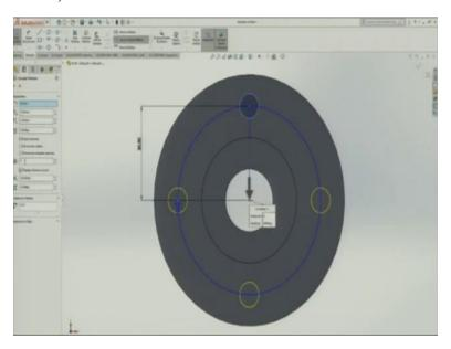
Now smart dimensioning is one of the places that I will show you. The smart dimension is to put the dimension in a proper location, so I need to put this in the centre of this. So, this is I will put value 30mm here, 30mm distance from centre. So, this is smart dimensioning, so this is exactly 30mm from the centre that is in the centre of the flanged part of the coupling. Now, I need to put 4 holes I will put linear sketch pattern here.
