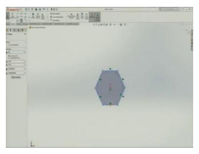
Let me first select bolt to be made here. I will select a plane, front plane here, I will select circle, okay. For bolt I think let me start from the head only, the head for the bolt is hexagonal, let me have hexagonal bolt, so a hexagon here.
