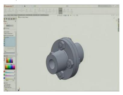
This is the assembly that we are going to make. What is this? This is a flange coupling in which we have 2 flanges and it is coupled using nut and bolt assembly.
