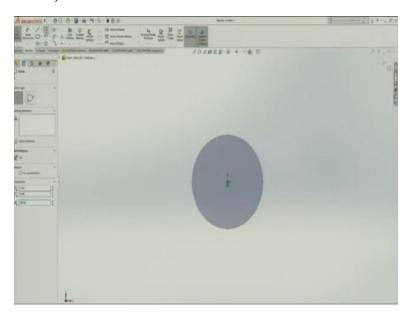
So, for making the flange first I will start form the circle, this is a circle, the radius of the circle first I will put the outer radius I will put radius as 40 because the dia is 80 millimeters here.
