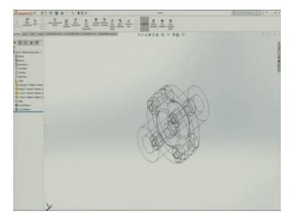
Also this is mesh, this is wireframe, wireframe is little difficult to understand, generally it is not shown. But sometime contingent requirement just to see whether what are the various internal components, internal lines, or drawings, dimensions, sometimes also shown.
