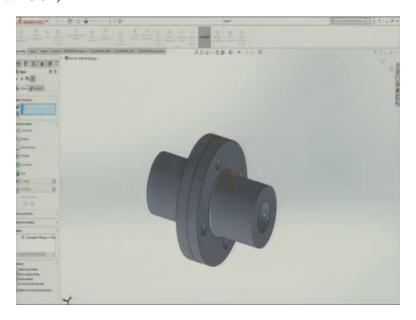
Again this phase has to be mated with this phase when I say this has to be mate, it has to come closer. So, in this case, now these are in the same direction now I have to stick the faces of the flanges, this face is the face of the other flange, I will again put mate and put select this surface is to be mated with this surface. So, the mate has happened. So, now the flange setup is ready. So, it is mated now I need to insert components again, I need to insert nut and bolt.
