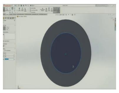
So, now this is the flange, so now I need to cut extrude here to make a hole inside it. So, we can select this and make it perpendicular we have made this phase perpendicular.
