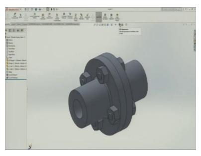
So, this is the final assembly that I need to make. In this we can see we need two flanges, four nuts and four bolts. So, to make them let me start with my assembly part. So, I have made nut, bolt and flange.
