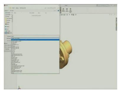
Okay let me first save it. Assembly format in the assembly format, we have the assembly format which is ASM, then we have the IGS, this is IGS, when we change one computer to other, STL is, Standard Tessellation, so this is used for 3D printing, IGES is graphical exchange format, CATIA, PRO even different softwares are there, Adobe Photoshop, JPEG images can be made.
