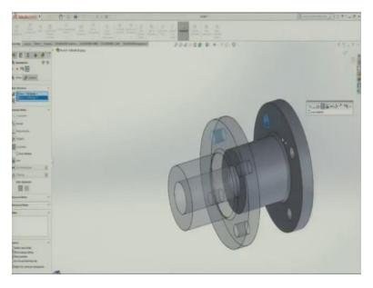
Now, these components to be mated and one of the flanges to be flipped over. So, as we know that when we have to mating the hole has to be coincided, so I will just mate the holes, so I will mate this hole with this hole. Okay this is mated again please see.
