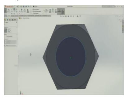
So, now this feature is almost study okay in this, this side I need to put hole now here. This hole size is 8mm dia and 4mm radius, I need to cut extrude this as well.
