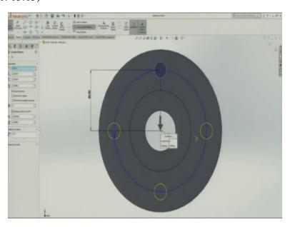
So, now we did a drill hole here for the nut and bolt system. So, nut and bolt should be perpendicular to the axis here. So, diameter for the hole is 8 mm, so before 8 mm dia I put 4mm as radius.
