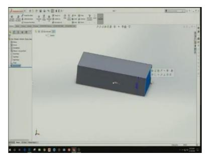
So, I have made a cut extrude for you here. And I like to just mirror this. But this is a box kind of a shape that has made. So, I will just select the whole body here. So, I will go to mirror command.
