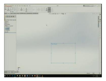
So, let me try to see the normal to the plane, normal to the tape plane. Yes, this is an important to note that how do we pan that we click the control button and then we move it, it can pan and the central scroll up and down can just make it zoom in and zoom out and by the simple left click it can show different views.
