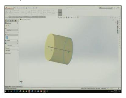
So, we can apply extrusion by either dragging this arrow, this is one ways.
