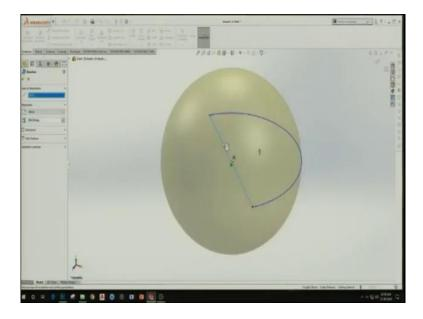
I will put this as if I just click this as exit of revolution. It has revolved it completely it, has turned into a complete ball. Why it has done so? Because there were certain options like evolve, blind evolve, up to vertex revolve, up to some surface offset from surface and so on. So, since the angle is 360 degree here, 360 degrees means it has completely evolved to 360 degree and turned into a sphere. Now, we can also revolve to maybe midplane or up to some vortex or so on.
