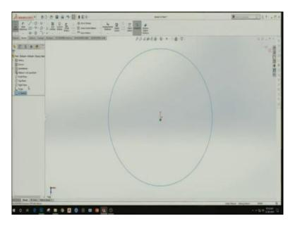
And okay and making it normal to the plane. So, I can edit this sketch, I can edit this sketch implies I can change the dimensions of the circle. So, let me change it to 40 mm now okay if I now make, like to make a different geometry, suppose if I like to make a line here.
