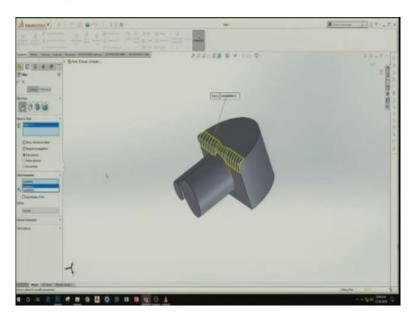
Symmetric if it is both sides like on the vertical and the horizontal side was at the 90 degree we would like to make it symmetric or is asymmetric. So, let me change this to symmetric and give it value, so 10mm seems a little big on this plus let me change to 5 mm okay this is okay somewhat okay then better. Somewhat okay then before. So, this is Fillet.
