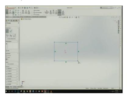
So, one point and hold and leave it here, second point. So, this is the first rectangle it is created. So, it shows all blue. So, the blue line here show that is not constant, the dimensions are not yet fixed that is we can just change the dimensions.
