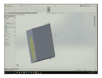
So, on the top of it will not be seen in the other way we can see that it has cut it. So, what are the kinds of the extrude cut those can be made. So, it is blind through both up to line, up to vertex, up to surface then offset from the surface and so on. Let me try to make this a blind hole of 60 mm, okay 60mm is a blind hole that is selected here. So, I will accept it.
