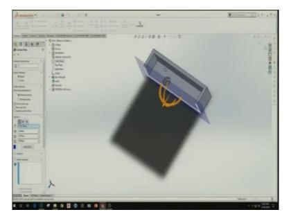
And this is Section View. Section view is the wherever we move this plane, it will just show this section of the plane. So, this is section view. So, similarly, there are different kinds of views are there. So, this is the general things those we can do in the SOLIDWORKS.
