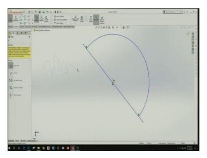
So, power trim means if I click here, I am just going free hand whenever, at where at the point if I touch anything, it just goes off. So, again this is trimmed, again this part is trimmed. So, to trim the object it will trim the sketch between any two intersections. So, by dragging the mouse we can just trim them so, accept.
