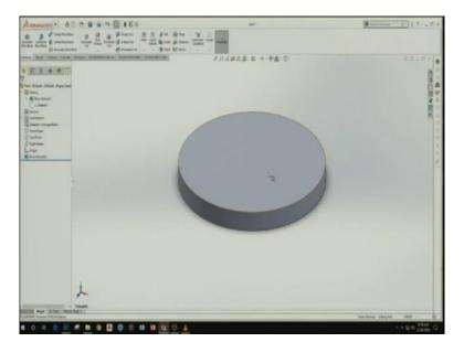
So let me put extrusion value as 20. So, it has turned to a disk now. So, this is a disk of 20 mm height and 19mm radius. So, let me try to put various pins over it. So, how does that happen?
