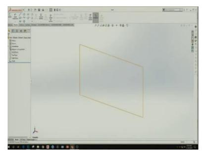
So, let me try to start from the scratch. So, we need a plane first to start, we need to decide the plane here. Then I first I have to select the plane front, top, or right plane. So, suppose if I need to draw a circle, so in which plane would I like to draw the circle? If I have to, first I have to select the plane for that.
