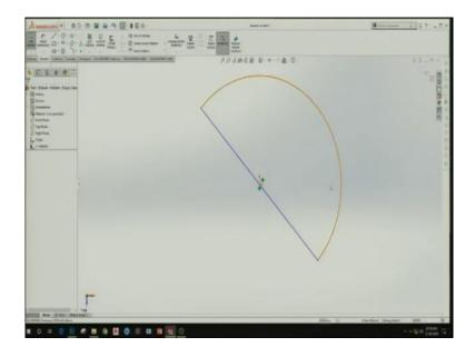
Now, we have made a semicircle, okay one of the 3D object just showed you was extrusion. Now suppose if I like to make sphere from this semicircle that is making a ball out of this how do I do?
