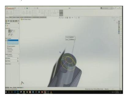
So, let me try to apply Chamfer here. So, it is showing Chamfer of distance 10mm into 45 degree. So, let me try to change this length also to 5mm. So, when I click here, so I will click right button.
