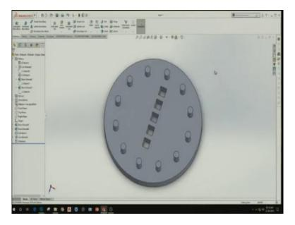
So, it has made the cut extrude here. Cut extruded pattern here or extruded cut pattern, so this is how do we use pattern command. Also yeah, one of the options is mirror option.
