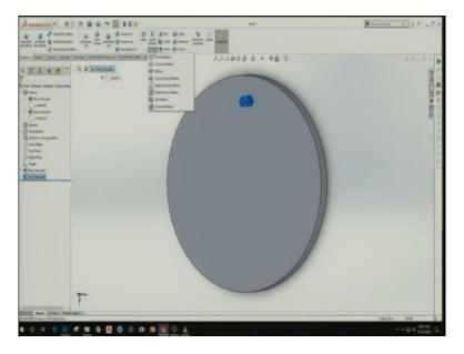
So, I will click here on the linear pattern I will select circular pattern from here it will ask instance spacing or equal spacing. So, I will put equal spacing then how many numbers do you need all along 360 degree how many number let me say, if I say 8 I put the number 8 here and it will ask me direction that clockwise or anti clockwise? It is clockwise is selected here 8 numbers symmetrically put there. So, x y z direction it is asking, okay everything is correct okay done.
