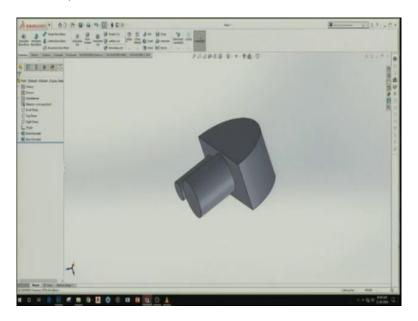
One of the things that we can do is which is very commonly used is Fillet. Okay if you click on Fillet, it will lost the edge that is filleted, so, this edge can be applied with a Fillet. So, it is asking the Fillet type coordinate variable, phase fillet, full round. So, constant size Fillet, variable size Fillet, Face Fillet and full round fillet a certain types are there and Fillet radius is given here full preview, partial preview, no preview, symmetric, and asymmetric.
