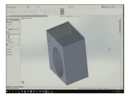
So, we are going to change the same extrusion we want to apply same extrusion here, so it is extrusion cut here, so this is already blind, blind means up to certain limit. So, let me try to change its length. Now, it is 40 mm blind through all would be obviously through all, so up to mid plane is one of the options. Okay, blind up to let me say 30. Okay, up to mid would also, would actually up to mid would be up to 25mm and a blind up to 30 mm is hole or up to 30 mm here.
