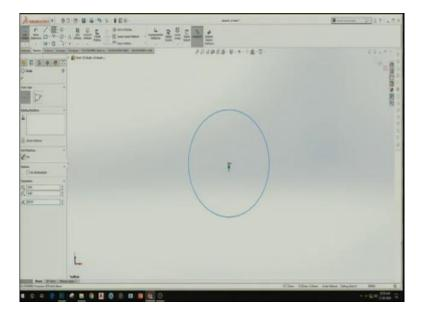
Suppose if you put 50, so, it is showing 50 here, it is not showing 50 mm radius circle. Now, what if I have to develop it 3D drawing of this circle, how to first save this? We have close dialogue here is a green tick button that is accept, accept means we save it and then exit it.
