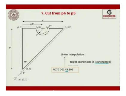
Then, from here we have to go along a straight line, so it is N70 G01. Now, I am not changing the Y value, it is only the X. I go to X9.302. So, the target value of Y is unchanged. So, it is linear interpolation. Here it was circular; counter clockwise circular, so here it is linear. So now, from here I will have to go again a linear towards the point p1.
