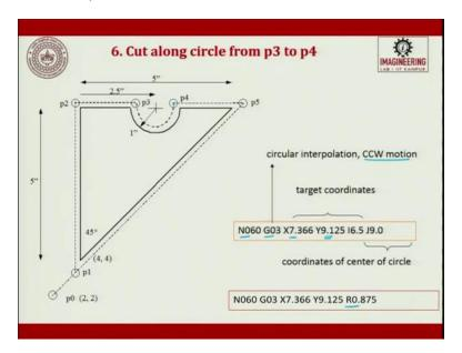
Next one is circular interpolation, counter clockwise motion. So, N60 G03. So, it is from here I have to swing it around up to here. So, it tries to tell me the point, so which is 7.366 and Y is along a straight line, 9.25. And I and J are the coordinates of the center of the circle, or you can try to define the radius of R. You can write it like this or you can write it like, N60 G03, X is the same, Y is the same. I0, you can define R0.8. Then you can go up to this point.
