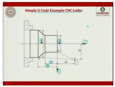
So now, let us take; this is for your milling component. Now let us see, one example for a turning component. So, a simple G code example for a CNC lathe. As I told you, in milling you will have X, Y and Z; 3 points. But in that program, we did not have any Z value, because we assume the work piece to be a plate. So, it is a constant Z. So, that is why we did not define the Z value at all.
