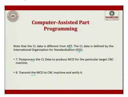
Note that the CL data is different from APT. So, CL data is defined by the International Organization of Standards (ISO). And finally, you do post processing and transmitted to the MCD.
