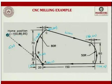
So, when we try to look at the sequence, N5 absolute position, so G90 and metric units has to be used. Then you will have; next is call for tool 1. Then define work zero at A. So, if you want to define the point at A, you can make this as (0, 0) or you can try to make this point as (0, 0). I have made offset from this point as (0, 0) and I have given these values. But, if you want to follow the sequence what is given here, you can also do that.
