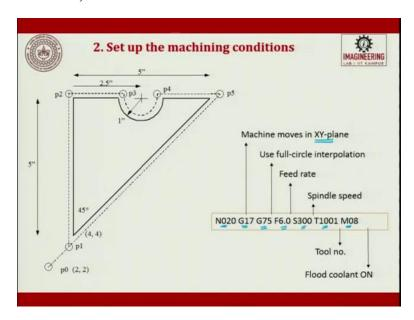
So then, N02 I am trying to move. G17 is the plane, XY plane I am going to use. And then use, full circle interpolation is G75. Then we are defining the feed, cutting speed, tool number, and finally the flood coolant on. Miscellaneous will come at the last. This is second point.
