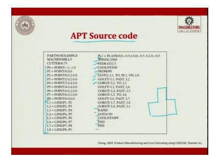
This is what we said here. So, here prime disadvantage of APT is that it uses English like command. So here, this also you should see. I told you. So, an APT post processor program is used to read these statements, interpret the meaning, and perform all the necessary calculations to generate a series of cutter location points. So, that is what is CL data file, which will be generated. So, this is the APT source code which is generated. This will be compiled and you can use it.
