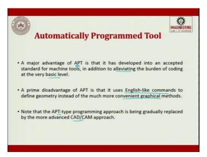
Automatically programmed tools, a major advantage of APT is that it has developed into an acceptable standards for machine tools, in addition to the alleviating the burden of coding of very basic levels. The primary disadvantage of APT is that it uses English language command to define geometry instead of convenient graphical method. Note that, APT type programming approach is being gradually replaced by more advanced CAD/CAM approaches.
