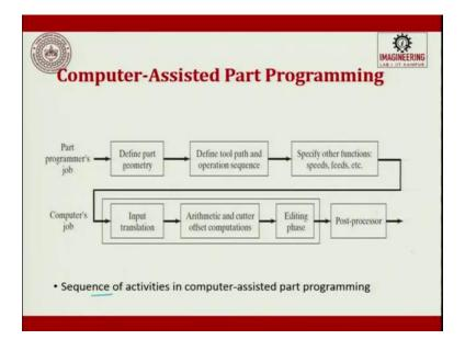
So, this is what a part programmer's job is, define path, define tool path operation, specify other functions speed, feed, etc. The computer's job will be, input translation, arithmetic and cutter offset compensation, editing phase and then it does a post processing. The
