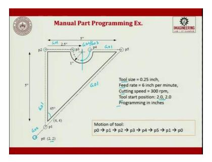
The next important topic in CNC is going to be, Manual Part Program, an Example. So, we will try to start from here, this is a component. So, we will try to start from point p0, then we go to p1. This is all in inches by the way; these are all in inches. So, we will go to p1, from p1 we will go to p2. You know the length; you know the angle which is set 45 degrees. Then from here you will try to come here offset. Then you have a radius, so the radius is divided into 2. So, this is one clockwise.
