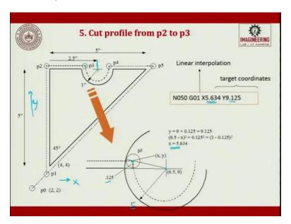
Then, from here I have to come up to here. So, this is what is N050 G01. I have to say from here it is 9.25, which is fixed. And from here, I know the diameter up to here; the length up to here is 2.5. And I have to, this radius is 1 inch. So now, I have to subtract it and find out what is p3, so p3 is a point here. So, we know the diameter is 0.25, so radius is 0.125.
