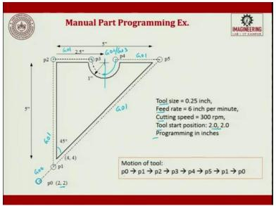
Next, from here I will try to do your linear interpolation, which will go from here N0, N40, G01. So now, from here I have to go up to here. So, what I will do is, I will try to; because this is 4 and this is 5, so this is 9 inches. So, I will have to go X3.875. I will go up to p2 destination which is 9.125. Why is this 125? because we have told the diameter of the cutter is 0.25 inches, so half of it.
