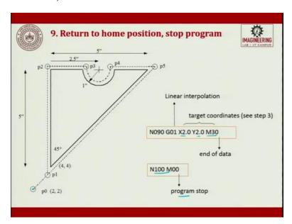
And then, from here I will try to move here. So, it is G01. So, X2 and Y2; so, I come to this point and I say end of the data. And then I say, N100 M00 stop the program. So, the complete part is executed in this program. So, we have done it in 9 steps.
