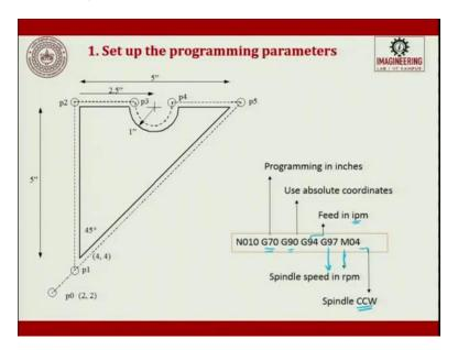
So, let us do step by step, by step. First, set up the part programming. So, first block you write, N010. So, the entire program is inches, G70. We are going to follow absolute, G90. So here it says, the feed is in inches and then we have; this in inches. Then we have spindle speed in RPM, and then we will try to have spindle on, which is in the counter clockwise direction.
