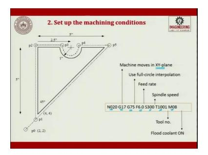
Then the third one is, we have N03. We are saying G01 X3.857 and Y is 3.698. So, this is the target coordinates, to the end point what it has to go. So now, from here it will try to go here. So, this is p1, this is p1. So, here if you look at it, so this is p1. So here, it is (4, 4), this point is (4, 4). So now, I have to go stop here. So, I have to find out the point. So, it is 4 minus 1.25 times, which is a diameter, so it is 3.85 comes here. And Y axis is this.
