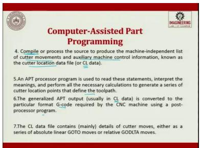
Now that we have understood manual programming, let us move to the next step called as computer assisted part programming. So, in computer assisted part programming, here it APT or Automatically Programmed Tools is high level computer programming language, most commonly used to generate instructions for numerical control machine tools.
