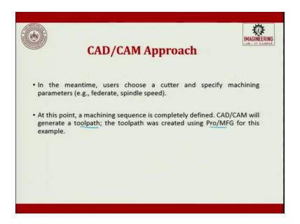
So, the next approach is going to be CAD/CAM approach. So, there will be a demonstration which will be done by Dr. Amandeep Singh, on this topic. But let us quickly go through what is covered here. The CAD/CAM approach is the most popular and advanced approach in generating CNC codes.
