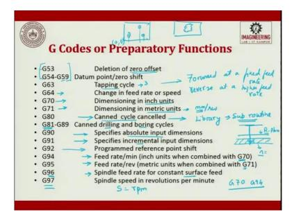
This, 70 and 71 it is an inches. So M, it is in metric. So, this is how syntax is. You can write it as N10, 70 which is in inches. Then you call it as G90, which is in absolute scale. Then 94, 97 and M04. Let us see, what is 94.
