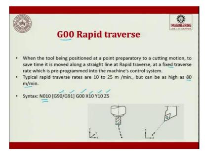
So, now whatever we have studied in rapid traverse, let us have a pictorial representation and understand. When the tool is being positioned at a point preparatory to a cutting motion to save time it is moved along a straight line at rapid traverse, at a fixed traverse rate which is preprogramed into the machine's control system. Fixed traverse is the highest feed rates, whatever it is. Typical feed rates are 10 to 20 meters per minute, but can be as high as 80 meters per minute.
