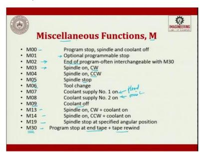
The next important topic in CNC is going to be, miscellaneous code functions. So miscellaneous codes are, these are all important from the point of your execution. G00 command are preparatory code, they will be used for simulation, dry simulation and see on the system whether the profile, whatever is cutting is to your requirement. But when we start introducing the miscellaneous codes, these codes are going to help me while manufacturing the product.
