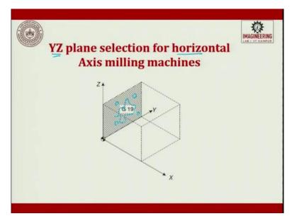
So, YZ for horizontal axis milling machine is G19. So, you see for from machine to machine, horizontal to vertical axis when you do, so you can see the planes differ. You have to define these planes, then after defining this plane in this plane, what are all the operations to be done. So, then you can ask that to do.
