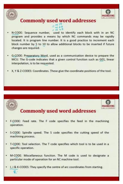
So commonly used to word addresses are, N code. So, N code is the sequence number used to identify each block with an NC program and provides a means by which NC command may be rapidly located. For example, N10, N20, N40. So, N is nothing but the line number. It is program line number. It is a good practice to increment each block number by 5 or 10.
