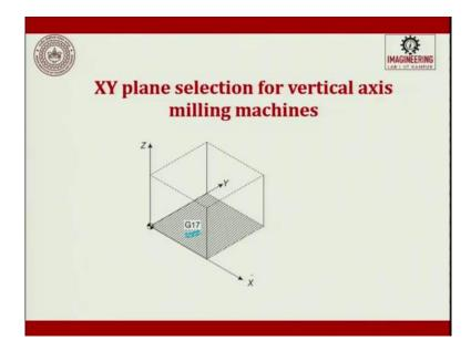
So, this is the XY plane selection, on a horizontal axis milling machine. Please see the difference. This is XY plane for vertical axis milling machines, bottom XY plane. When I do the same thing for a horizontal axis, XY plane I, this comes like this. So, this is X and Y, G17.
