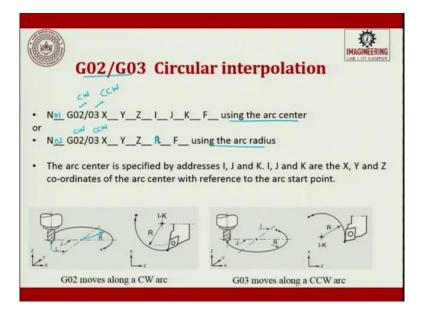
When we talk about circular interpolation, G02 or G03, it is circular interpolation. There are 2 formats. One is number block 01, so then you can choose either G02 or G03 this is circular clockwise. This is circular counter clockwise. And then X, Y, Z. Then you will have an offset in x axis, offset in y axis, offset in z axis, then you will have a feed rate. So, using the arc centre.
