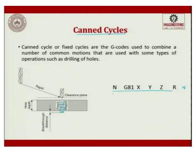
When we see a Canned cycle, a Canned cycle or a fixed cycle are G codes used to combine a number of common motions, that are used with some type of operations such as drilling of a hole. So, from here rapidly it comes to this plane and this plane is called as a clearance plane. And from here, you can keep going inside and outside. So, number of times it can peck and then do the operation.
