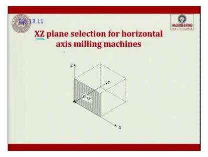
So, the XY plane for horizontal axis X is at plane, horizontal axis milling machine X and is at, so this is G18. X is at plane selection for horizontal axis milling machine.
