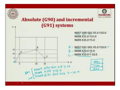
So, this is absolute and increment. I am just comparing. So, N07 is the seventh line of that particular program. You have called G90, which is absolute and then you said G01 moved to this point A, which is X5 and Y10. So, the next point is going to be, if you are, if I am going to move here, it is going to be next to G, N. So, to have a safer role it will be N008, G90 then you will say G01, X25, Y15.
