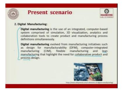
When we talk about digital manufacturing, it is the use of an integrated computer based system comprised of simulation, 3D visualization, analytics, and collaboration tools to create products and manufacturing process definitions simultaneously. Digital manufacturing evolved from manufacturing initiatives such as design for manufacturability, computer aided manufacturing, flexible manufacturing, lean manufacturing that highlights the need for collaborative products and process design.
