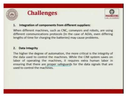
So, the integration of components from different suppliers when different machines such as CNC, conveyers, robos are using different communication protocols, this might cost a lot of problem for integration. Next, data integrity the higher the degree of automation more critical is the integrity of the data used to control the machines. While the CIM system saves on labor of operating the machine, it requires extra human labor in ensuring that there are proper
