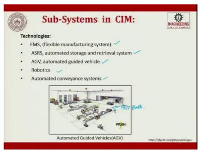
The technologies which are used under CIMs are going to be FMS, ASRS. ASRS is nothing but automatic storage and retrieval system, then you will have AGVs. AGVs are automatic guided vehicle, these are AGVs what is moving here. This is an AGV then you also have robots which keeps moving. So, this is AGV path and you have robots, you have CNC machines and you also have automated conveyer systems.
