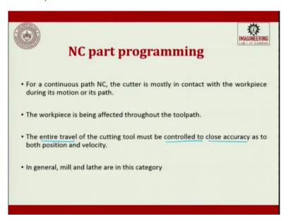
For a continuous NC machine, the cutter is mostly in contact with the workpiece during the motion. The workpiece is being affected throughout the toolpath, the entire travel of the cutting tool must be controlled to close accuracy as to both position and velocity. And in general, milling and lathe machines falls in this category.
