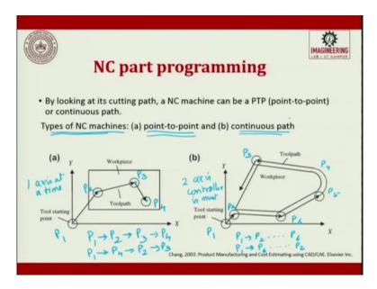
There are 2 types of NC machine programming, one is called as point-to-point, the other one is called us continuous. In point-to-point programming, we are only worried about the starting point and the ending point, we are least bothered the path it which it traces towards the output. For example, let us take this as P1, P2, P3, P4. So here it is said as, P1 go to P2, then go to P3, then go to P4.
