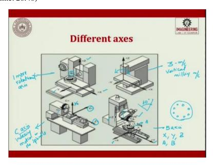
So you can see, different axes I have put. So, this is a 3 axes machine which is vertical milling machine. So here, it is the same vertical milling machine, but I have an axis more one is, I have
