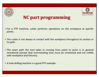
For a point-to-point machine, the cutter performs operations on the workpiece at a specific point. The cutter is not always in contact with the workpiece throughout its motion or its path. The exact path the tool takes in moving from point-to-point is in general immaterial. This is what we explained and I have also told you, what is the hardware involved behind. Hold drilling operation machine, is a good example for point-to-point.
