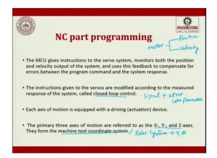
The MCU gives the instruction to the server system, monitors both the position and the velocity of a system. I told you as far as motor is concerned, you have only 2 things to monitor, one is the position, the other one is the velocity, with which you can try to control the movement of the tool or the work piece. So, monitor both the position and the velocity output of the system and uses its feedback to compensate for error between the program command and the system response.
