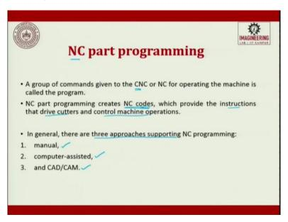
When we talk about NC part programming, a group of commands given to a CNC or a NC for operating the machine is called a program. So, here you write program using alphabets, numerical, that is alphanumerical and you try to control the complete machine. The logic what is used here, the hardware what is used here in a CNC machine, is the same which we will use it for rapid prototyping also.
