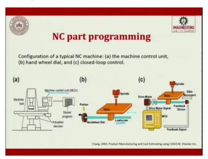
So, you can see schematic diagrams. So, here you can see a configuration of NC machine. So, you see an MCU, this is an MCU, though it looks like a monitor, behind that it has so many processing units. So, that does the MCU job and this is the typical machine. So, these are the actuation drives, and here is a storage device, it can be a pen drive or a USB or it can be a floppy disk, it can be a hard disk. So, so many things can be a storage program device.
