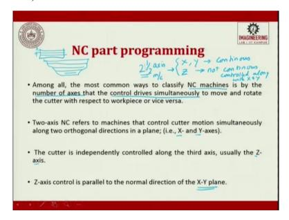
Among all, the most common way of classifying NC machine, is by the number of axes that the control drives simultaneously to move and rotate the cutter with respect to work piece or vice versa. So here, we are now defining the NC machine, number of axes simultaneous control. Now, we are going into continuous simultaneous control. So, there are possibilities where X
