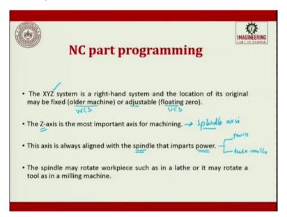
The XYZ system is a right hand system, and the location of its origin may be fixed or adjustable. So, this is what I said world coordinate system or user coordinate system. So, we call here in CNC as old machines, that is a fixed one or we call it as adjustable which is floating 0. The Z axis is the most important axis of the machine, where it becomes the spindle axis.
