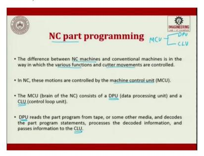
So, when we look at the NC part programming, the difference between NC machine and the conventional machine is the way in which the various functions and the cutter movements are controlled, this is the only difference. In NC machines these motions are controlled by MCU. MCU is nothing but the brain of a NC machine which consists of 2 things, one is called as data processing unit, the other one is control loop unit.
