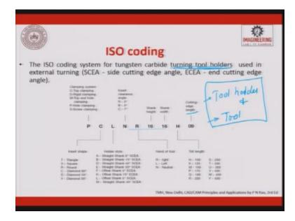
So ISO system for tungsten carbide turning tool holder, that was for the tool and here we are talking about the tool holder used in external turning. So you will have the similar digits which are followed. So you will have P where which talks about the clamping system, top clamping, rigid clamping, top and hole and then you have screw type.
