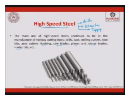
So high speed steels are used for drills and which is used for broaches. Broaching is an operation wherein which the geometry is very complex. You can also use it for tapping where the thread geometry is complex. Wherever there is an impact load and there is a complex geometry, we prefer to go use HSS.
