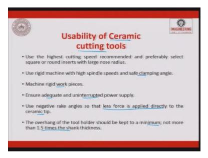
So the usability of ceramic cutting tools, use of highest cutting speed recommended and preferably select square or round inserts with large nose radius are always preferred in the ceramic cutting tool. Use rigid machines with high spindle speeds and safe clamping angles.
