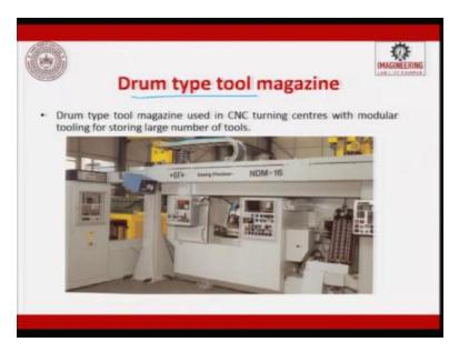
So you can have a drum type tool magazine. These are drum type tool magazines okay. So drum type, which is used in CNC machines.
