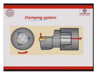
So the clamping system you can have a clamping system like this. So here you can see these, this is used for machining. And here you have made some small grooves, so these grooves are used for clamping it.
