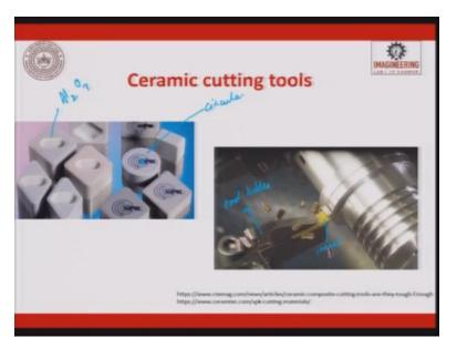
So these are some of the ceramic inserts. These are all alumina, so this is all square or cuboidal. This is all circular. So circular, the advantage is it has infinite cutting edges. And you can help self-rotating, self-propelling inserts and you can also have inserts with clamp. So this is a turning operation done. Here is an insert, so the insert height and all you have to calibrate it and keep and this is a tool holder.
