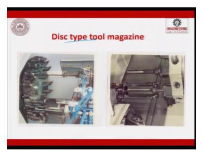
So a disc type tool magazine. This is a tool magazine which is disc type and this is how does it change is given here.
