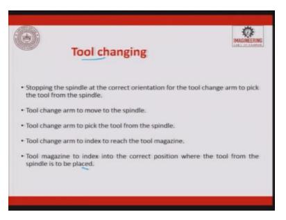
Tool changing, stopping the spindle at the correct orientation to, for the tool change arm to pick up the tool from the spindle. These are the steps which are involved. Tool change arm to move to the spindle, then the tool change arm to pick the tool from the spindle, the tool change arm to index to reach from the tool magazine to reach there.
