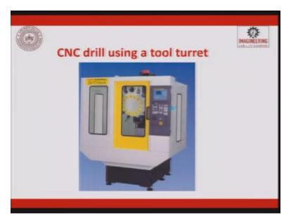
A CNC drilling used in a tool turret, this is what is a tool turret which is used. So for drilling operation, this is a CNC machine. This is an interface where you can write program, you can see simulations here.
