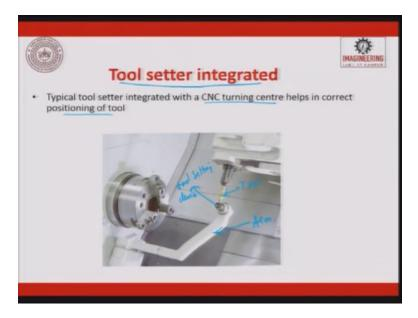
So today we also have tool setter integrated into a CNC machines. So you have a knob which is attached. This is a tool and this is an arm which is attached and here is a tool setting device, which gives you the measurements. So if you want to check the height of the tool, diameter of the tool, you can check it and accordingly this will be entered into the register.
