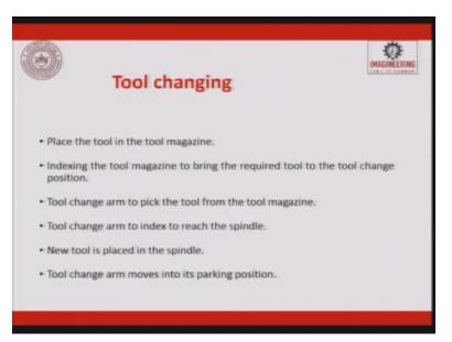
Place the tool in the tool magazine. Indexing the tool magazine to bring the required tool to the tool changing position. Tool changing arm to pick the tool from the tool magazine. The tool changing arm to index to reach to the spindle. A new tool is placed in the spindle. The tool changing arm moved into the parking position.
