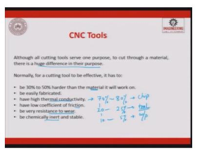
Although all the cutting tools serve one purpose to cut through a material, there is huge difference in those purpose. So some places, if there is a lot of variation in the tool in the work-piece material, so then the tool has to have enough of toughness. If it is a complex job machining, the tool should give us the flexibility of regrinding.
