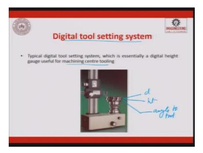
So while inserting the tool, insert inside a tool holder, it is not so easy. There are so many angles which are to be maintained apart from the height and the diameter. So when we use this CNC machines, in the CNC machines itself you will always have a digital tool setting
