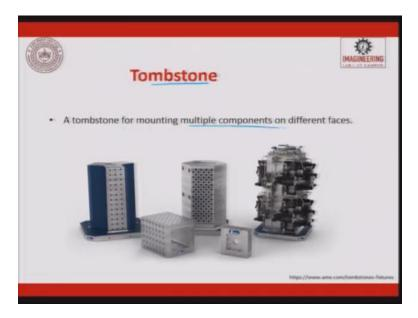
And you can also have a tombstone wherein which this is used to be mounted on top of a table, so different faces can be used for machining.
