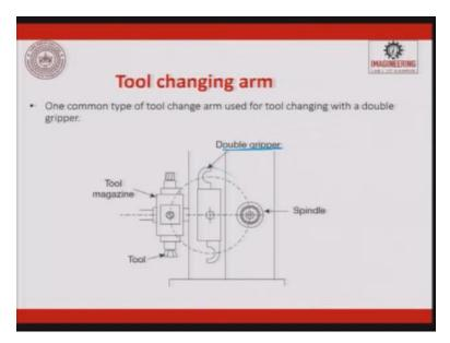
So this is what is the double gripper attached to an ATC, automatic tool changer. Tool here, tool magazine here and then this is the spindle where this comes and removes this and puts it back into the magazine.
