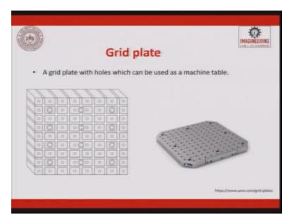
So these are the grid plates which I have already discussed in the palettes. So grid plates with holes which can be used as a machine table which we discussed in automatic tool changer.
