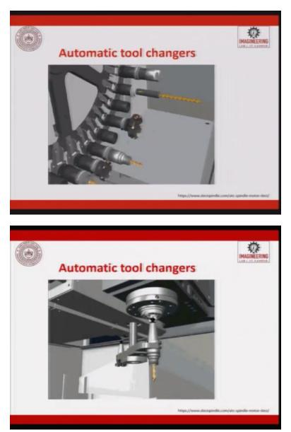
So you can see here automatic tool changer, this is the automatic tool changer, ATC. So a tool which is now removed, removed from it, removed from the spindle. This is mounted and this is put back into the system and this starts doing it. So this is an automatic tool changer.
