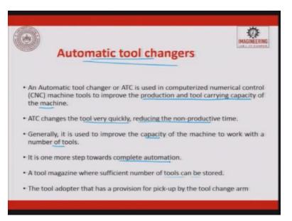
So now we have seen about the tool material and then tool holder modularity. Now let us see a very important thing which is called as automatic tool changer. So like we saw automatic pallet changer for improving the productivity, we will also see here automatic tool changers. This is to change the tool from one to the other, such that in a single setting you can do multiple machining operation.
