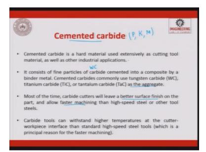
The next one is cemented carbide. There are several types of cemented carbide P type, K type, M type so many different types are there. The cemented carbide is a harder material, uses extensively as a cutting tool material as well as the other industrial applications. It consists of fine particles of carbide cemented, so it is, carbide is nothing but tungsten carbide cemented into a composite by a binding material.
