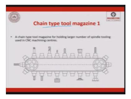
So there is a chain type tool magazine. You can have more number of tools, so you will have something like a chain type. A chain type tool magazine for holding large number of spindle tools used in a CNC machines.
