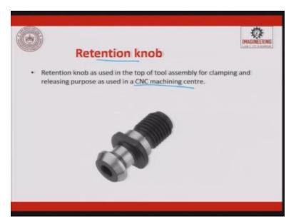
So this is the retention knob. It looks like this. The retention knob as used in the tool of tool assembly for clamping and releasing purpose as used in a CNC machining centre. This is a retention knob.
