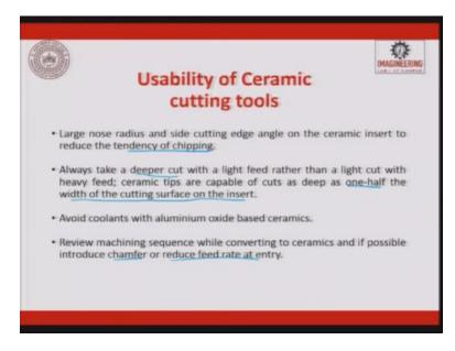
Large nose radius and side cutting edge angle on a ceramic insert reduces the tendency of chipping. This chipping because ceramic when the toughness is poor, so if a crack gets initiated, next immediate thing what happens is the chipping of the cutting tool. So that is removed.
