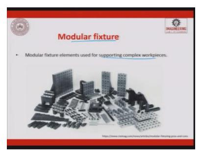
So today we talk about modular fixtures. These are all the components of a modular fixtures. So all these things are used to develop a fixture and support a complex workpiece. So this makes the CNC machine versatile to hold any type of shape or geometry.
