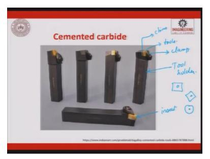
If you look at these, these are some of the cemented carbide tools. In HSS, the entire tool will be made out of HSS. When we come to cemented carbide tools, we will have a tool holder and then these are the tools. These tools are held by a clamp. The height are adjusted by chims or height adjuster.
