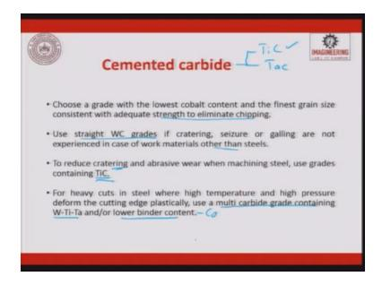
Choose a grade with the lowest cobalt content and the finest grain size consist with adequate strength to eliminate chipping. Use straight tungsten carbide grade if cratering, seizure or galling are not experienced in the case of work-piece material other than steel. So use straight tungsten carbide grade.
