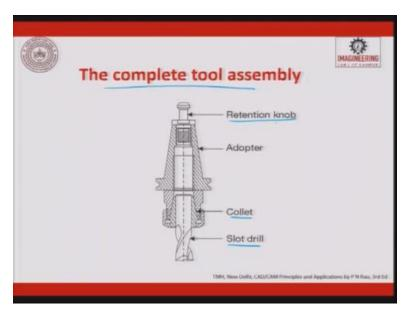
When we look at a complete tool assembly for a milling cutter, you will see or a slot drill, so this is a slot drill. This is fixed inside a collet. This collet has an adapter, this is an adapter, this is a collet. So this is a collet. This collet is spring-loaded. So you can press fit it and then get it removed.
