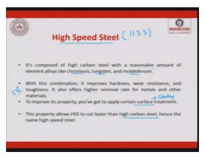
When we talk about high speed steel, the high speed name came from the ancient time, so we still keep continuing the same. So this is high speed steel. It is composed of high carbon steel with a reasonable amount of elements like chromium, tungsten and molybdenum. So they give the hardness and the cobalt which is present there gives you the toughness.
