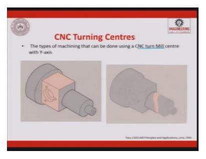
So if you want to do a typical job like this, a hole to be done and then you will have a cube to be machined and then drill and then along inside you want to have a tab which can be done. So all these things can be done in this turn mill centre with Y-axis this way and then if you want to make a groove, it can also be done.
