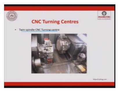
So this is how a twin turret looks like. So this is one turret, two turret and here is the lathe machine, this is a spindle wherein which you will load the work-piece.
