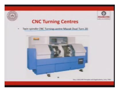
So this is how a twin spindle CNC turning centre looks like, a twin spindle CNC. Two spindles are there. You have multi-spindle automats today. So you will have 6 spindles are there. These are basically an SPM machines. You would have never even thought about 2 spindles.
