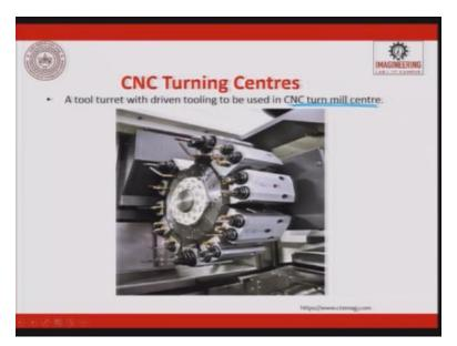
So where we will have tool turning with driven tools to be used in a turn mill centre. So you can have so many tools which are attached and then this in turn will be doing turning operation as well as a milling operations.
