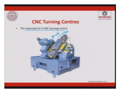
So this is the slant bed CNC turning centre which I have already discussed. So here you will have the spindle which rotates and here you will have the tool which rests.
