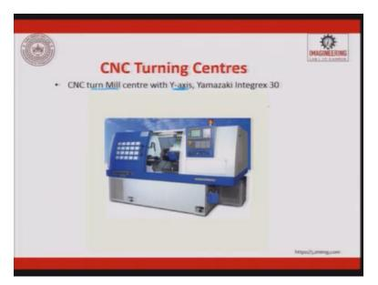
So you can have CNC turning milling centre with Y-axis. Y-axis, why is it specified? Because in a lathe machine you will always have X and Z-axis only.
