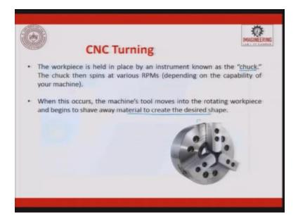
The work-piece is held in place by an instrument called as the chuck. So when we try to do a manual lathe machine, we will have a chuck wherein which there will be a nut here, you put a counter of the nut here, a tool, and then we try to move. So when we try to move one nut, there will be internally threads which are helical at a plate. So now every job will be moving uniformly.
