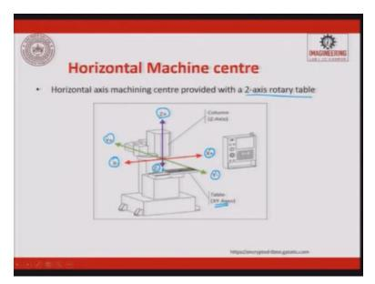
So horizontal machining centre provided with 2-axis rotating table. So this 2-axis rotating table you can have. So here what we have defined is, we have defined the axes, so it will have Z, which is tool when it moves away from the work-piece it is positive, towards the work-piece it is negative and depending upon this as zero, you will have a negative X and a positive X, positive Y and a negative Y.
