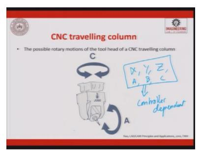
So the travelling column, the possible rotary motions of a tool head of a CNC travelling machines are, this is C and this is A axis. So this is C axis, this is A axis, so X, Y, Z you can also have A, B and C. So I said gamma and theta that depends on the controller. So please check these characters are controller dependent.
