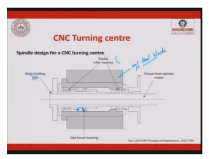
When we talk about the spindle design for a CNC turning centre, so the spindles nowadays are expected to rotate at 100000 RPM. So you see that this is the work-holding end and this is the power from the motor is given here. This is the work-holding end, this is the power getting transferred. Since it is rotating at 100000 RPM, you need lubrication on top of these bearings.
