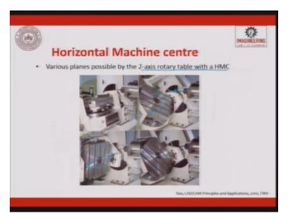
So these are the various planes by the 2-axis rotating table in a HMC. You can see here this is a table, HMC is horizontal machining centre. You can see the table can be swiveled and you can bring it like this, you can take it to an angle, you can bring like this. Here is a tool, but now you buy just controlling that table movement, you can try to have a complex component machine.
