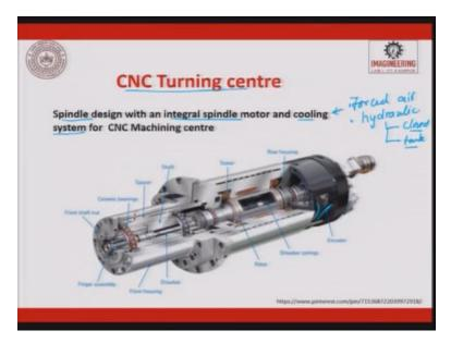
Okay and you see here, this is the latest CNC turning centre spindle. So the spindle design is an integral part of spindle motor and cooling system. When we start rotating at 100000 RPM, you should see that there will be a huge heat which is generated between the stationary part and the moving part. So you need to have a cooling system. It can be forced air or it can be hydraulics.
