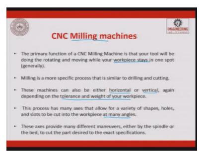
The primary function of a CNC milling machine is that tool will be rotating and moving while your work-piece stays in one spot. That is what I said, machining centre, work-piece stay. Milling is a more specific process that is similar to drilling and cutting. These machines can also be either horizontal or vertical again depending on the tolerance and weight you decide to go for a horizontal machine or for a vertical machine.
