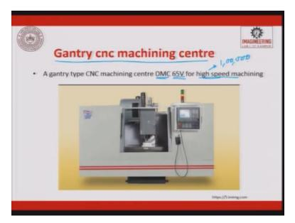
So the other one is gantry type CNC machine. So here I have just shown you a DMC 65V. So DMC 65V is a machine, so which is used for a very high speed machining centre. Here the speeds what we talk about is 100000, okay.
