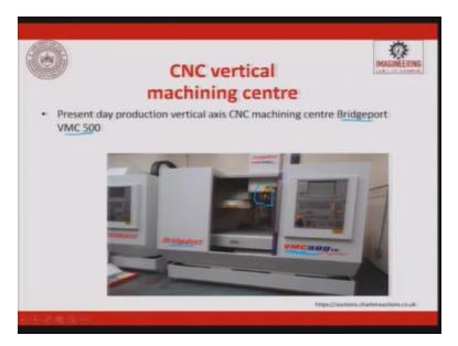
So, CNC vertical machining centre, this is the vertical machining centre. Present days production vertical axis CNC machining centres use Bridgeport VMC 500. This is the machine, the Bridgeport is a machine name, VMC, vertical machining centre 500, 500 can be the capacity or the volume of the work-piece which you can mount.
