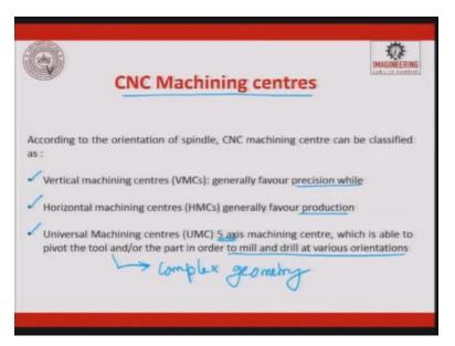
When we talk about the machining centre, according to the orientation of the spindle, CNC machining centre can be classified as vertical machining centre, horizontal machining centre and we also talk about universal machining centre. Vertical machining centres they generally favor precision, while horizontal machining centre generally favors production.
