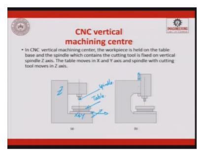
So these are typical vertical machining centres. We are just showing how are these spindles getting supported to the base machine. In CNC vertical machining centre, the work-piece is held on a table. This is a table okay and the spindle which contains the cutting tool, this is the spindle, which contains the cutting tool is fixed on the vertical spindle axis, Z.
