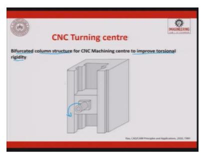
So this spindle is attached to a column okay. So now there are several modifications which are happening in the column in order to maintain a high damping coefficient and reducing the vibration transfer. So you can see here bifurcated column structure for CNC machine centres are used in order to improve their torsional rigidity, because this fellow when it rotates, there is a torsional load which is coming up when it starts milling.
