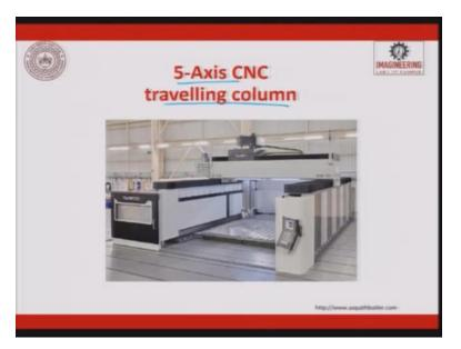
So here also you can make 5-axis, it is almost equal to 5-axis machine. This is how a typical 5-axis CNC travelling column, CNC machine looks like, machining centre looks like. You can see that complete component, a large heavy component can be there and it is directly mounted on the floor. So you do not have to worry the weight resting on the table. The table is also on the floor.
