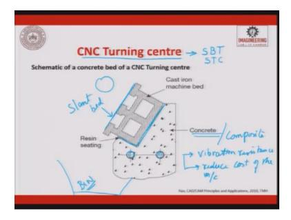
So when we talk about the CNC turning centre, we can see the latest development in turning centres in order to remove the vibration which is getting induced in the lathe bed, so they
