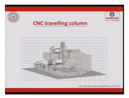
So this is a CNC travelling column. When we have a large work-piece, we used to have, we used to use a travelling column. For example, when we are trying to machine a wing of a plane, when we are trying to do a large aerospace component, if you are trying to machine a wind blade, blade of a wind turbine, windmill, so then we use this CNC travelling. Big turbine blades which are for used by the marines, or by ships, are machined by CNC travelling column.
