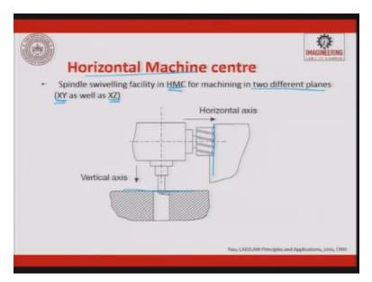
So horizontal machining centre and vertical machining which we can have a combination. So here you can see here a spindle swiveling facility in HMC, horizontal machining centre, for machining in 2 different planes it does on a horizontal plane, it does on a vertical plane. So it does on XY and XZ. Now you should understand, when we try to write programs for CNC in a machining centre, there is something called as plane definition very important.
