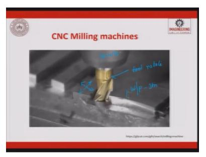
So this is how is milling. So you see here work-piece is stationary, tool rotates, tool can be given the feed rate so it can move both in this action and this action. Again, here the spindle, which is here, which is used to hold the tool can be operated either hydraulically or pneumatically.
