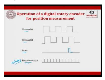
When you look at the positions of the digital rotary encoder, channel A, channel B and it tries to say an index where there is a difference and that is index is given as a pulse here. So, these are the encoder output, these are the index, index are nothing but a shift between the two comparison whatever it is and then it tries to say where there is a shift, it tries to say that is index.
