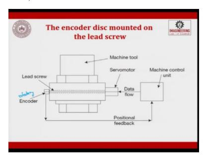
The encoders disc mounted in a lead screw, this is encoder this is a rotary encoder, and this is a machine tool we have seen enough of servo, data feed, machine tool, position feedback is given from the encoder, the velocity is given by the tacho generator.
