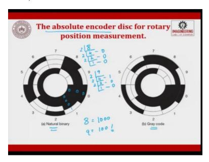
So, the absolute encoder discs for rotary position devices, this is natural binary and this is gray. So, when you have a number and then you want to convert it into binary so what we do is we divide it by 2 we say 4, 0, 2, 2, 0 and 1, 0. So, if you have a digit 8 so it is nothing but 1 0 0 0 so if you want to go to 9, this 4, 2 then you have 1 here, then you have 2, so if you have 9, it is 1 0 0 1 okay.
