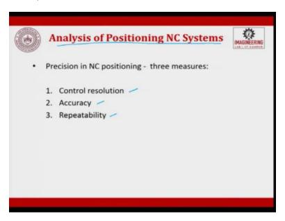
The last part of the discussion is going to be on the analysis of positioning of NC machine so the precision in the NC machine positioning there are three measures you can have control resolution, you have accuracy, and you will have repeatability. So, three things are very important when we have to measure about the position in a CNC machine or in a NC machine.
