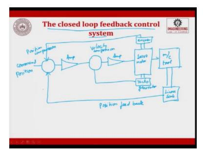
The closed loop feedback system, so the closed loop feedback control system, which we can draw a schematic diagram and see, you will have a command for position, command for position, this
