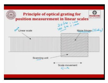
When we talk about a linear screw the principle of a linear screw works on this moire fringe pattern. Moire fringe pattern you have a linear scale and then you have a nut. So, the nut whatever it is or a sliding scale, this is a main scale and this is a sliding scale.
