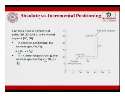
So, these are the examples for absolute and incremental, so absolute is you are trying the work head is present at point 20 comma 20 is moved to the point 40 comma 50, in absolute case you will write it as X 40 and Y 50 in absolute scale because it all happens with respect to the 0. In incremental form what you will do is, you will represent X equal to 20 and Y equal to 30, because it takes with respect to the previous point.
