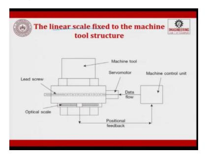
And the linear scale when it is fixed to a machine, it is fixed along here and here is a sliding scale, the position is taken and it is given to the machine tool, this is how a linear scale is attached to a machine tool to get the output.
