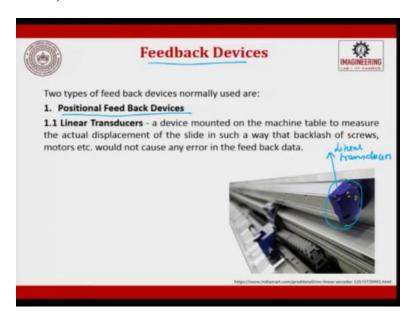
Feedback devices, so when we started CNC we saw there are 5 sections, so in that we saw motors, we saw drives and then now we have come to the last which is nothing but the feedback device. There are two types of feedback devices, one is called as the positional feedback device, the other one is called as a velocity feedback device.
