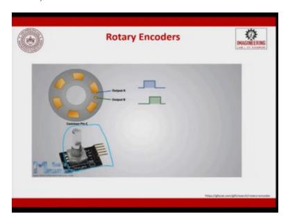
So, in animation, you can see here there are two outputs when the, when the light falls you can see A getting activated, then output B is getting activated entry and then accept. So, you can see at both the things very clearly, so it enters so this is an output which is taken and it is fed to a system where in which it is processed. So, in reality it looks like, in reality it looks like this.
