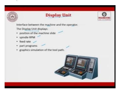
The display units are going to be it will try to display position, spindle speed, feed rates, part program, and graphical simulation. So, all these things will be done in the interface between the man and the machine. So, you can see the position of the machine tool, you can see the speed with which it is operating, feed rate moving, part program run based on the part program simulation.
