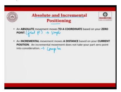
The last part is about absolute and incremental part, absolute and incremental position. An absolute movement moves to a coordinate based on your zero point, for a fixed point, for a zero point is called as absolute. An incremental motion moves a distance based on your current position, an incremental movement does not take your part zero point into consideration.
