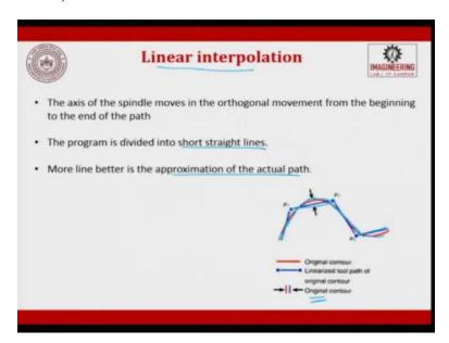
What happens in linear? The axis of a spindle moves in the orthogonal movement from the beginning to the end of the path, it moves only orthogonal. So, if you want a point like this you will try to move, if you want a curve like this you will try to move in points like this. The original contour what you wanted and the linearized machine moment, why?
