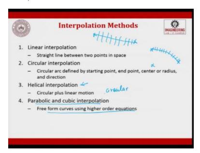
We will see about the interpolation methods, so when we talk about interpolation I told you linear interpolation, we will have circular interpolation, we have helical interpolation for complex jobs we have parabolic and cubic interpolation. Linear interpolation is start point, endpoint, between these two points discretizing several points is linear interpolation. Straight line between two points and space linear interpolation, shortest distance between two points.
