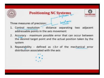
What is control resolution? The control resolution is nothing but distance separating two adjacent addressable points in the axis movement is controlled resolution, it is otherwise called as just
