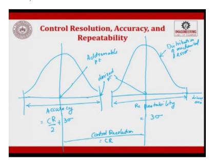
If we wanted to represent it in a figure form let me do it, these two are called as addressable points this is called as the accuracy, which is nothing but CR by 2 plus 3 sigma. So, this is the repeatability, which is equal to another 3 sigma, this we are moving it in a linear access you can also have on a rotating access so here is the desired point.
