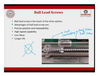
So, this is how a ball screw mechanism looks like, so you will, this is which is nut and this is the lead screw or which is other, or ball screw, the nut is otherwise called as recirculating nut. So,
