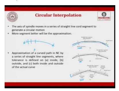
Next when we look at circular interpolation, it is almost the same, the axis of spindle movement in a series of straight line cords segments to generate a circular path. So, this is the original you want, the arc which you want and this is how the linearized motion happens, the distance between these two is called as the tolerance, inside tolerance.
