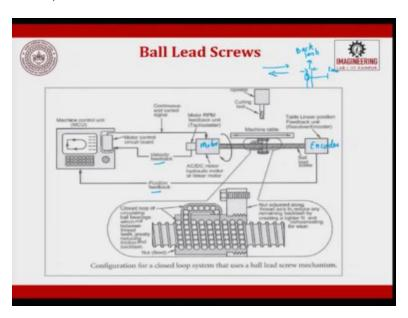
If you look into the schematic diagram, this is how it is. So, you will have a motor which is attached to a ball screw, which we saw recirculating balls screw mechanisms, today it is available in a very-very economical price up to 30 centimeter 1 foot. It is very economical available, the resolutions are very high today.
