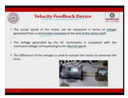
The last one is the velocity feedback drive. The actual speed of a motor can be measured in terms of voltage generation from a tachometer. So, this is a motor, this is a tachometer it tries to generate a voltage signal and that from the tachometer is taken as output and again attached.
