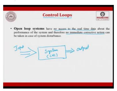
So, let us talk about the control loop, open loop system have no access to the real time data about the performance of the system and therefore no immediate corrective action can be taken in the case of the system disturbance. So, what happens here? You will have an input, you will have a system here, a system is a CNC machine here then you will have an output.
