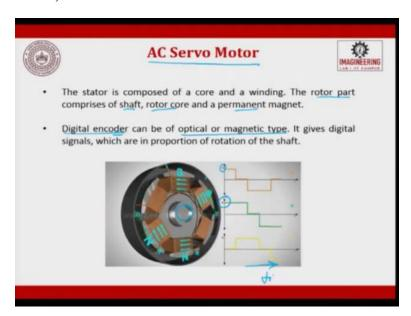
So, this is the animation for AC servomotor, the stator is composed of a core right, stator is composed of a core and a winding. The rotor parts comprises of shaft, torque, rotor core and a permanent magnet, the rotor part comprises of a shaft, rotor core and a permanent magnet.
