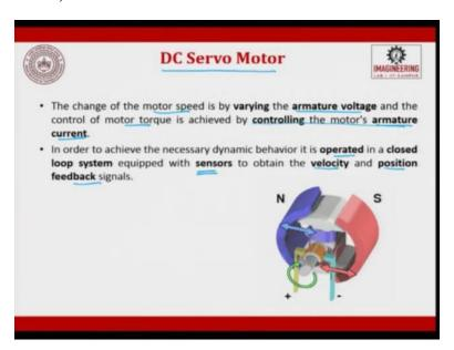
So, this is how is the simulation, or the animation sorry it is the animation of how does a DC servomotor work. The change of the motor speed is by varying the armature voltage and the control of motor torque is achieved by controlling the motor armature current. So, the change of motor speed is by varying the voltage and the motor torque is achieved by changing the armature current.
