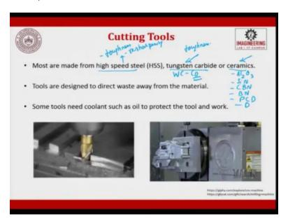
When we talk about cutting tools, as I told you earlier also, cutting tools are different from machine tools, we have never talked about the cutting tools, the cutting tools are tools where they are harder than the work piece and they have the geometry which gets superimposed to the work piece to generate a profile.
