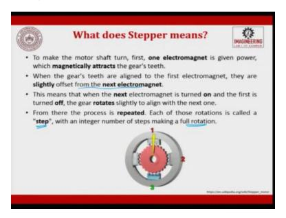
How does a stepper motor work? So to make the motor shaft turn, first, one electromagnet is given power which magnetically attracts the gear teeth. So, you can see the animation here, when the gears teeth are aligned to the first electromagnet, they are slightly offset from the next electromagnet.
