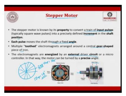
Now, the last motor we will see is the stepper motor, the stepper motor is known by its property to convert a train of input pulses, square pulses, into a precisely define incremental in the shaft position. So, what it does is? You have a 1 RPM, now you divide that 1 RPM into several small segments and these segments are called as steps.
