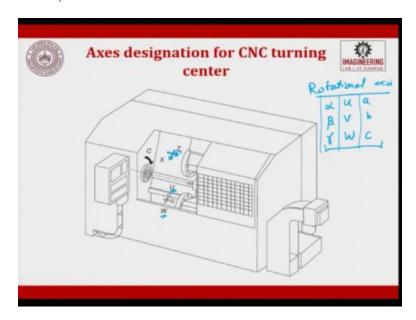
When we move towards a turning center, a lathe machine you will try to have, see you will try to have I told you two axes, X which is the depth and Z along the feed, X and Z will be the two directions, you will give and rotation about Z is the C axis and rotation about X is the U axis, rotation about Z is a W axis.
