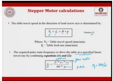
So, the stepper motor calculations, the total number of pulses required to achieve a specified X position increment is calculated by,
