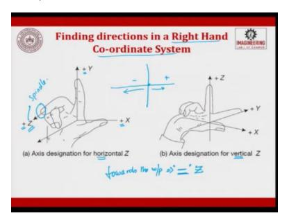
Now, let us get into little bit of how are these axis is fixed in a CNC machine. So, they follow right hand co-ordinate system, so right hand co-ordinate system is followed and you make sure that the perpendicular to the plane will always be Z and this Z will be focused towards the spindle. So, the perpendicular to the plane will be focused towards the spindle so now you can easily fix the X and Y.
