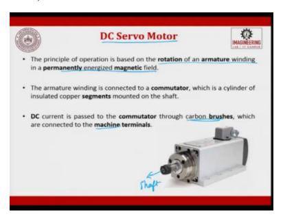
So, this is how a typical DC servomotor rotates, or looks like, the principle of operation is based on rotation of an armature winding in a permanently energized magnetic field, please understand the principle of operation is based on the rotation of an armature winding in a permanently energized magnetic field DC motor. So, that is what is a DC servomotor works.
