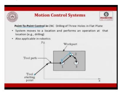
Now, let us see the next one is point to point control system based on that. As I told you the tool, the drill will come here, do the first drilling operation it will go to 2, it will do the operation, it will come to 3 and drill the operation, in between what path it takes does not matter for us. So, it will start here, and then it will accelerate till here, it will stop here.
