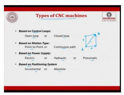
When we talk about different types of CNC machines, they are classified into 4 types based upon the controller loop, when we talk about the control loop there are 2 types, one is called as a open loop system, the other one is called as a closed loop system. If we do not get a feedback on our system, then that is called as open loop system, when we get a feedback from the machine tool to the MCU we process that data it is called as closed loop.
