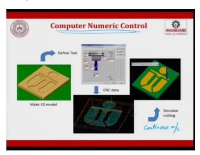
So, when we use a CNC machine what will happen is, you want to make a mold so then you make, you want to make a mold so the tool is define the tool, we define all the length, diameter, flute length, everything and then this data is given to a CNC and here you see that there are so many simulations, the cutter path is done and then finally after the simulation you will try to generate this part.
