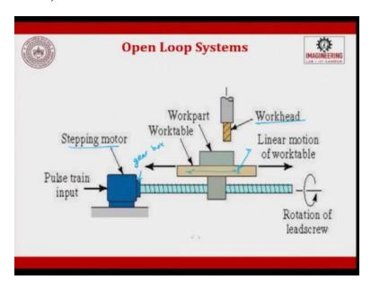
So, when we will look at the figure for a open loop system, you will see that there is a motor which I have already explained to you it is a stepper motor or a stepping motor, this is attached. So, you will have a gearbox here, or you can directly couple also gearbox, this is attached to a lead screw. So, this motor rotates the lead screw, this when it rotates it moves the table.
