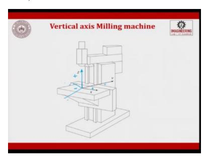
So, for a vertical milling machine so you will see this is your spindle axis, suppose you want, okay this is your spindle axis, so spindle axis I have said plus and this is minus, assuming towards the work piece, away from the work piece. Now, if you try to fix this as an origin so when you move this side it is minus and this side it is plus and it is plus here and minus this side, for Y axis. So, by this way you will be able to fix the axes vertical CNC machine.
