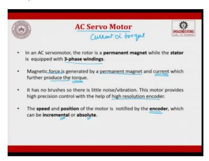
So, let us see next the AC servomotor, in a AC servomotor, the rotor is a permanent magnet, same like AC and DC motor. So, I am just talking about AC servomotor, the rotor is a permanent magnet, which the stator is equipped with the three phase winding. The magnetic force is generated by a permanent magnet and the current which further produces the torque.
