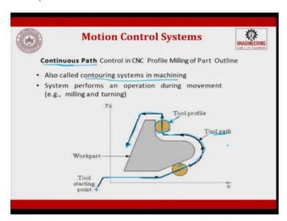
When we talk about continuous path system, so in continuous path system, the control in CNC profile milling of the part geometry. So, it is very clearly said that if you want to machine the part, the cutter has to start from here, go along this line then make the stepper, then take a radius, then go along this line, make a straight line and then come back.
