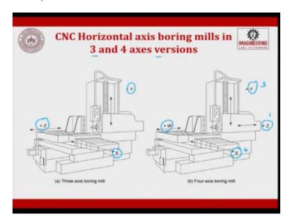
So, the CNC horizontal axis boring mill in 3 and 4 axis version so this is the boring mill, so this is the spindle axis first you fix Z, then you will fix up X, then you will fix up Y, when we try to make a rotation, a rotation axis first in a 4 Axis. What will happen? This is the spindle axis you will fix first, then you will go second, then you will fix the third and rotation I said u, v, w. So, about Z axis whatever rotation happens is W axis.
