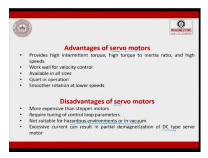
So, an advantages of servomotor is it provides high intermittent torque, high torque to inertia ratio and high speeds. So, that is why servomotors are more used, works very well for velocity control,
