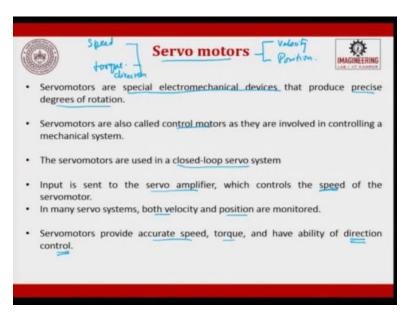
So, let us look at a servomotor more in detail. Servomotors are especially electromechanical devices that produce precise degree of rotation, it is a special electromechanical device, which produces precise degree of rotation. Servomotors are also called as control motors as they are involved in controlling a mechanical system. What is a mechanical system? The entire machine tool is attached to a motor.
