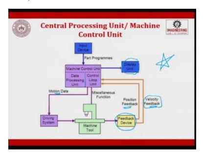
So, when you look at the block diagram for the machine control unit, you have a input device in the machine control unit, you have two parts, one is data processing unit, another one is control unit, control unit is basically for the movement, data processing is to convert the data such that the machine can understand.
