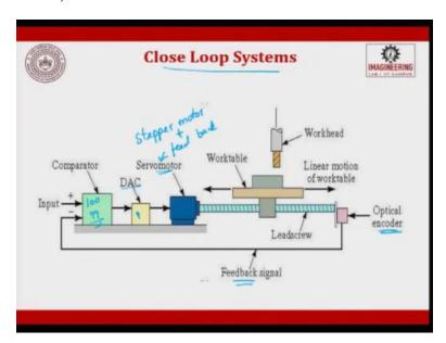
So, when we look at the complete block diagram of a closed loop system, you will see that you have a motor as a servomotor, a stepper motor is converted into a servomotor, it is attached to a lead screw, this lead screw is attached to a table, the table has the work piece, the machining relative motion can happen and at the end of the lead screw, you have an optical encoder which suppose you hear you give 100 turns, it will check whether hundred turns are done.
