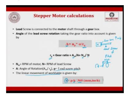
So, the lead screw is connected to the motor shaft so this is the motor, then this is the lead screw. So, the lead screw is connected to the motor shaft through a gearbox, so here I said there is gear box. So, what is a function of a gearbox? The gearbox can increase or decrease, decrease the speed.
