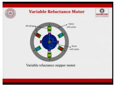
So, the variable reluctant type motor, the variable reluctant type motor, we have a cylindrical rotor is made of a soft steel and 4 poles. It is made of soft steel and 4 poles. It has 4 rotor teeths, 90 degrees apart and six stator poles of 60 degrees apart, these are 90 degrees and these are 60 degrees. So, these, this is a router with pole and these are stator with poles and these are the windings which you have.
