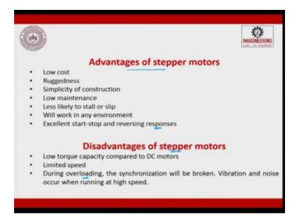
So, what are the advantages of stepper motor? A stepper motor are low cost, they are ruggedness, they are simple in construction, they have low maintenance, less likely to stall or slip will work in
