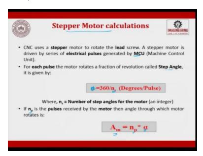
So, stepper motor calculations, we will try to see a small calculation, CNC uses a stepper motor to rotate the lead screw, a stepper motor is driven by a series of electrical pulses generated by MCU, for each pulse the motor rotates a fraction of revolution called a stepping angle. So, stepping angle,
