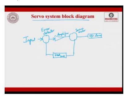
So, let us see the block diagram for a servo system so servo system is input, then you have a error detector, then you will have an amplifier, then you will have a servomotor, then you will have a output device, and from a servomotor we try to give a feedback.
