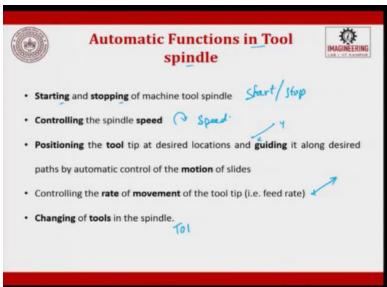
So, welcome to the next lecture on Computer Numerical Control. So, let us look little bit more on functions, so the automatic functions in tools spindle which is there in a CNC machine are, it has
