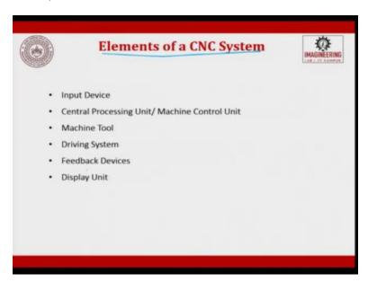
So, let us now look into the elements of a CNC system, you will have a input drive, you will have a central processing unit, or a machine control unit, you will have a machine tool, you will have drive systems, you will have feedback devices, and you will have display units, these are all the elements of a CNC machine.
