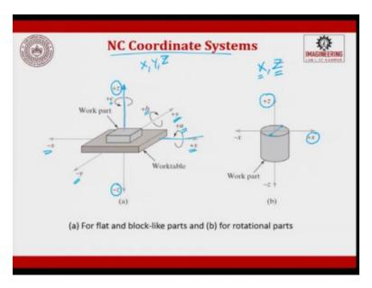
When you take a flat work piece the coordinate system for your flat work piece, when it is resting on your work table, I told you this direction perpendicular to the plane will be Z, when it is away from the work piece it is positive, when it is towards the work piece it is negative right and then once you fix this you will quickly go fix your X axis positive, X axis negative, then Y axis positive, Y axis negative.
