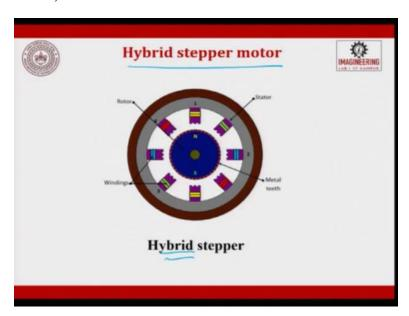
So, this is what it looks like in a Hybrid stepper motor, you will have a mix of permanent and variable reluctance. So, you can see here windings, which are there like permanent and you will have rotor, which has north and south, we will have metal teeths, which gives the combination of both. So, that you try to get the better performance of these two.
