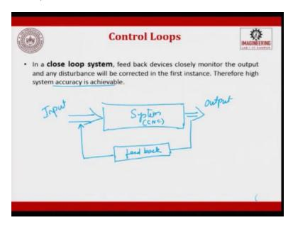
Now, let us look at a close loop system. In a closed loop system the feedback device closely monitors the output and any disturbance will be corrected in the first instant, during the process itself we have a self-correcting mechanism. So, that on process quality assurance is done and not after machining the part, if you look into the block diagram, it will be input, you will have a system, you will have an output.
