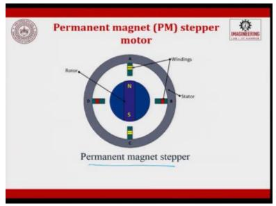
Today the stepper motor technology is very much understood and it has become very competitive. So, you get stepper motors at very low costs today. So, the permanent magnet stepper motor, which was the classification, first classification of the stepper motor, the rotor is a permanent magnet, the permanent magnet motor rotor has no teeth and is designed to be magnetized at right angles to its axis, there is no teeth in the gear.
