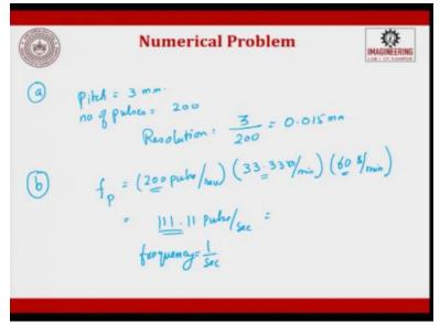
So, let us try to solve a problem so that we have a better understanding about this CNC and in reality you will have these specifications either given by the costumer or by the manufacturer. So, the problem goes like this, the shaft of a stepping motor, or a stepper motor is connected directly to the X axis lead screw of a machine table.
