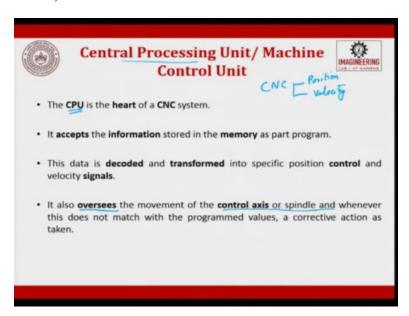
When we talk about the machine control unit or the CPU, CPU is the heart of a CNC machine, it accepts the information stored in the memory as a part program, this data is decoded and transformed into specific position controls and velocity controls. I told you in a CNC machine two data are important, one is position, the other one is velocity, these two are very important.
