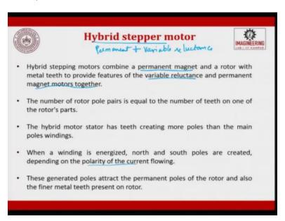
So, you have a Hybrid stepper motor, today which is available hybrid stepper motor is a combination of a permanent magnet and a rotor with a metal teeth to provide features of a variable reluctant and a permanent magnet motor together. So, today hybrid is permanent plus variable reluctance and a permanent magnet. The number of rotor poles paired is equal to the number of teeth on one of the rotor parts.
