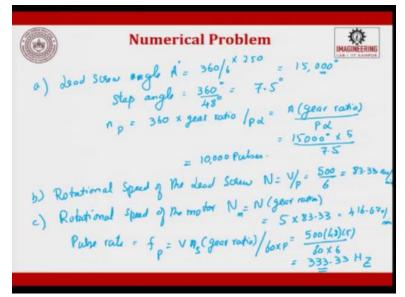
Let us try one more problem, the work table of a positioning system is driven by a lead screw whose pitch is equal to 6, pitch is 6, P is equal to 6 millimeter. The lead screw is connected to a output shaft of a stepping motor through a gearbox, gearbox ratio which is given as 5 is to 1. So, 5 turns of motor to 1 turn of lead screw.
